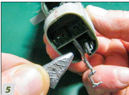
5 The instructions call for 30 grams of weight in the nose, which is about the same as five U.S. quarters. There wasn't enough space to fit that much weight. I flattened a large fishing sinker in a bench vise and glued it in place with superglue. At this point, I kept my fingers crossed and hoped it would be enough. (Spoiler: It wasn't.)
