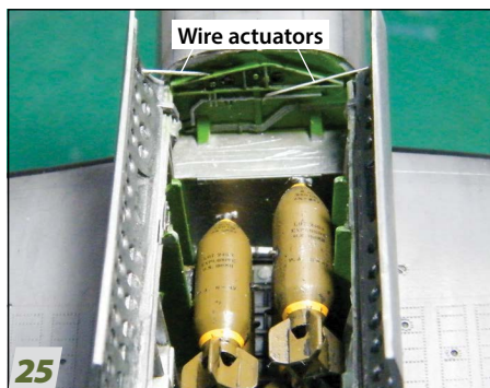
25 I loaded two 500-pound bombs into the bomb bay. Sadly, the kit did not include actuators for the bomb-bay doors, so I made two from .015-inch music wire.
