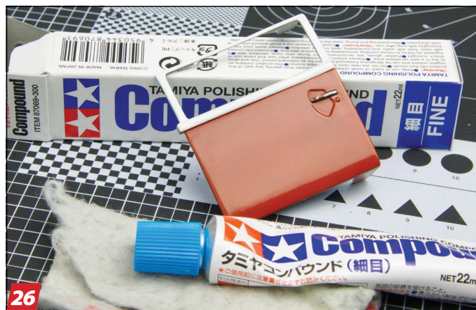
26 With a soft cloth and Tamiya Polishing Compound (No. 87069), I polished all of the body parts. This process creates an extremely smooth surface that resembles the paint on a new or well-maintained car. Just gentle, circular motions is all you need, and take your time. There's no rush. Just polish and relax.
