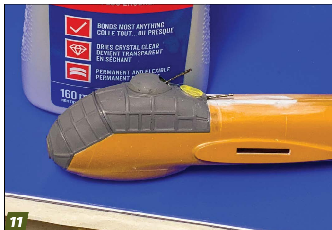
11 Whether it's a modern kit or a vintage one, I turn to white glue, Weld-Bond in this case, to attach clear canopy parts. Hobby-specific canopy glue is another option. These glues allow you to place the part and avoid crazing or fogging the clear plastic.
