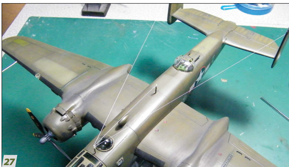
27 For the antenna wiring, I went old-school and stretched sprue. I was able to pull some fine .005-inch strands. Unsurprisingly, they were difficult to cement without melting the material. Thin superglue may have worked better. After the antennas were in place, I brush-painted them with a thinned 1:1 mix of Tamiya Dark Copper (No. XF-28) and Flat Brown (No. XF-10).
