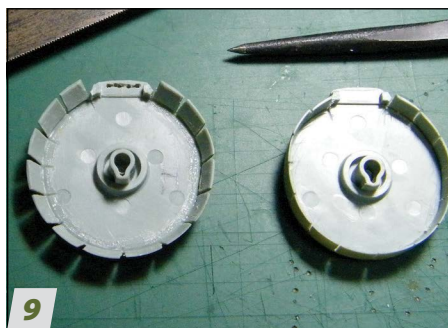
9 The kit cowl flaps come molded closed. That's not too exciting, so I separated the individual flaps with a razor saw. Then I ran a scribing tool around the inside of the cowl at the bottom of the flaps to thin the plastic. But not too much! You don't want them to break. Using tweezers, I tweaked each flap to the correct pitch and touched it with Tamiya Extra Thin Cement to soften and then harden in the new position.
