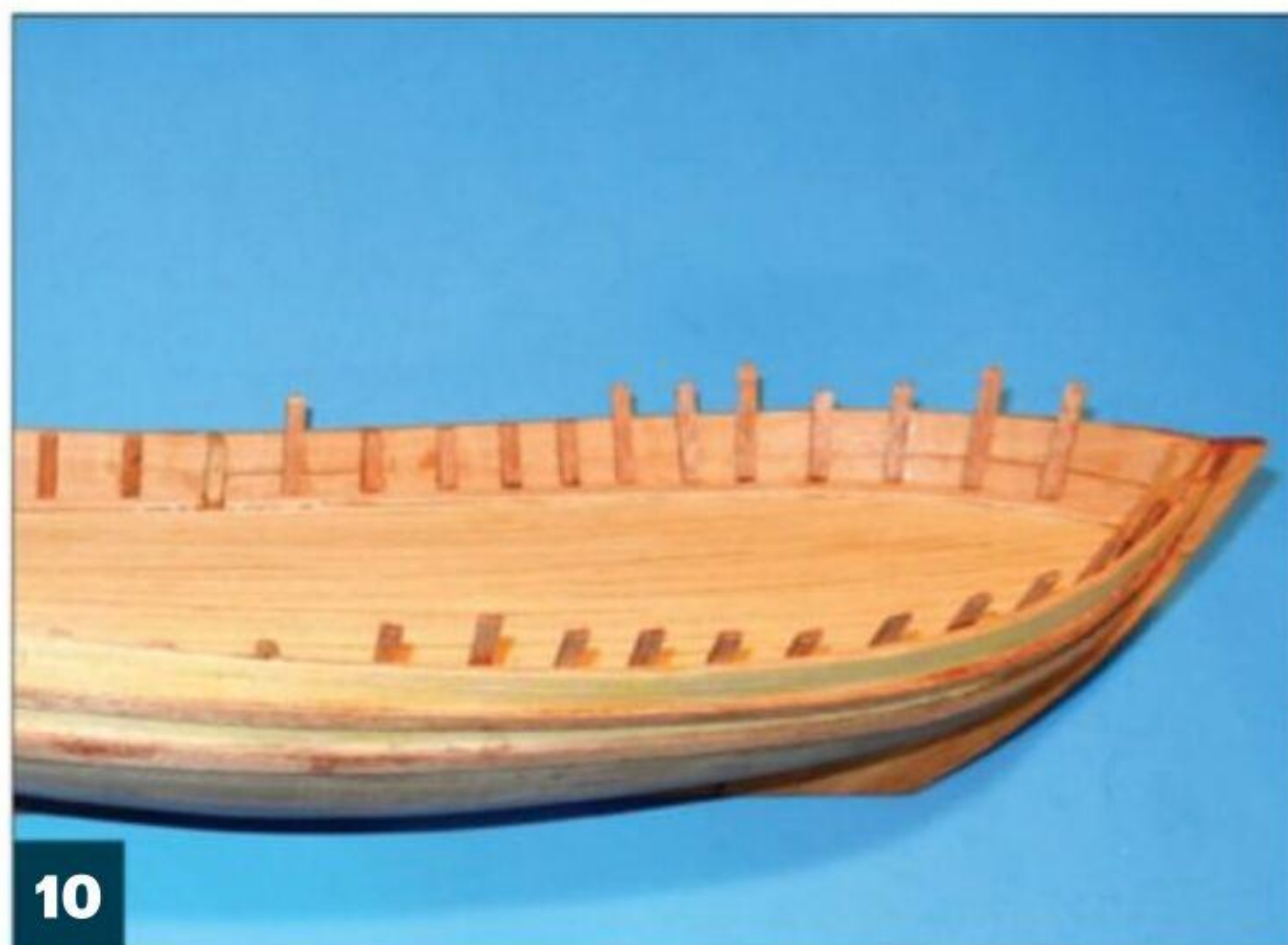
10 Mahogany stanchions were added along the inside of the bulwark. These not only provide more strength to the bulwarks but also reflect what you'd see on a real ship.
