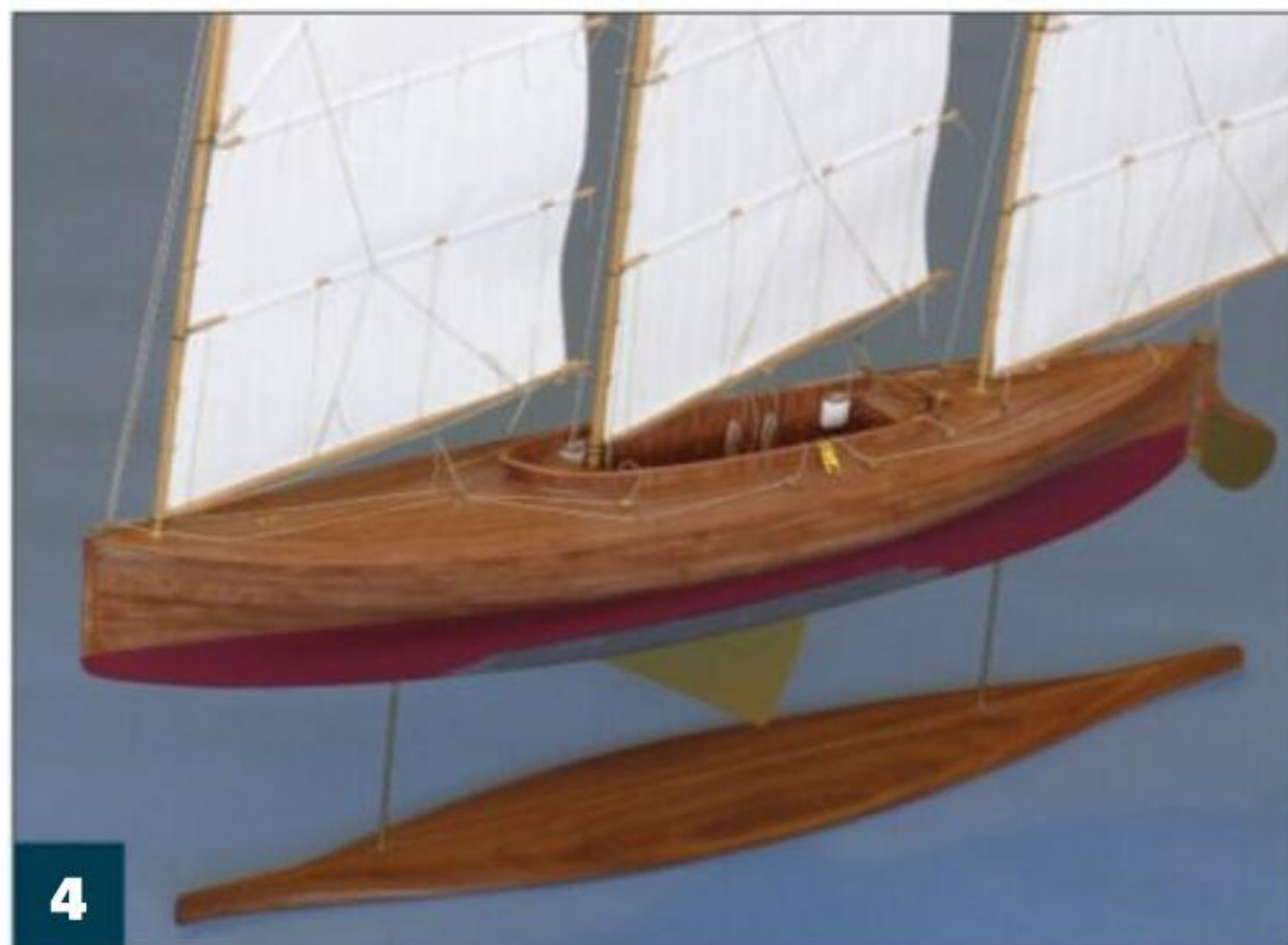
4 Carrying the previous idea a bit further, the base on this model is carved to not only show the shape of the waterline but also mimic the shape of the hull just below it.
