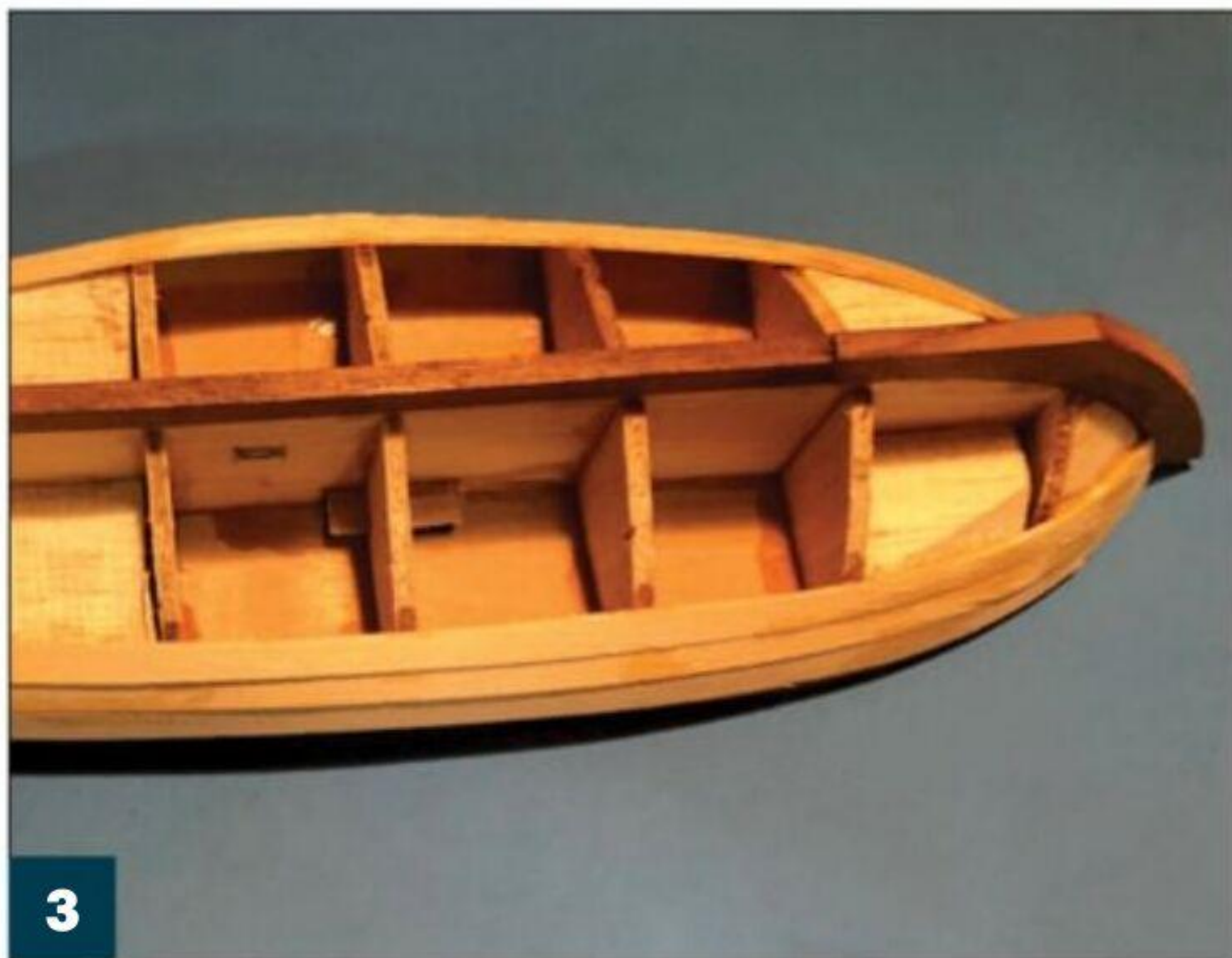
3 I've placed the mahogany keel and begun the first layer of planking. Add planks to both the starboard and port sides at the same time to keep the planks symmetrical and avoid twisting the hull.
