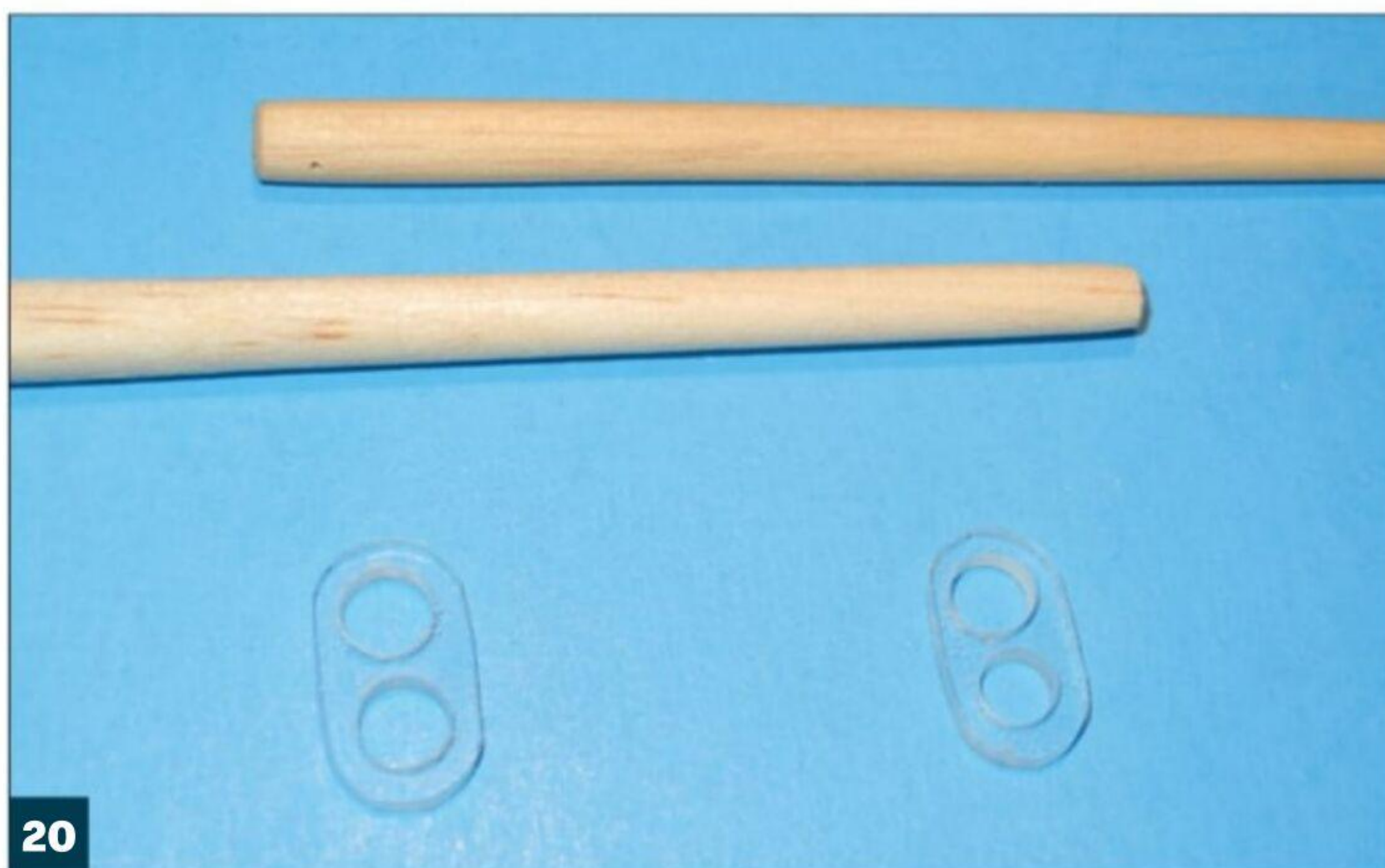
20 The brass fittings for the topmast were brittle with age, so I made new ones from \frac{1}{16} -inch Plexiglas and that I later covered with brass strip.
