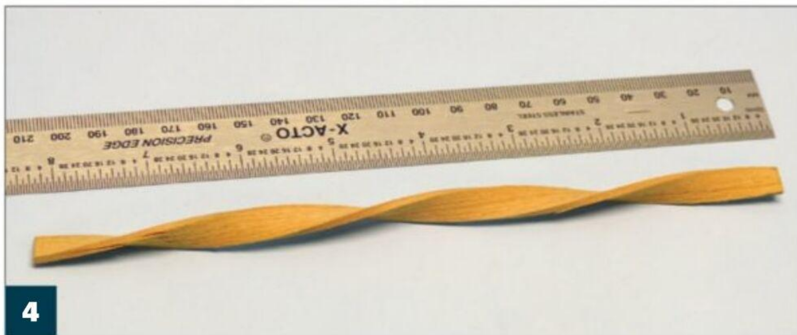
4 I soaked this alder — .080-inch thick, \frac{3}{8} -inch wide, and about 8-inches long — in hot water for a couple of minutes and hand twisted this shape. The ends were clamped and, after the part dried overnight, there was almost no spring back. Alder, related to birch, is one of the best woods for bending, and I use it for most planking.
