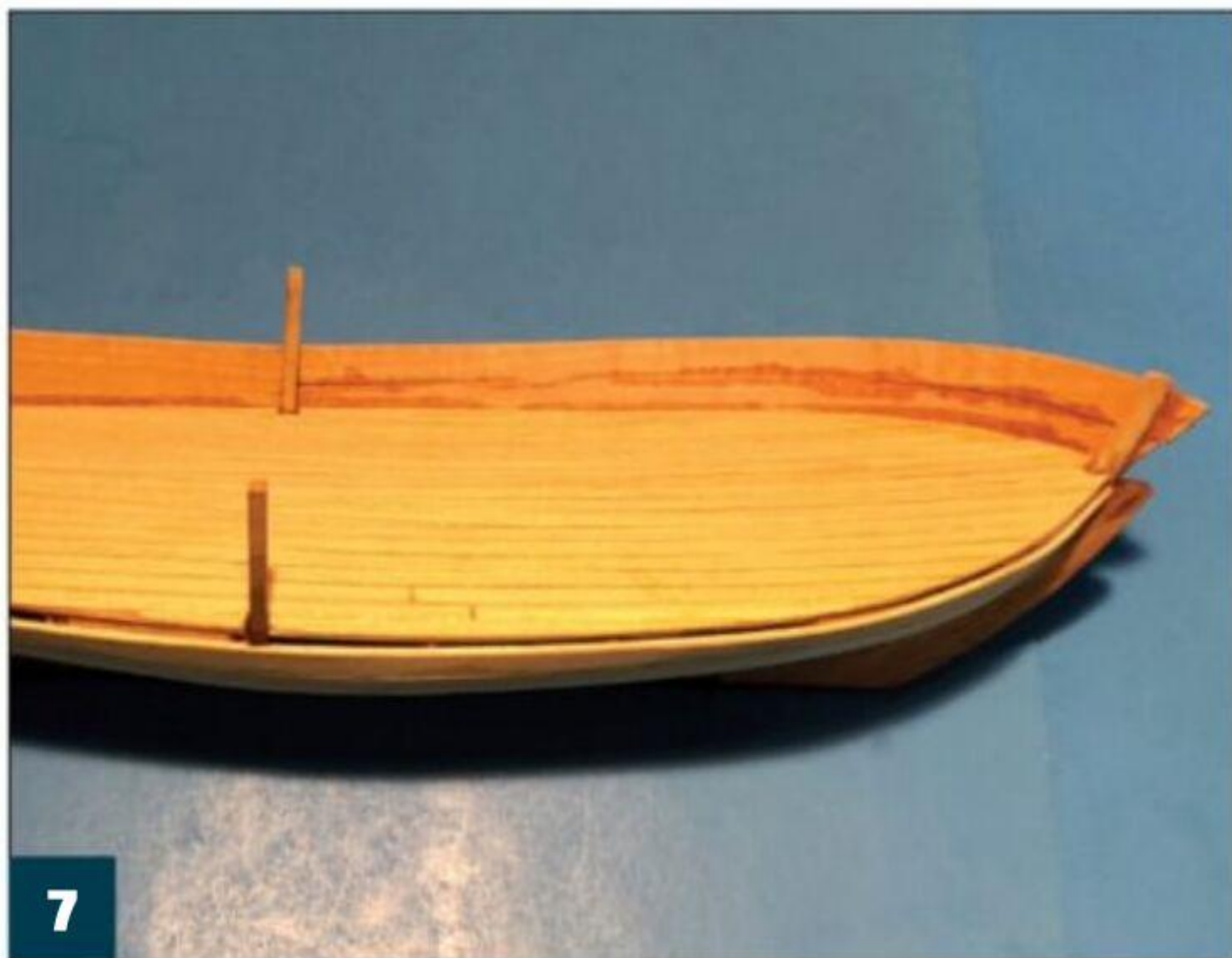
7 The kit provided no stanchions to attach the bulwarks to. So, I made my own from boxwood and then glued the bulwarks in place.
