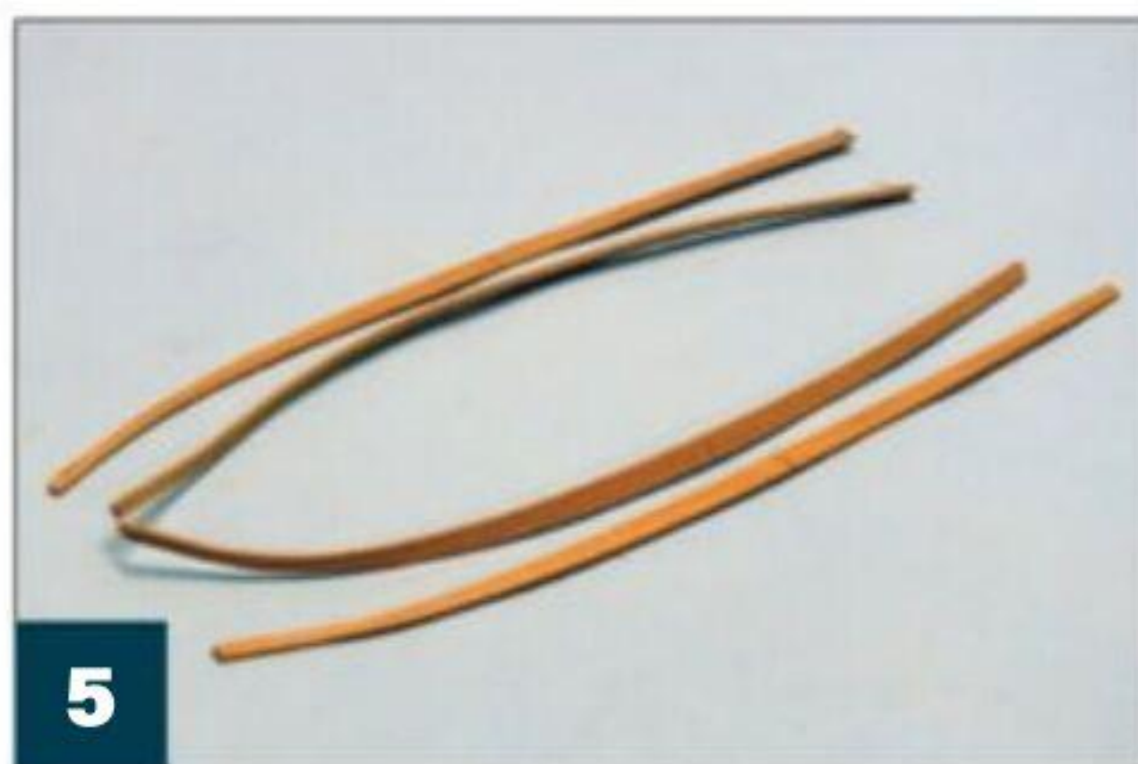
5 Before and after: I cut .050-inch alder for a pair of rowboat garboards (outer pair). After soaking them in hot water for a couple of minutes, I hand-formed them, clamped them to a wood plug carved to the hull's shape, and left them to dry overnight.
