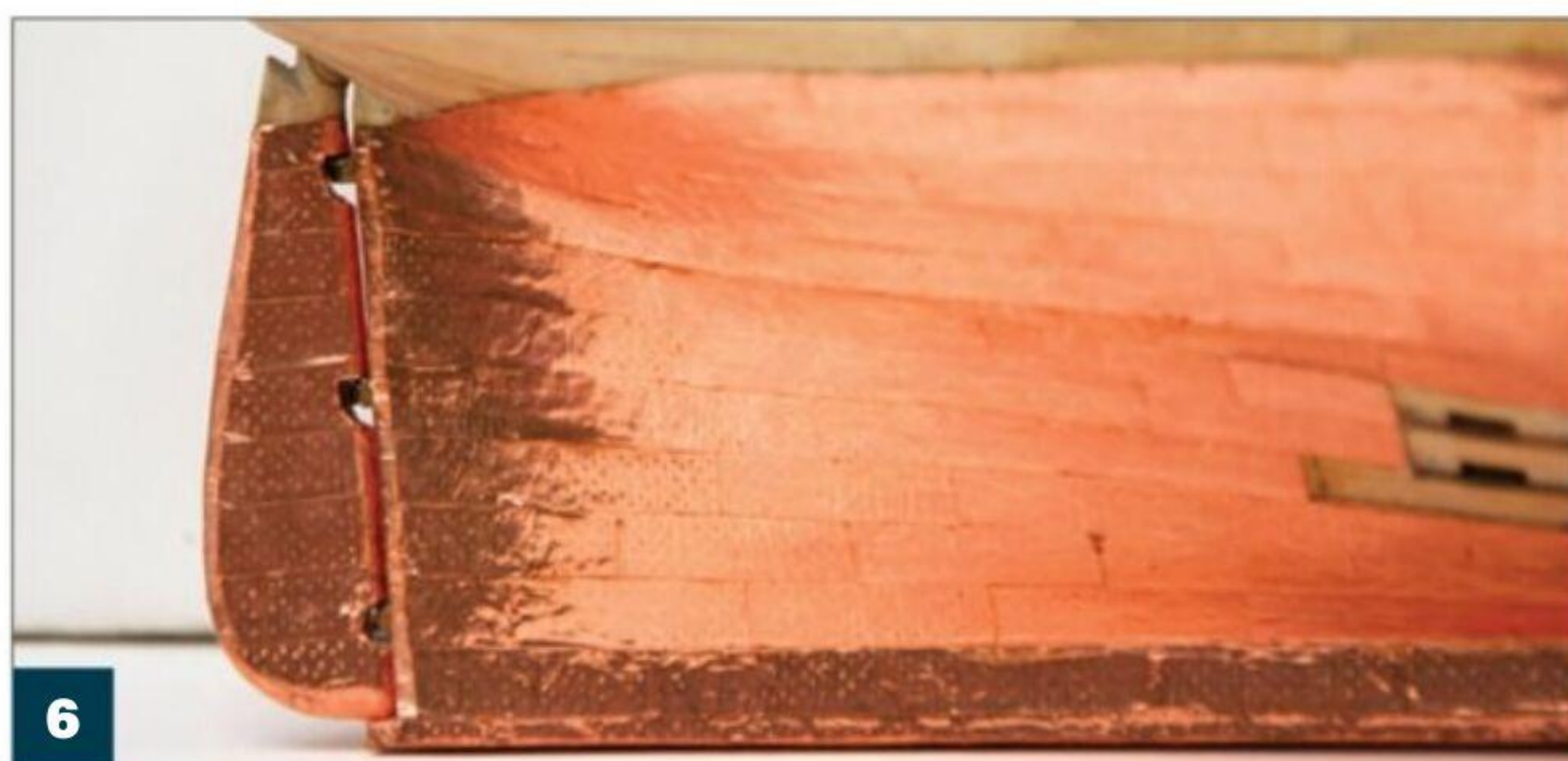
When plating the rudder, use the same rules as the hull: bottom to top, back to front.
