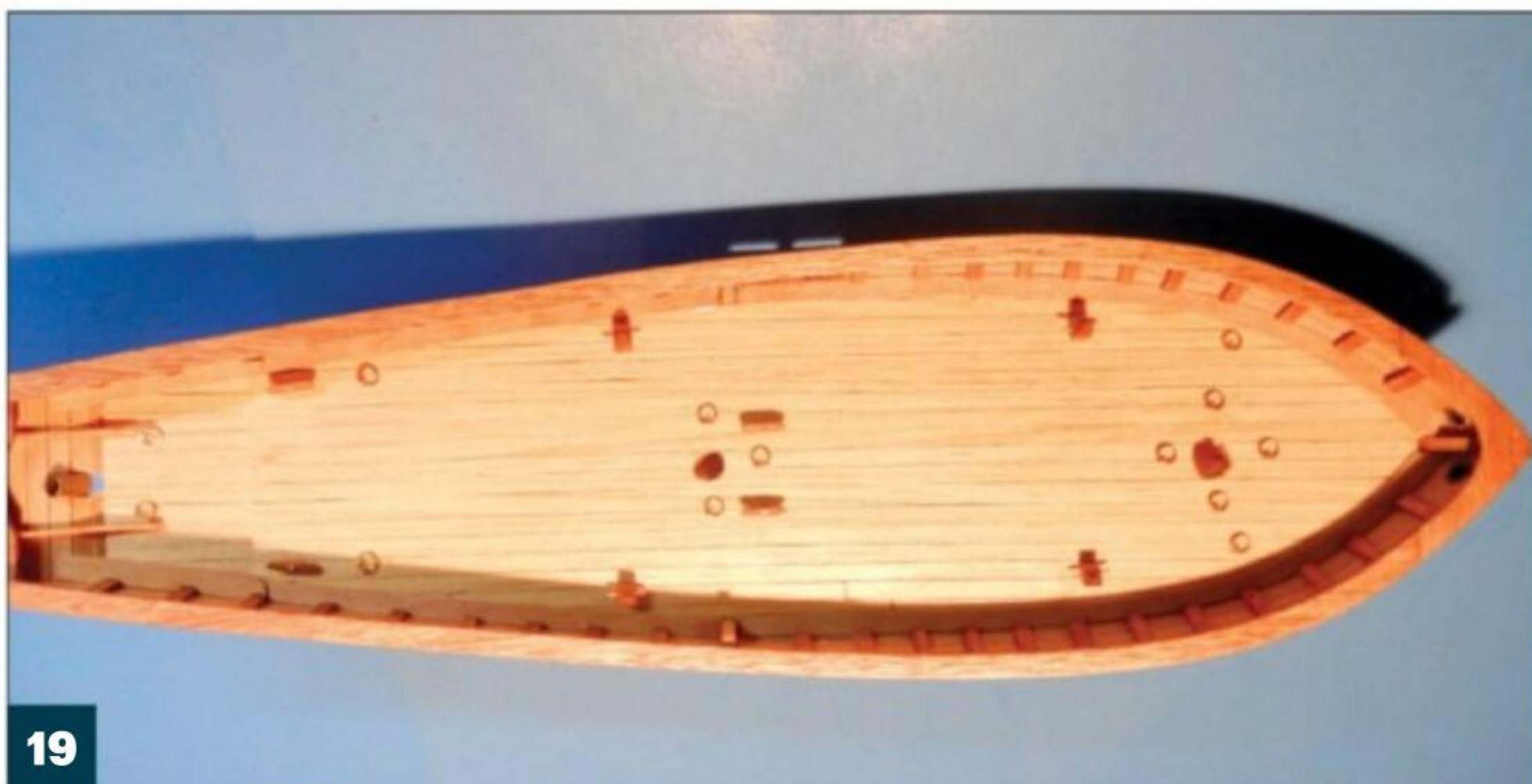
19 Following the kit plans closely, I cut scuppers in the bulwarks at midships and placed all of the minor fittings on the deck, including cleats and eyebolts around the hole for the main mast.
