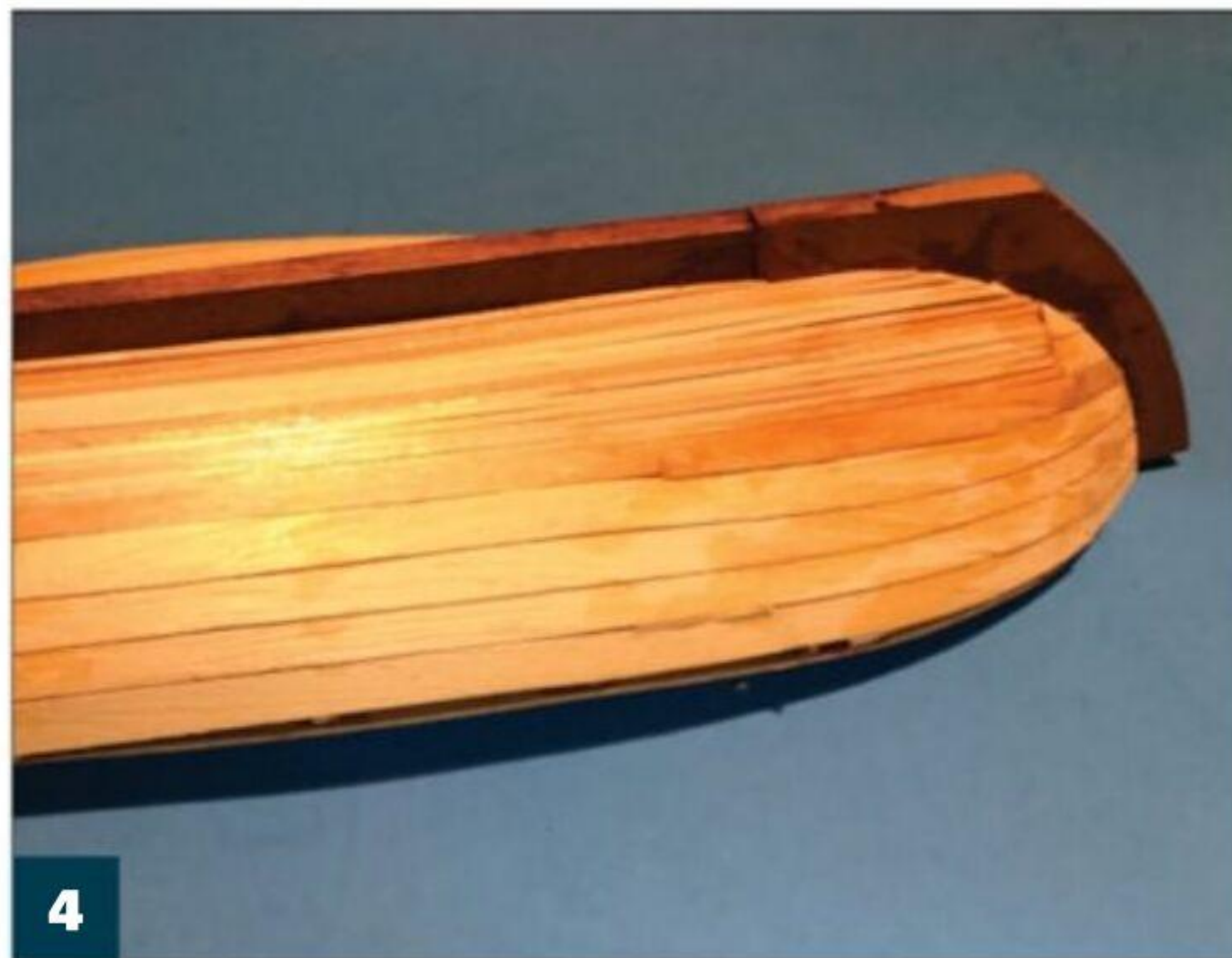
4 The first layer of planks is complete. Note the areas where I turned to narrower basswood strips instead of the lemonwood because the wider planks proved brittle and hard to work with.
