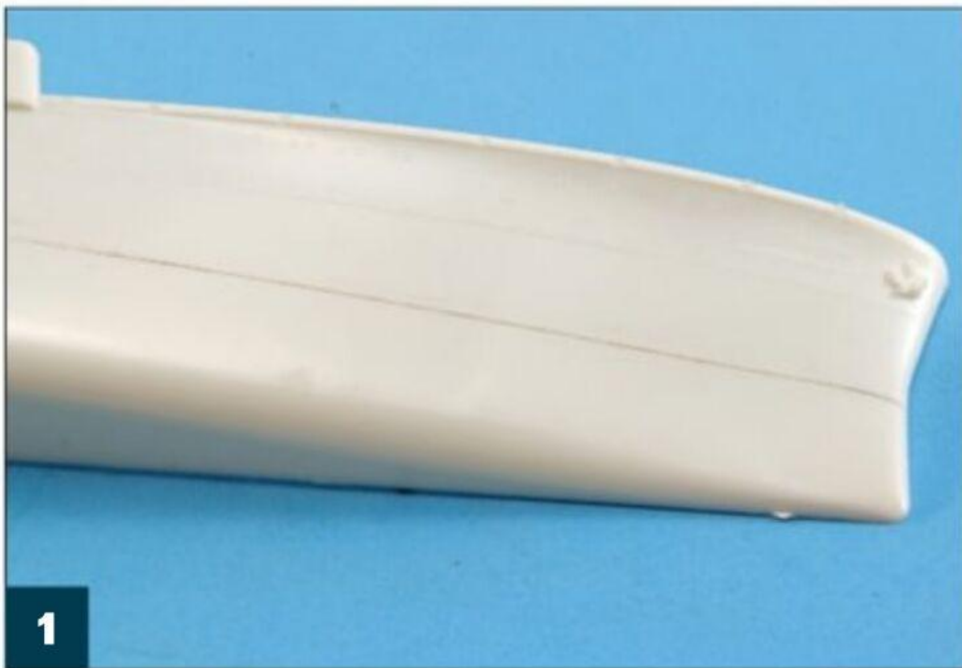
1 Start by marking the waterline along the hull with a pencil or scribing tool. This will help align the tape.
