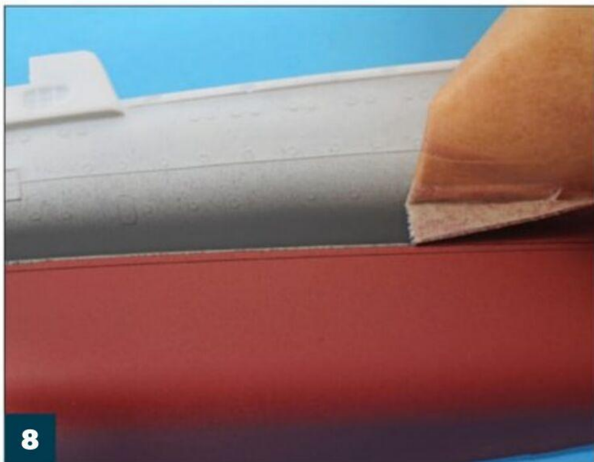
8 Remove the mask from the upper hull. If you do it carefully, it can be reused.
