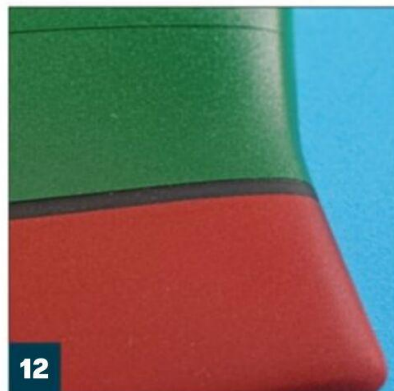
12 Peeling the tape from the waterline reveals a perfectly executed black line with no need for touch up. FSM
