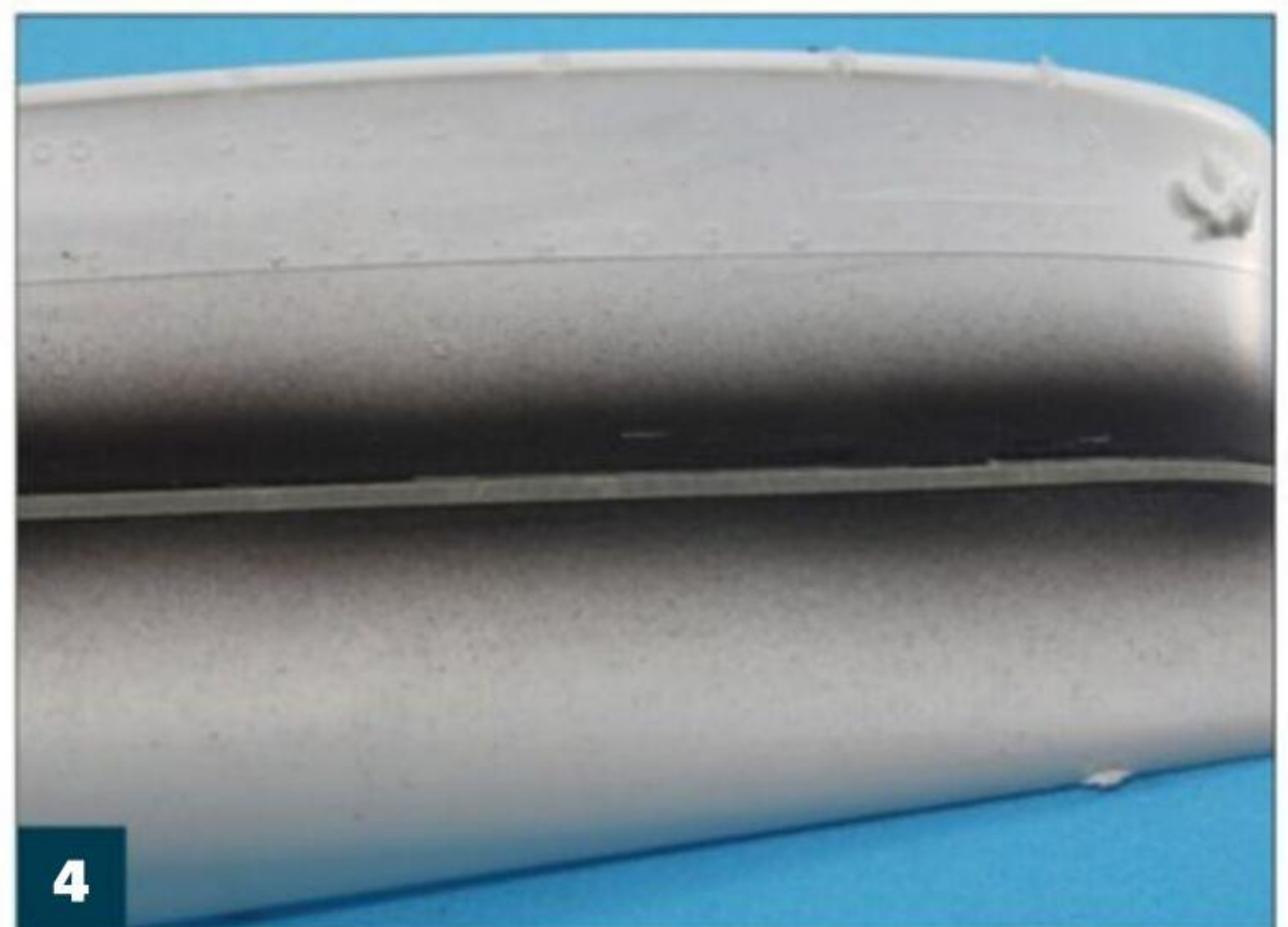
4 Burnish the waterline mask down to the hull for a really tight seal.
