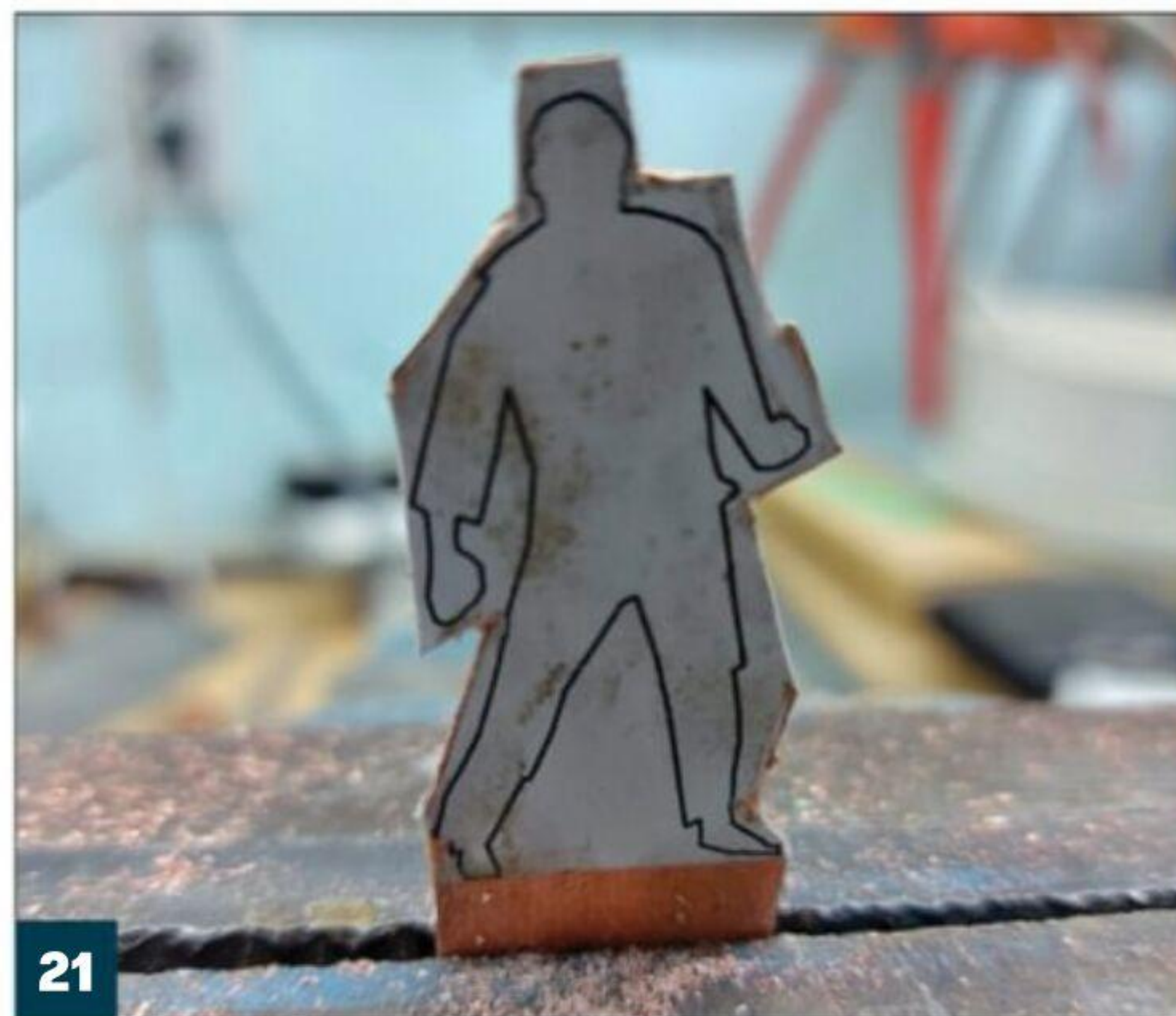
I used tin snips and cutting bits in a rotary tool to roughly shape the copper around the outlines.
