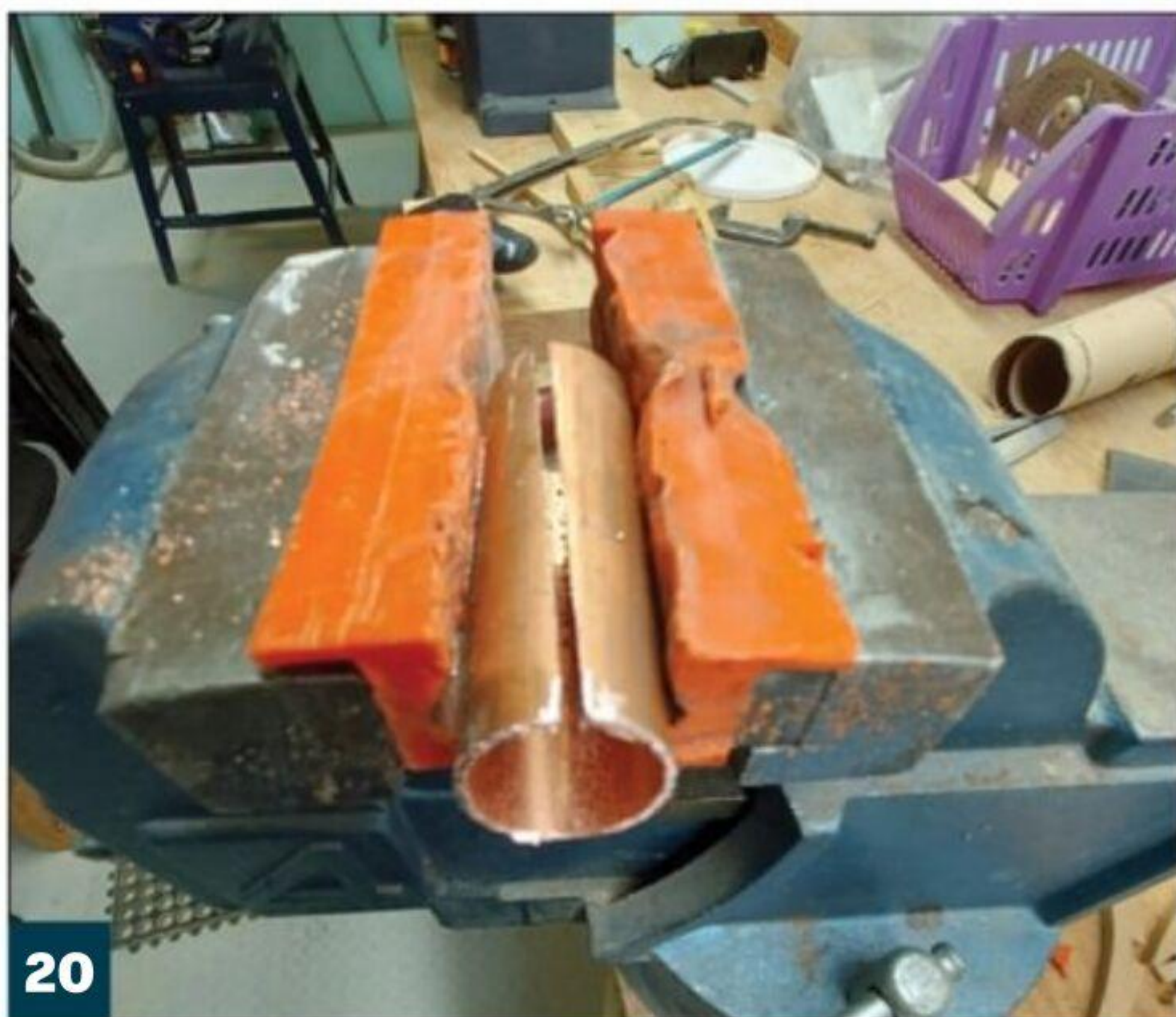
Rather than use cardboard for the silhouettes, I flattened copper tubing. This required more work but gives the figures substance.
