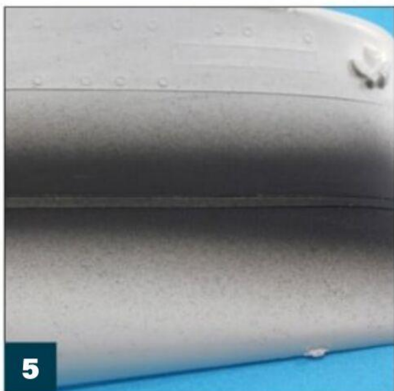
5 Overspray the tape with waterline color to seal the edges. Any bleeding that occurs will match the waterline.
