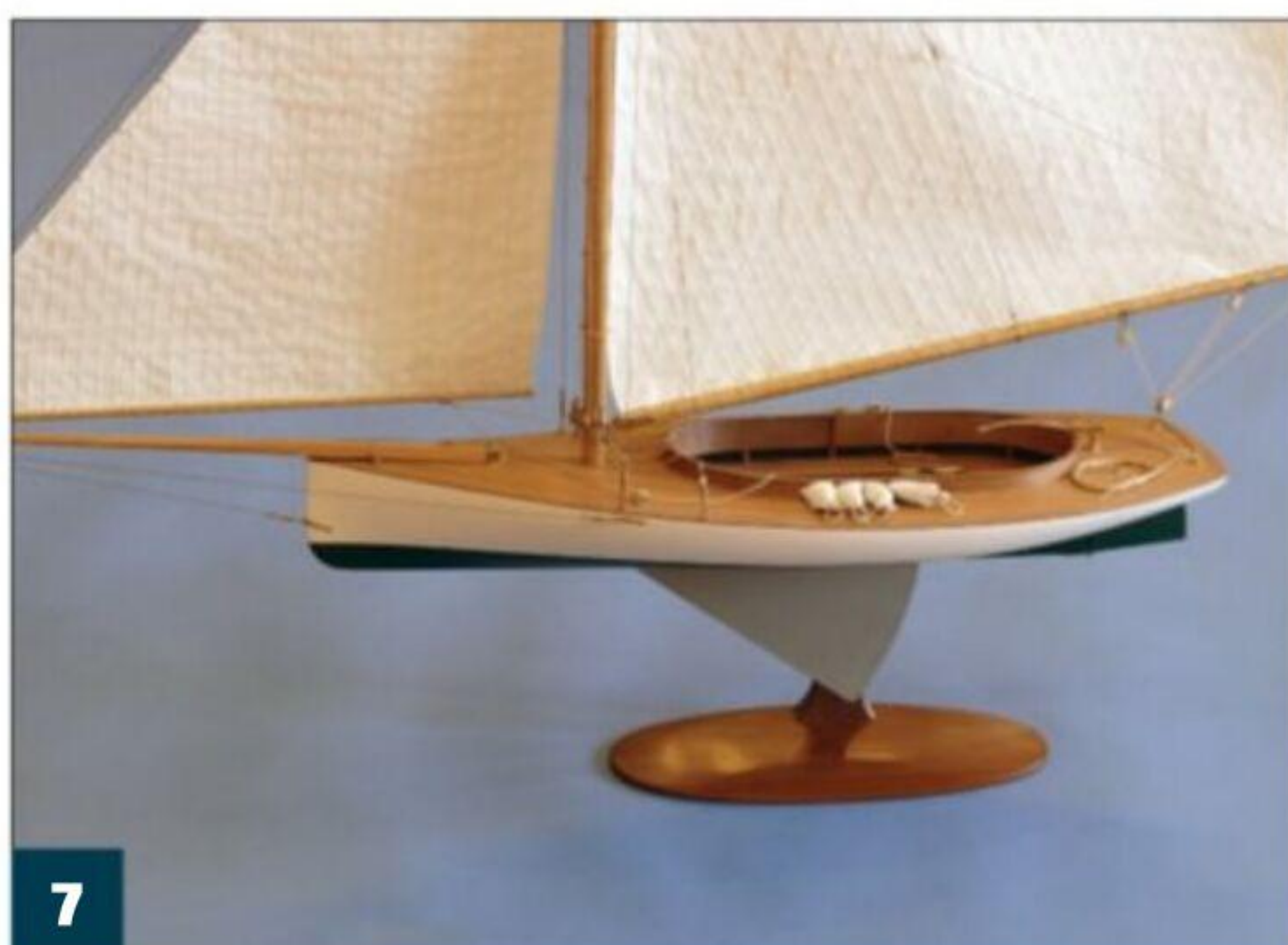
7 A relatively thick wooden base can be made to look thinner if the top surface is given a gradual taper. This concept can be adapted to almost any size or shape.
