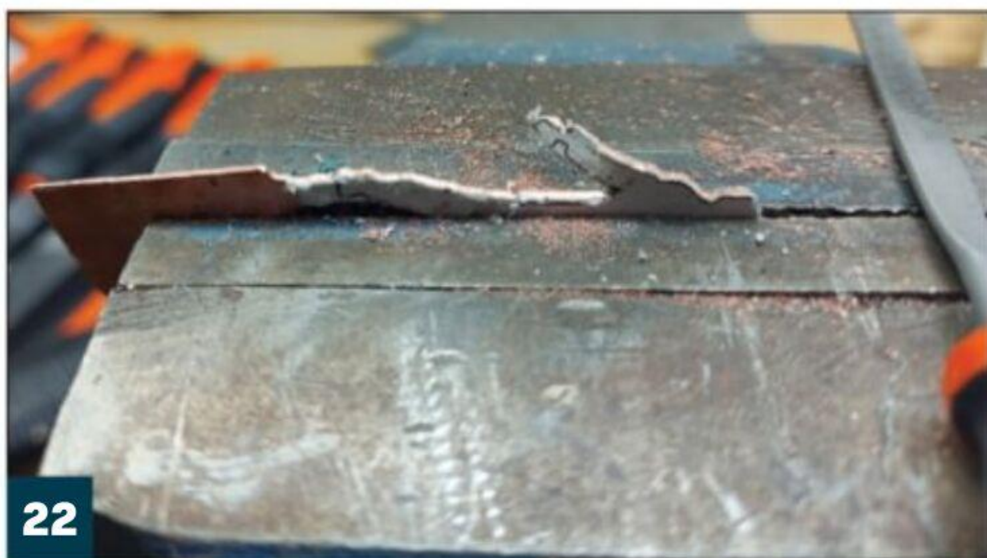
Jeweller's files refined the cuts to form the final shape of the raft's adventurous crew.
