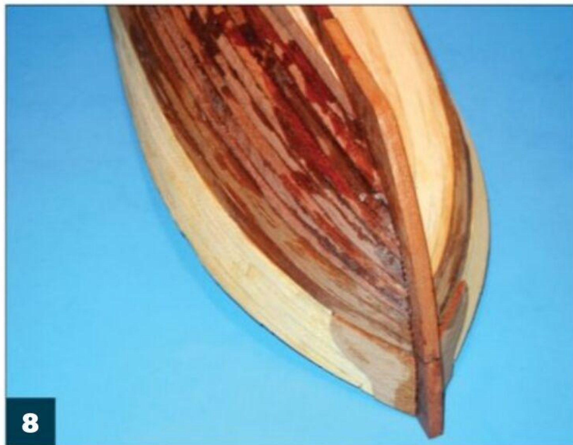
8 The wood supplied in the kit was not ideal, so I turned to strips of black walnut that I milled. You can find lumber of the same dimensions online made specifically for use with model ships.
