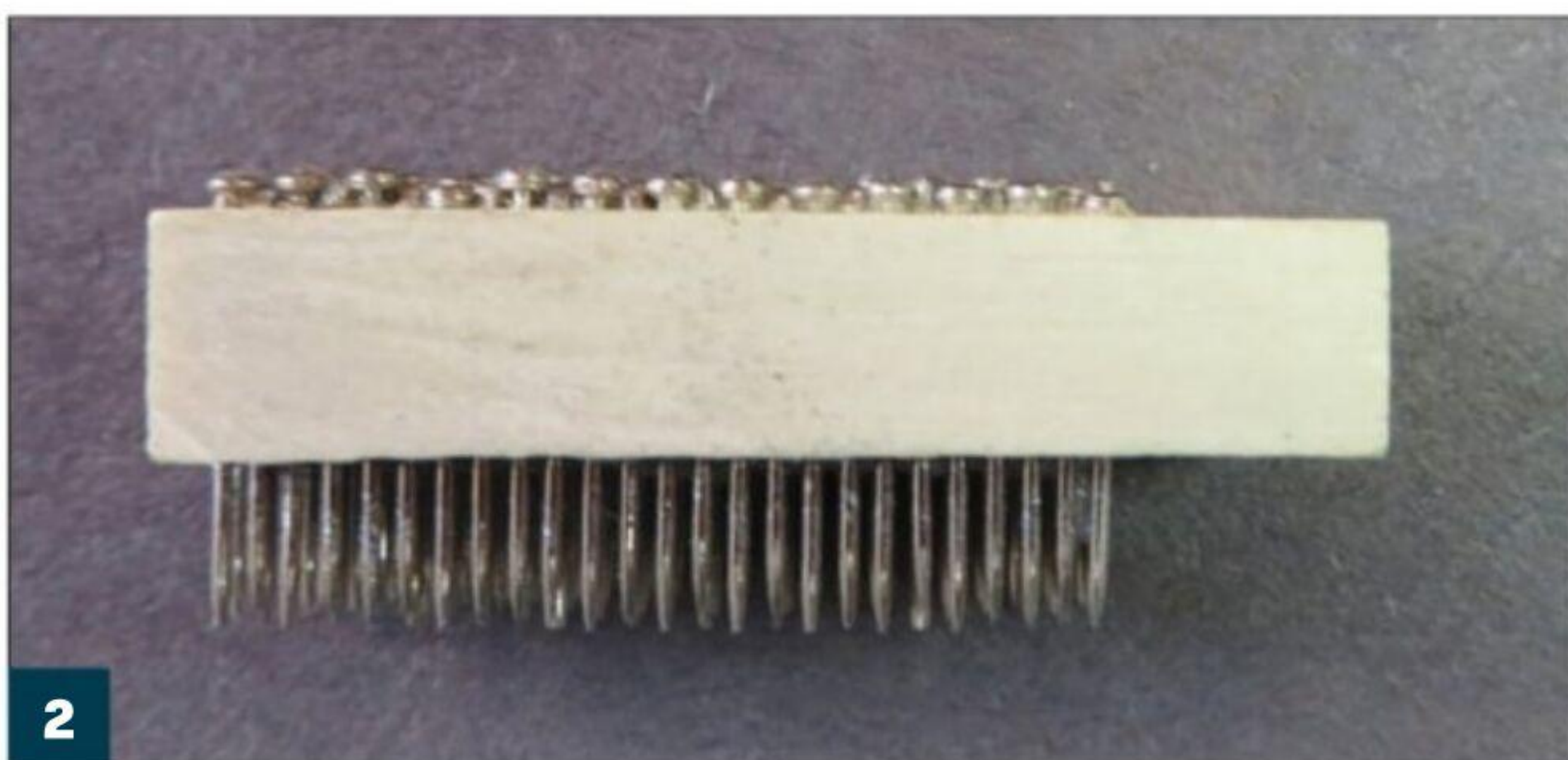
2 Ninety pin locations were bored into the a holly block and filled with applique pins.
