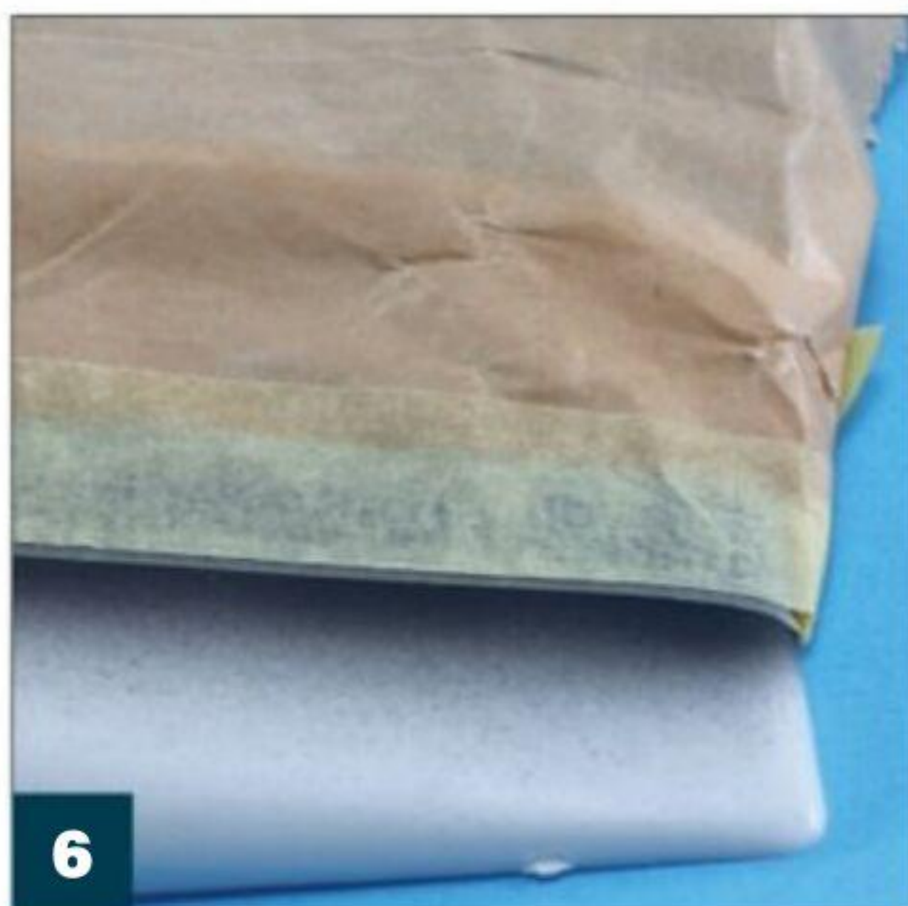
6 Mask the upper hull so the edge of the tape overlaps the waterline tape. I use either ProMask or tape and paper.
