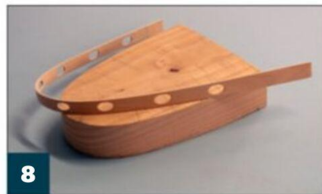
8 Here's the same cabin side, finished. Cutting openings for windows before bending would make it hard to curve the wood evenly around the form. The blank was extra wide to accommodate the hull's sheer and allow the front of the part to stay vertical once it was in place on the model. Details like these require planning.
