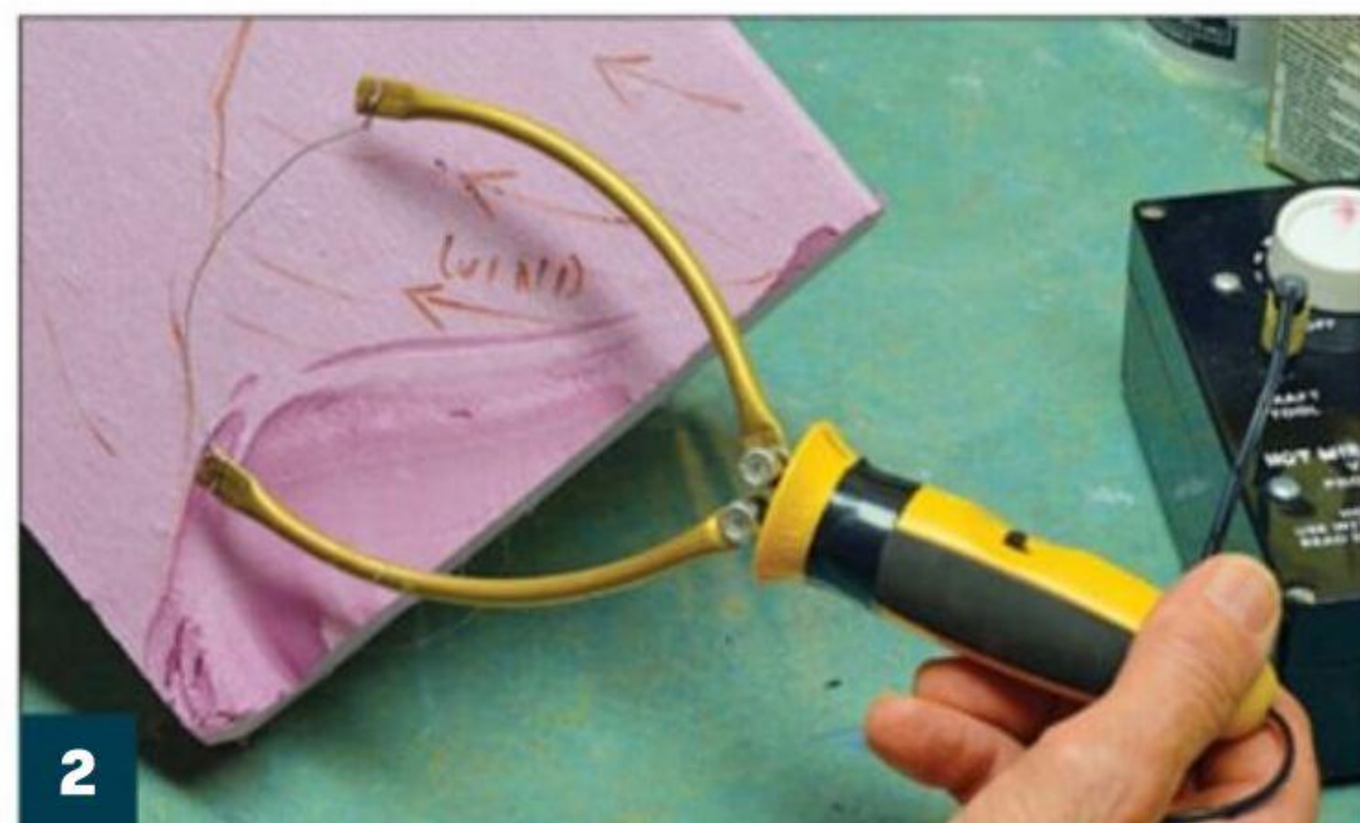
2 A hot wire cutter will give you a good start on where to put the troughs in your water's surface. It is difficult to make a mistake at this stage; follow your crest markings.
