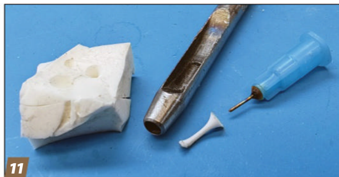
11 To make the Rundblickfernrohr 32 optical sight, I pushed a hollow punch through a piece of silicon rubber to get an elongated shape. Then I pricked the end out with a shortened hypodermic needle to make the eye piece. When painting was finished, I filled this depression with clear gloss to imitate glass.
