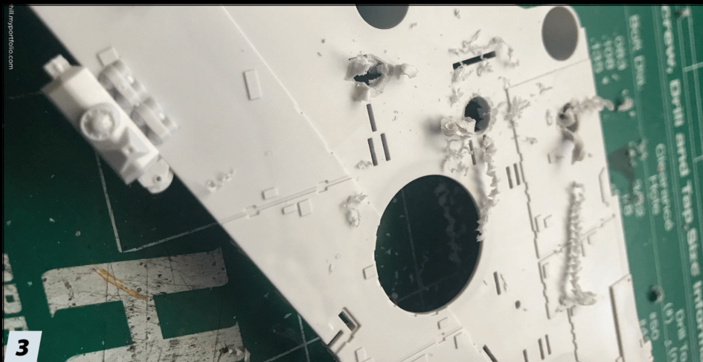
3 Using the blueprint I found on 3DSF.info, I measured and marked where each of the warning lights (.040-inch diameter) and landing lights ( \frac{1}{8} -inch diameter) would be and drilled them. In some cases, I had to remove internal supports to make room for the lights. The lights to either side of the entry ramp are larger, so I drilled them with a \frac{1}{4} -inch bit.
