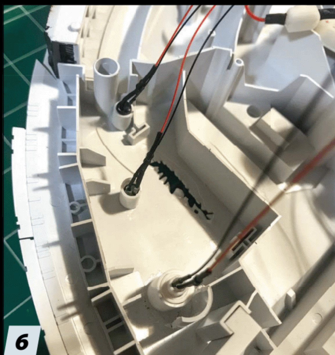
6 I used the same technique for the larger boarding lights, starting with \frac{5}{16} -inch tubing and nesting smaller diameters until reaching the \frac{3}{16} -inch tube and LED.
