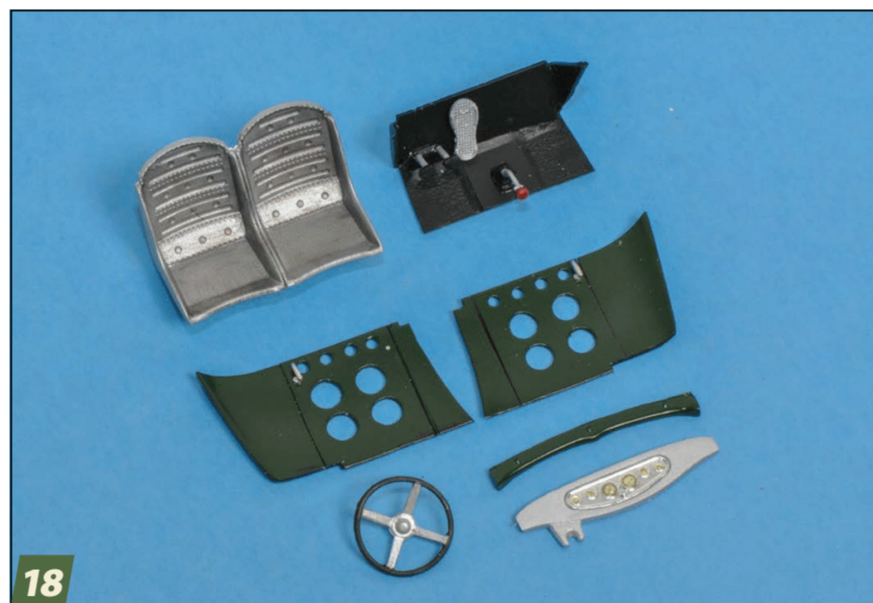
18 The completed interior components: seats from a Revell 1930 Model A five-window hot rod treated with Vallejo Dark Grey Wash (No. 70.517). The new floorboard with a sheet-styrene notch cover sports a shifter and gas pedal from Replicas and Miniatures Co. of Maryland. The steering wheel is from a Mod Rod double kit's '29 Model A roadster.
