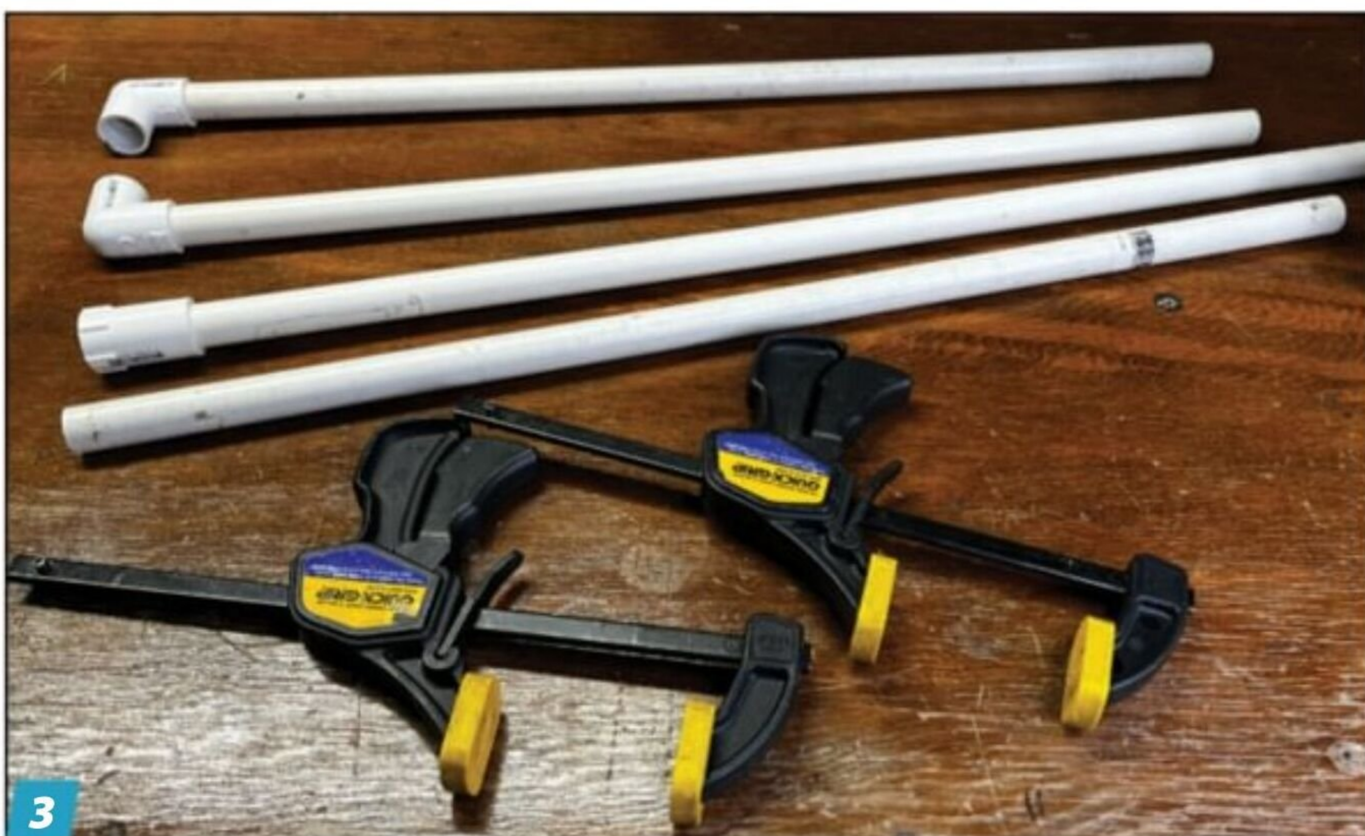
3 A couple of PVC uprights, a stringer to run between them long enough to accommodate your roll of background paper, and two bar clamps to hold the rig upright and you have a portable photo booth perfect for beauty shots — or process shots if you have the room to leave it up.
