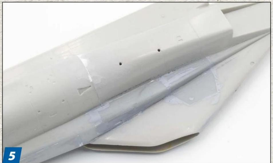
**3** A pair of sprue cutters helped me remove the wing pivot mount on the fuselage. Snipping this off would allow me to fit the wings on the airframe after painting.
