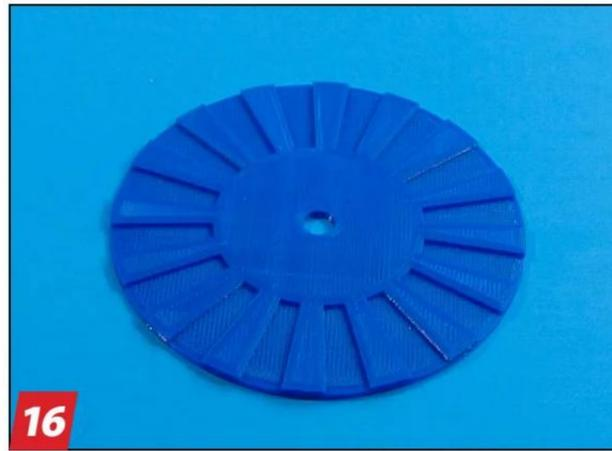
To make the base a bit more appealing, I thought a Japanese Rising Sun emblem would be appropriate. I designed one in a CAD program to fit the can and 3D-printed it.
