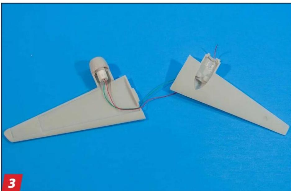
**3** Using a rotary tool, I ground away plastic from inside the nacelles to accommodate the added width of the styrene motor holders. I also drilled a small hole next to the wing attachment point to route the wires from the motors into the airplane body.
