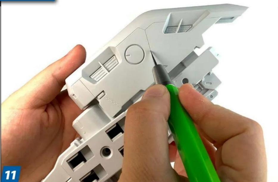
Deepen panel lines on all the parts. Re-scribing panel lines with a scribing tool as shown here creates definition and depth and helps pinwashes flow into the panel lines when applied later on. It has the added benefit of preventing the washes from overflowing and smudging during cleanup.
