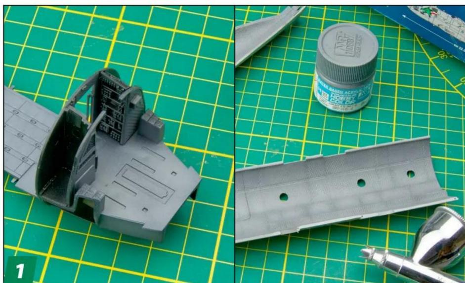
**1** I assembled the interior with Mr. Hobby Mr. Cement S, a quick-drying liquid glue. After priming with Mr. Finishing Surfacer 1500 Black (No. SF288), I airbrushed the floors and walls with a mix of Mr. Hobby FS36118 Gray (No. H305) and FS36231 Gray (No. H317).
