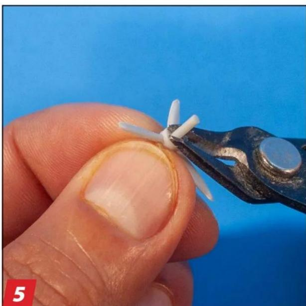
**5** The kit propellers have a shaft that inserts into the face of each cowl. I didn't think I could drill a hole in the shaft precise enough for the motor shaft and provide solid contact to not come apart as soon as I turned the motor on. Instead, I snipped each shaft off flush with the spinner.
