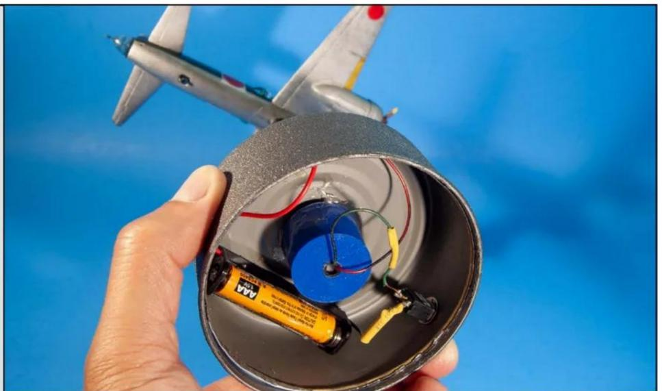
All that was left was to finalize the connections. After some trial and error, I added a 5-ohm resistor in series to the battery to limit the current and slow the propellers to a more realistic speed. Both motors were connected in parallel to the 1.5V AAA battery, and the power switch completes the circuit. All the components fit in the space under the can with room to spare.
