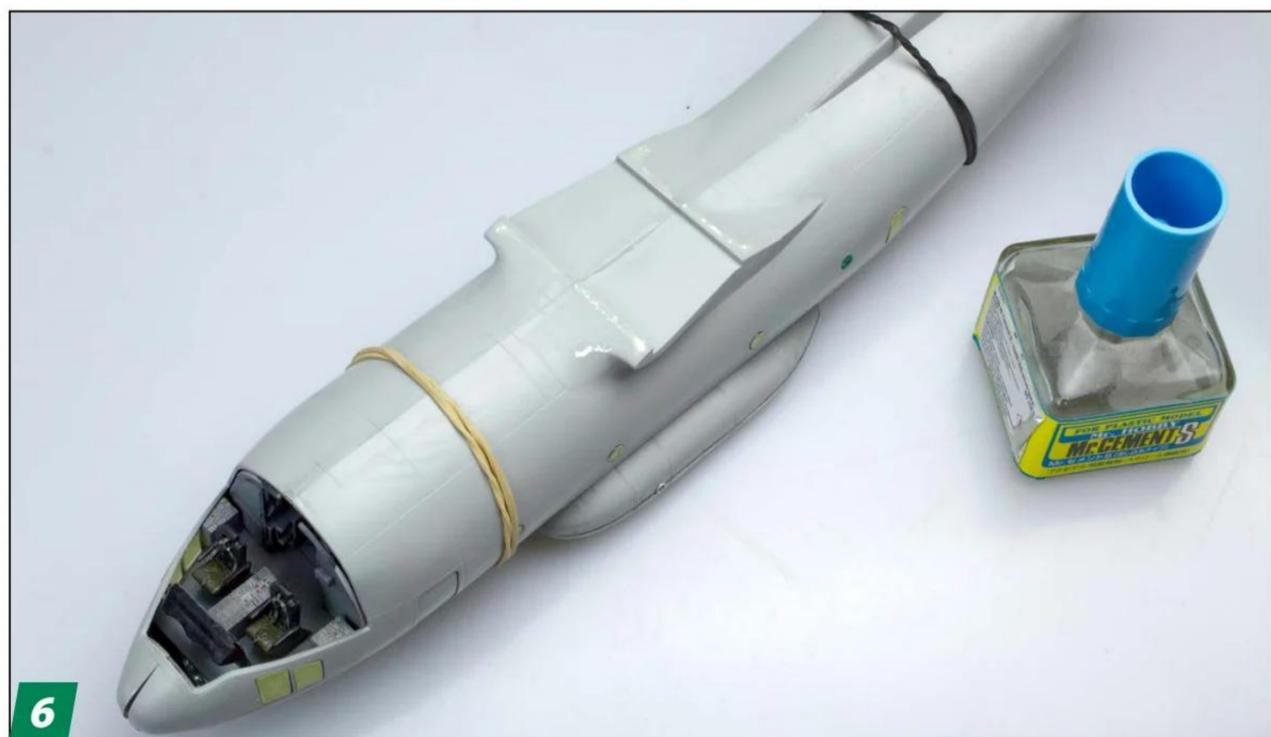
**6** I clamped the large fuselage halves with rubber bands to ensure they stayed together as the glue set. I used Mr. Hobby Mr. Cement S, which penetrates deep into the joins and provides a strong bond. After sanding the seam, I applied Mr. Dissolved Putty (No. P119) and sanded it smooth; this can take several applications.
