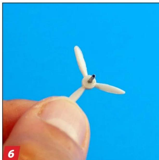
**6** Next, I drilled a hole into the back of the spinners and glued in lengths of copper tube that fit perfectly over the motor shaft and ensured a good connection.
