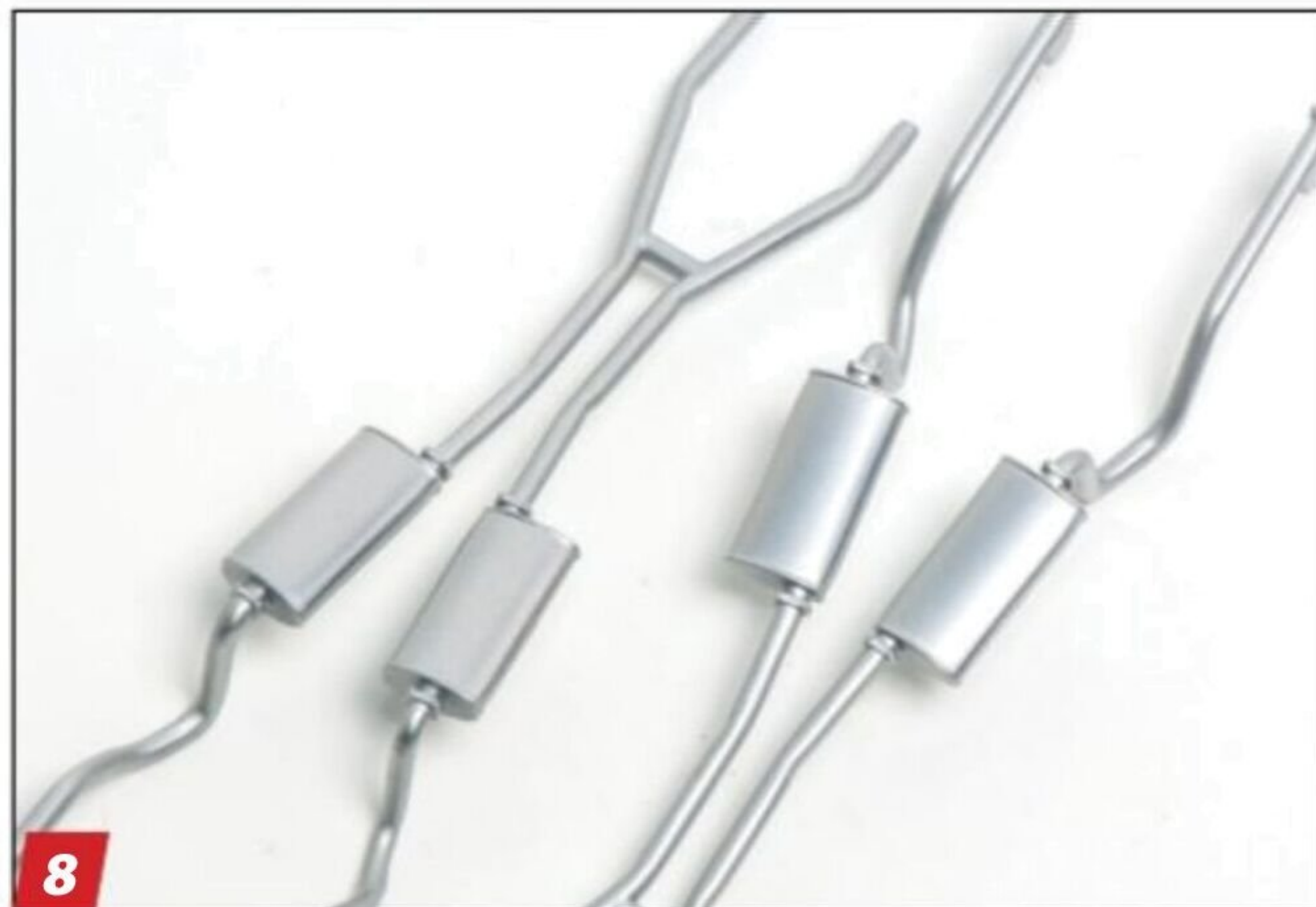
8 Exhaust systems can be finished with metallic grays or silvers. Some builders add a light overspray of rust-colored primer. Mufflers should be painted a slightly different shade, or you can add Matte Aluminum Bare-Metal Foil (No. 011) to them as seen on the right.
