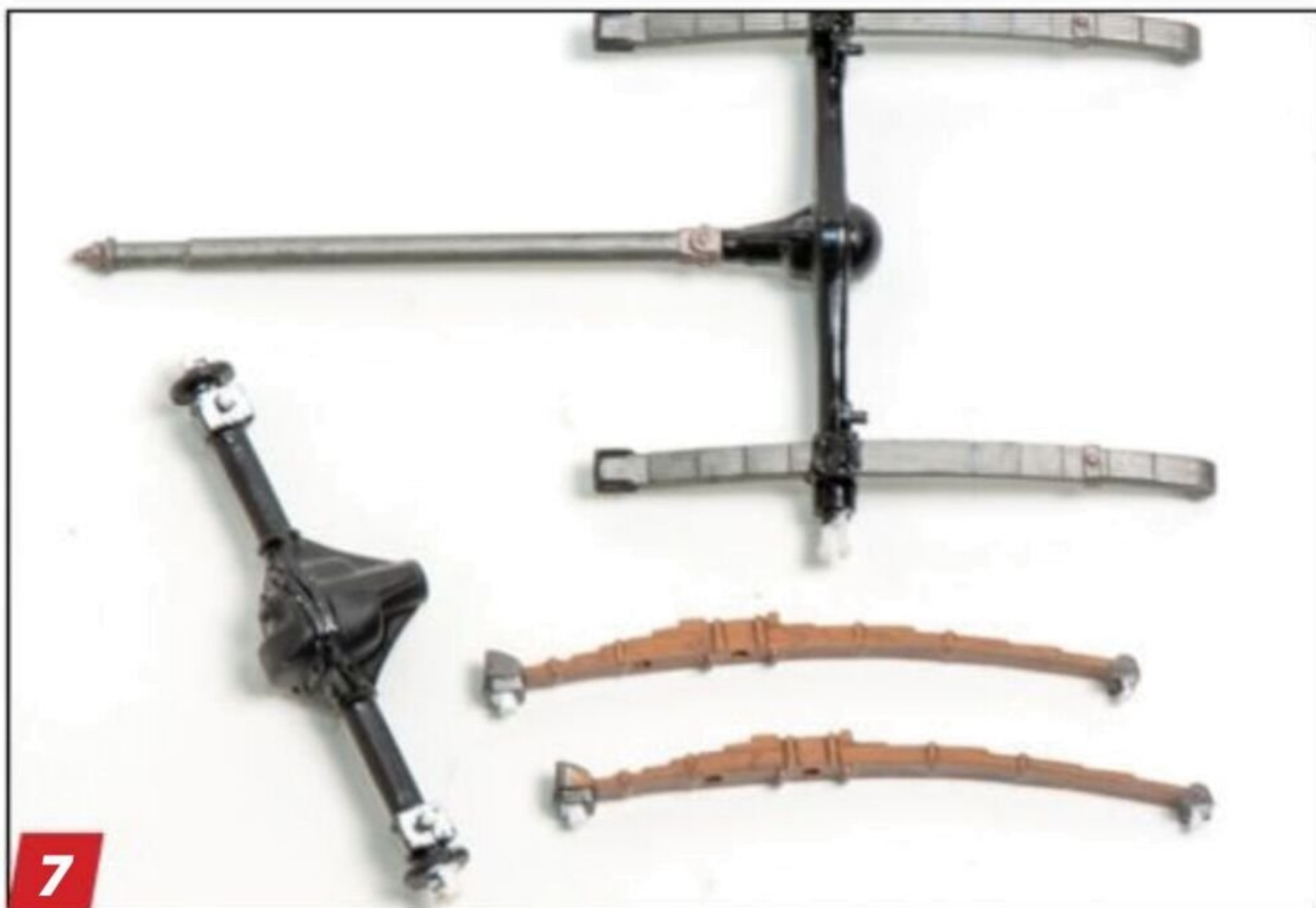
7 Chrysler's mid-century cars used leaf springs and solid rear axles. Restorers debate whether leaf springs should show metallic gray, Cosmoline coating, or black. Axles were usually gloss or semigloss black, and differentials were either black or metallic gray.
