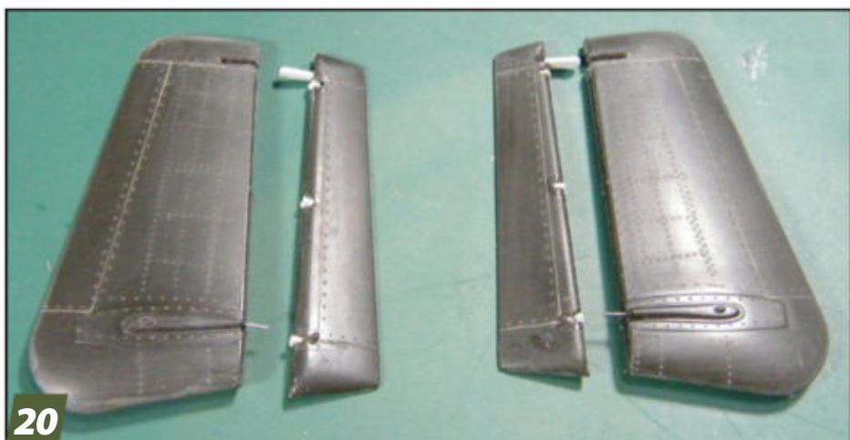
20 I cut the rudder halves from the fins before assembly. The mass balance at the top of the rudders was made from .030-inch styrene and corresponds to a slot cut into the fin's trailing edge. The rudder hinges are .030-inch square strip, and the push rod is .015-inch wire.
