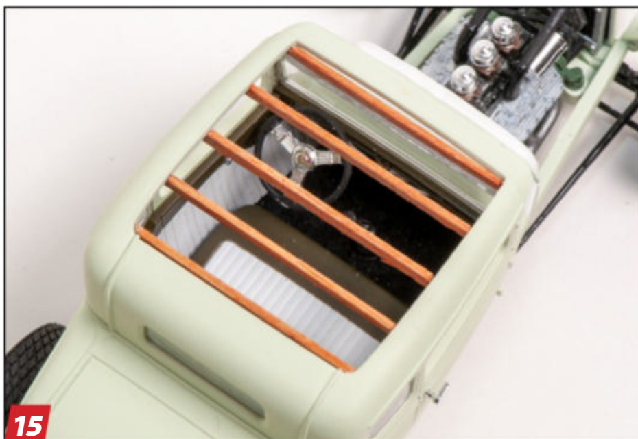
15 Some full-scale hot rods have exposed wooden roof bows. This process involves removing the molded flange in the Revell kit's roof and cutting thin braces from wood. Stain the braces before installation and attach with 5-minute epoxy. Visit FineScale.com/How-To for a Snapshot tutorial!
