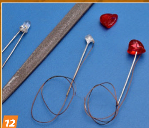
I hollowed out the solid gumballs with a spherical bit in a rotary tool and shaped LEDs to fit taking care to avoid working parts. The negative lead of each LED — they all go to a common ground — was retained to double as a support, but I cut the positive nearly flush with the underside of the LED and soldered on fine wire. The LEDs were inserted into the gumballs and the spaces filled with transparent epoxy resin.
