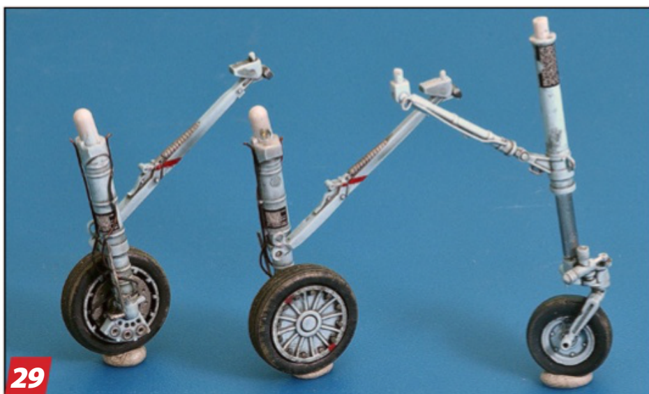
After painting the landing gear legs and wheels with Humbrol Sea Blue, I detailed them with copper-wire brake lines. I replaced the extended oleo on the nose leg with .8mm steel rod.
