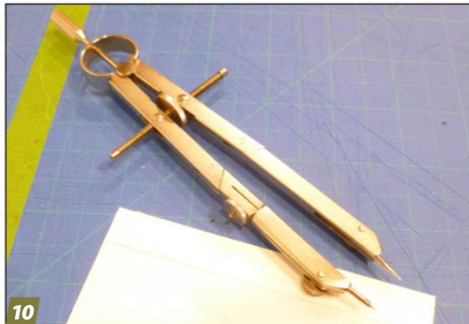
10 The thin line produced by dividers is barely visible, but this piece will be cut into ammunition rack faces and backs. I used a hobby knife to finish the cut; on thin styrene, repeat the passes with the dividers would have been enough to cut through.
