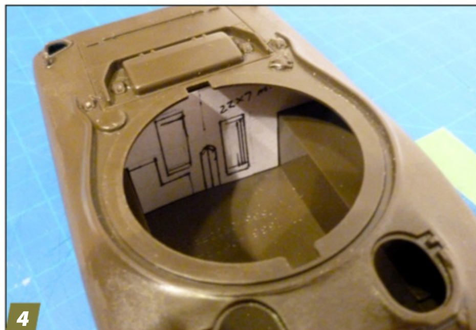
4 To ensure the engine compartment bulkhead's pattern was correct, I installed it with the upper and lower hull in position; tape held the pattern in place.
