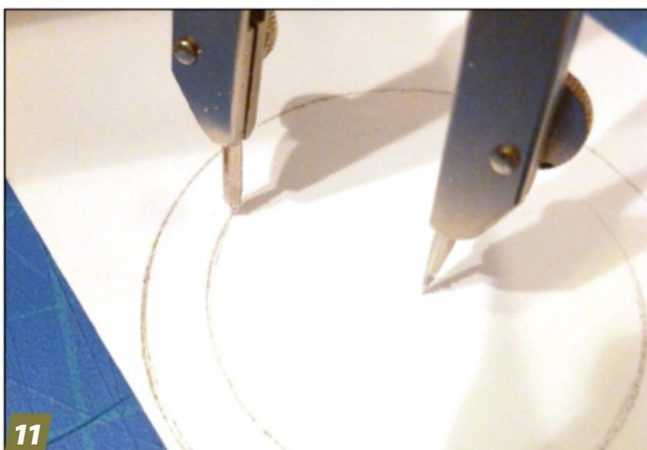
11 This is the easiest way I've found to make larger circles in styrene is to use dividers with two points. Here are the turret floor and step, which extends the entire turret floor over the sponson area. This technique works great for any larger circle.
