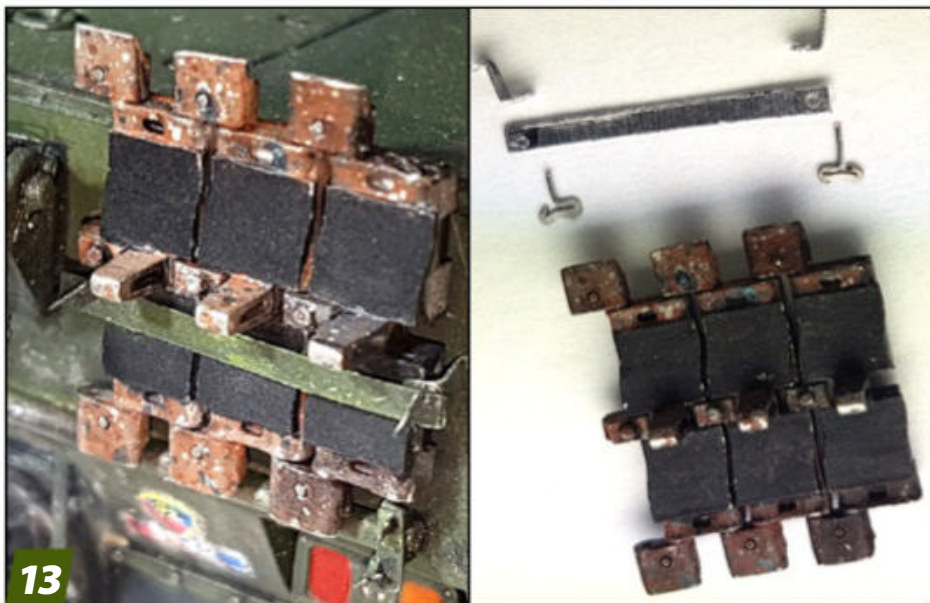
I wasn't happy with the spare tracks provided for the rear plate, so I mounted three extra Friulmodel links in a scratchbuilt rack.
