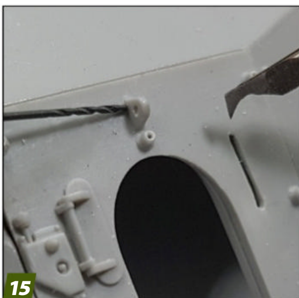
Improvements on the turret's front: I opened a lifting hook with a fine drill bit, hollowed mounting bosses with a needle, and deepened the gunner's sight slit with an engraver.
