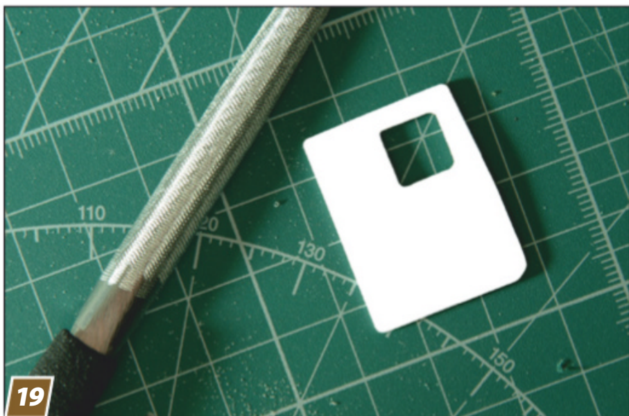
19 With the window opened by a drill bit and hobby knife, final shaping was accomplished with a small file.
