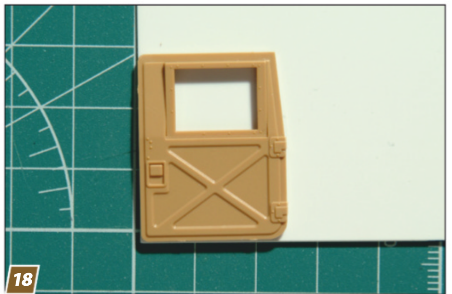
18 Using the kit doors as templates, I traced each door's outline onto .030-inch sheet styrene to form the armor doors.
