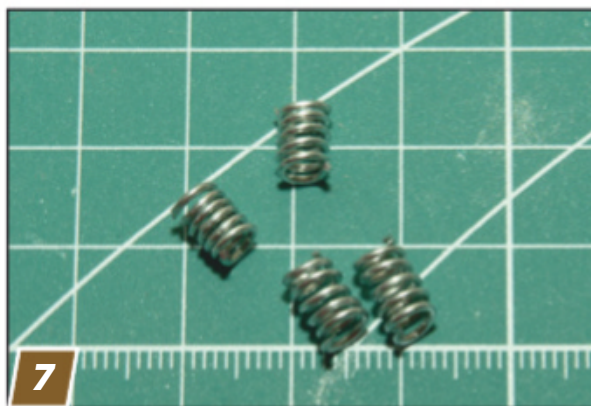
Paper clips, straightened then wound around a mandrel, produced scale springs that were easily compressed to fit their space.
