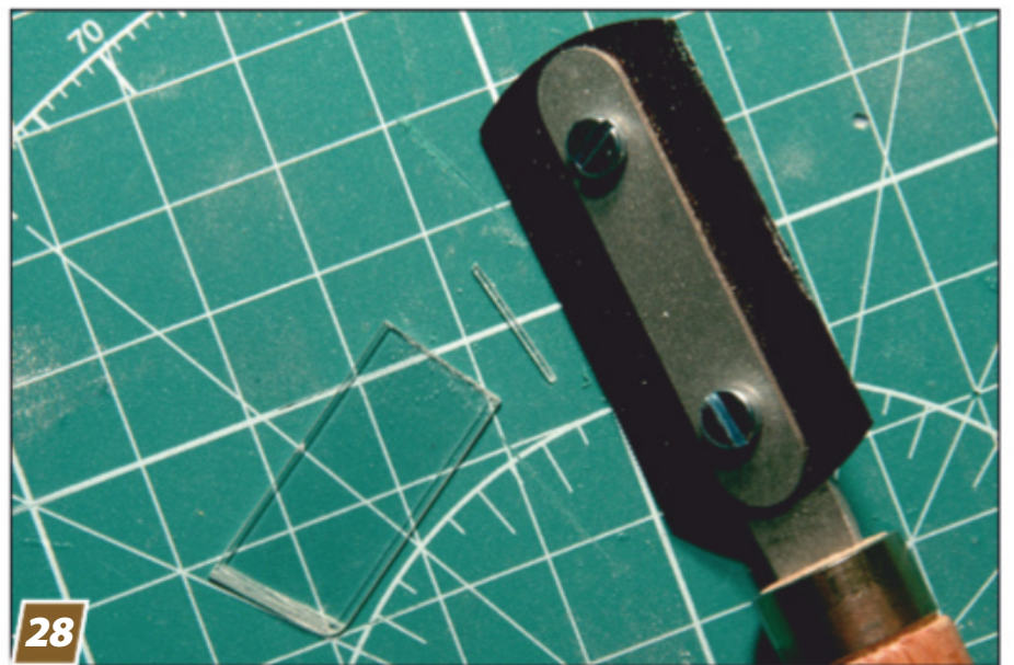
28 Armoring the windshield glass, I sawed the locating ledge from the vertical edge of a kit windshield piece ...
