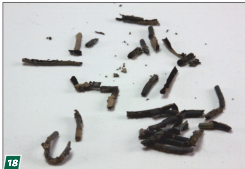
Yikes! With a shelf life considerably shorter than three years, the rubber tubing Bill had used for tie-downs went to pieces ...
