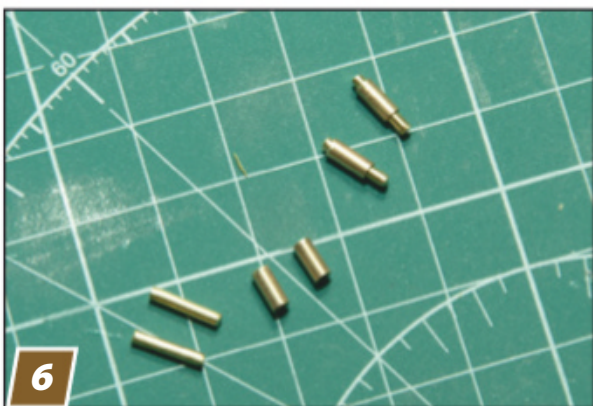
A 7mm section of \frac{1}{16} -inch brass rod telescoped inside a 5mm section of \frac{3}{32} -inch brass round made the shock absorbers.
