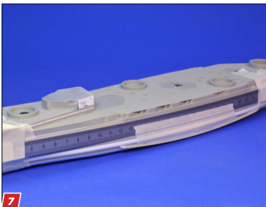
7 A flexible steel straightedge, securely taped to the hull, served as a guide for scribing a locating groove for the torpedo net platform.
