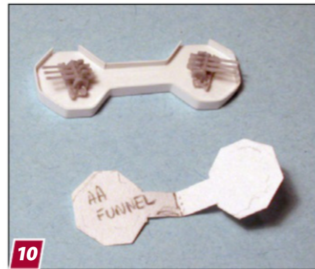
10 To form the anti-aircraft platform wrapped around the funnel, Harvey drew its outline on a folded piece of paper.
