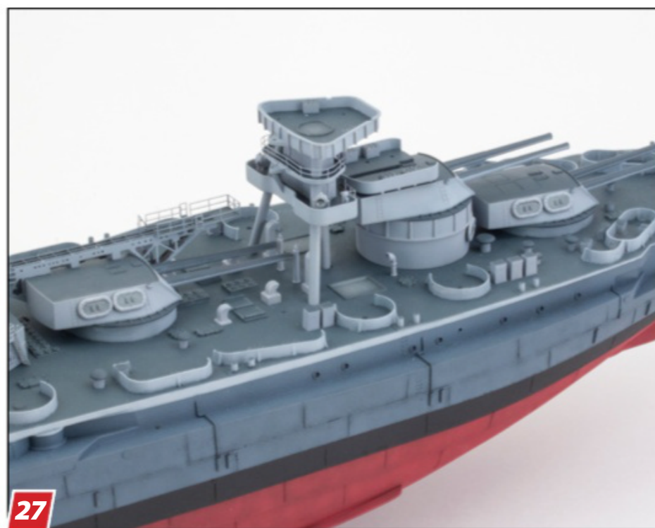
27 Details continue to proliferate on the aft main deck, including Carley floats on the turret sides. Bill kept everything removable as long as he could to be able to test fits.
