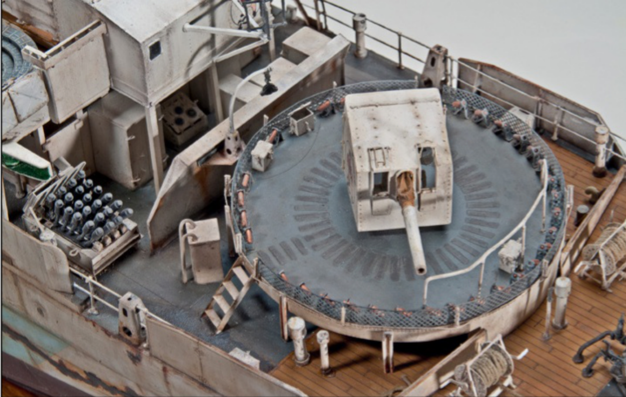
Almost all of the detail on the deck of the Fennel is either PE or scratchbuilt. That includes the weapons, weapons mounts (above), and even the decks themselves (below).
