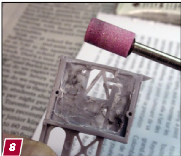
8 To improve the kit's solid-molded searchlight supports, Harvey grinds much of the plastic away from the back side of the parts.
