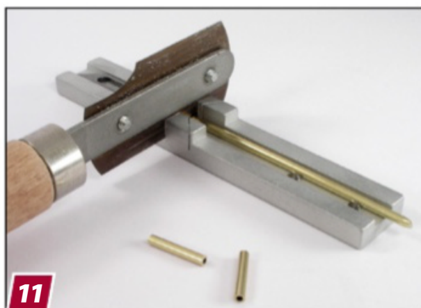
11 Anders disguised the pins with brass-tube sheaths he cut with a razor saw and miter box.
