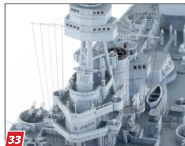
33 Rigging with black EZ Line, Bill begins at the yardarm with lines for the signal flags.
