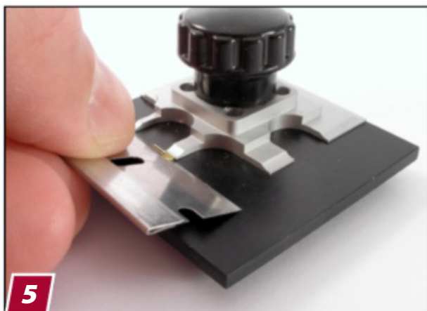
5 "The right tools make the job easier," Anders says. He uses a bending tool to shape most of his PE parts.
