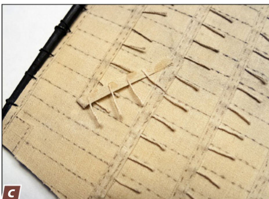
C Attaching reef points: In this front view, the starboard edge of the sail is shown uncovered.
