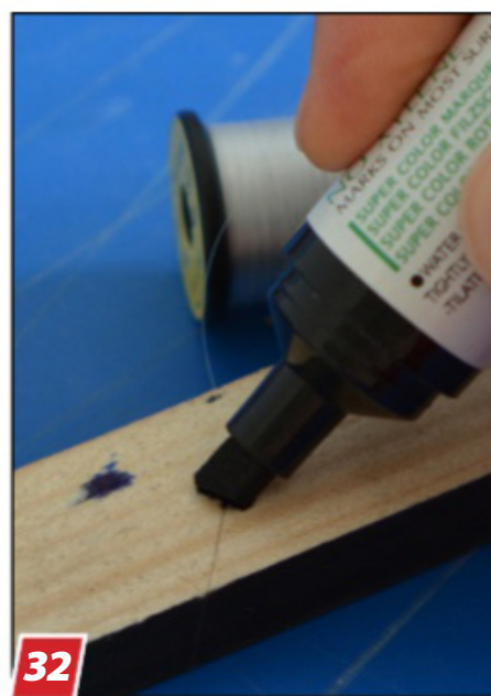
32 Dying transparent line with a marking pen: The line can be straightened by hanging it up with a weight at the lower end.
