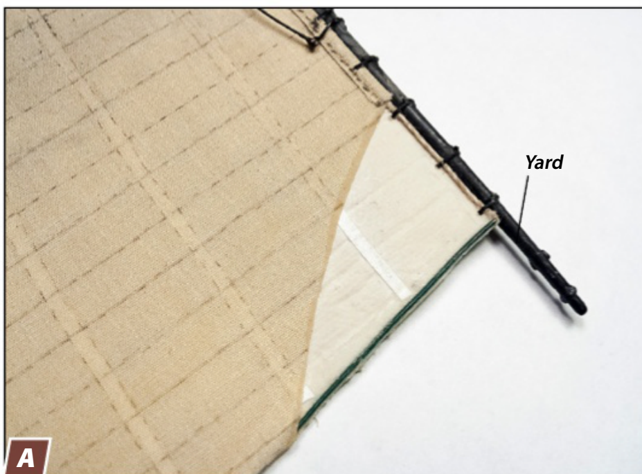
A A cutaway at the top shows thread glued to the top of the core and tied to the yard. Florist wire is on the side of the sail.
