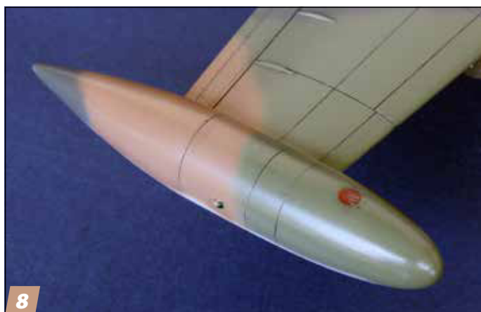
8 Working with tanks from my spares — I'm not sure where they came from — I reshaped them to make the wingtip tanks. I detailed them with filler caps, vents underneath made from .5mm copper wire, and position lights made from styrene rod sanded to shape.
