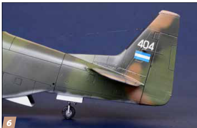
6 The taller tail is the same as the P-51D from the top of the rudder down. Note the directional antenna just above the flag; I cut and shaped them from .5mm styrene.
