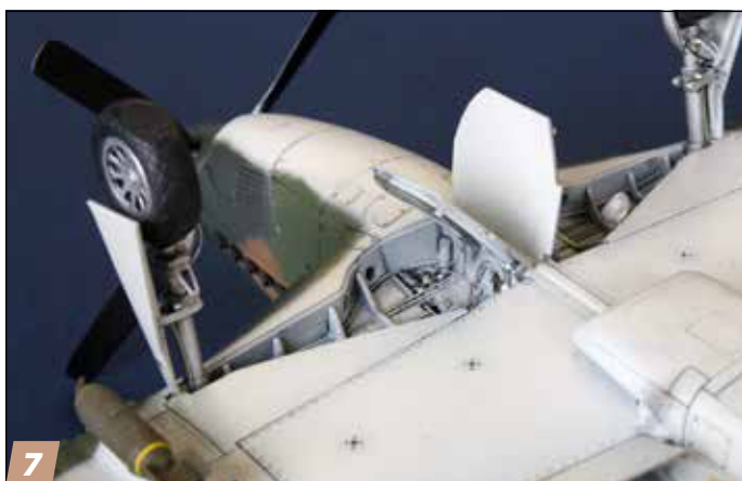
7 I added pipes and wiring to the wheel wells and drilled out structural openings in the front walls; this was difficult to do, so I only opened the innermost pair in each well. I also modified the kit landing light to match Salvadoran references.
