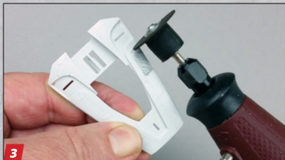
Using a cutoff wheel in the rotary tool, I carefully removed panels near the cockpit.
