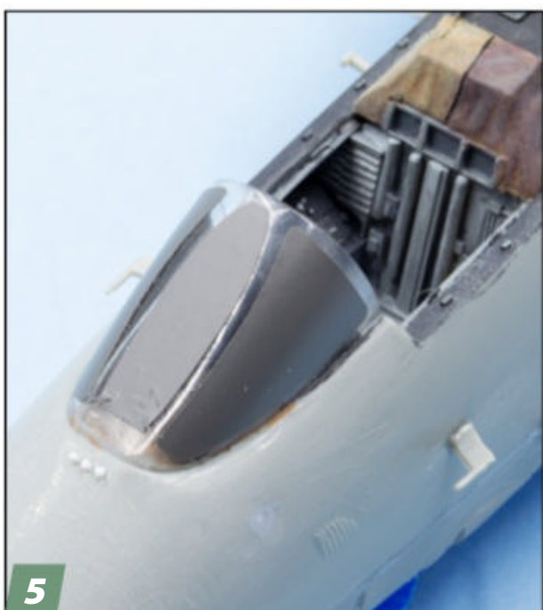
5 The framing molded on the windscreen of the Monogram Tomcat isn't quite correct. After sanding it off, I polished the part back to clarity and applied vinyl masks with the correct shapes. The framing was sprayed black after being glued on.
