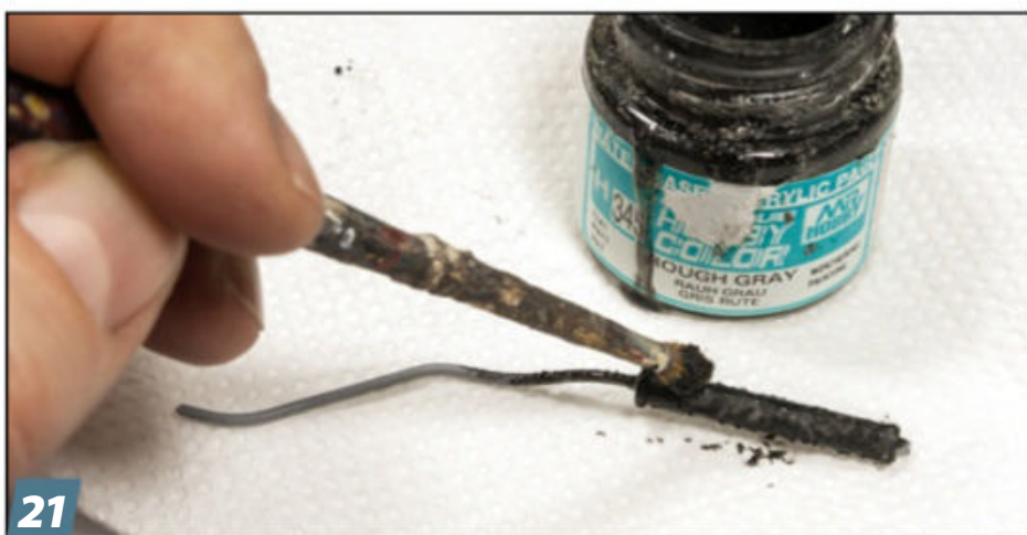
After attaching the photo-etched metal (PE) brackets to the exhaust, I textured the muffler and pipe with Mr. Hobby rough gray applied with a short-haired brush for a corroded look.
