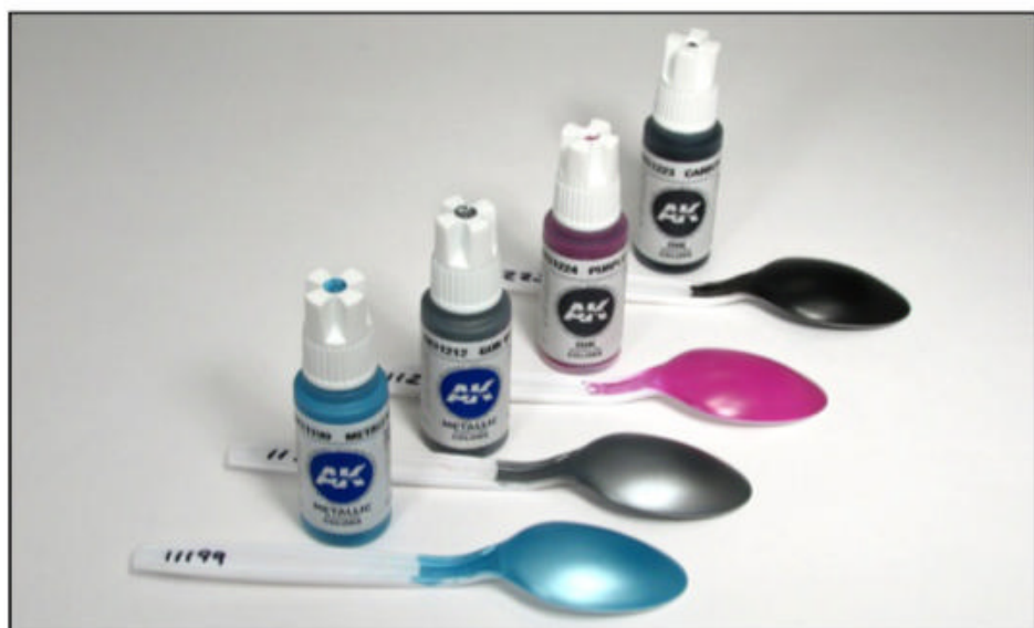
The metallic and ink colors tested. The main parts of the spoons were airbrushed, the areas painted onto the handles were brush painted.
