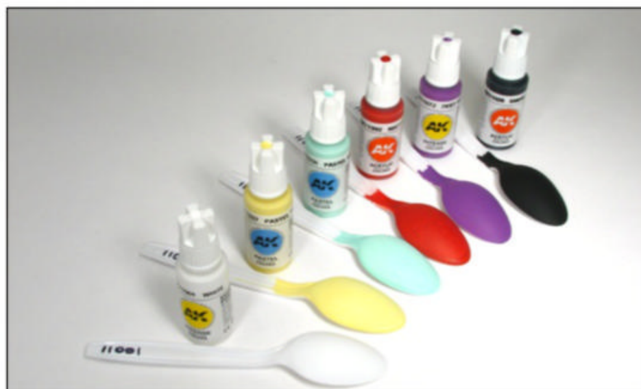
The intense, pastel, and regular acrylic colors tested. The main part of the spoons were airbrushed while the lower part onto the handles were brush painted. The brush painting worked better for me than airbrushing which was a bit tricky to get the colors mixed to flow and cover properly. These paints are essentially odorless and clean up easily.
