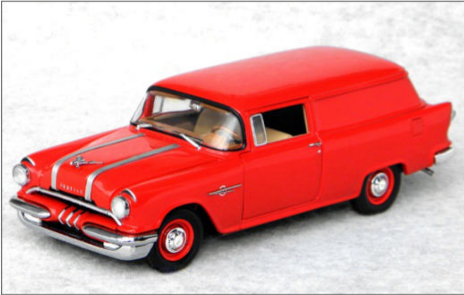
Cliff Read's 1/24 scale '55 Canadian Pontiac Pathfinder sedan delivery began as a low-rider '57 Chevy station wagon toy. He reproportioned the body with styrene, tin, Bondo, and epoxy; scratchbuilt the interior, trim, fuel tank, and parking brake.
