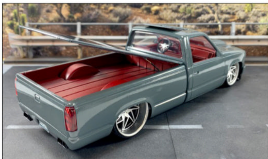
Following many show trucks on Instagram, Nathan Grubb built one of his own from an AMT 1/25 scale Chevy C1500. He scratchbuilt the bed floor and cover, tubbed the rear wells, scrubbed the rear bumper, and installed a sunroof.
