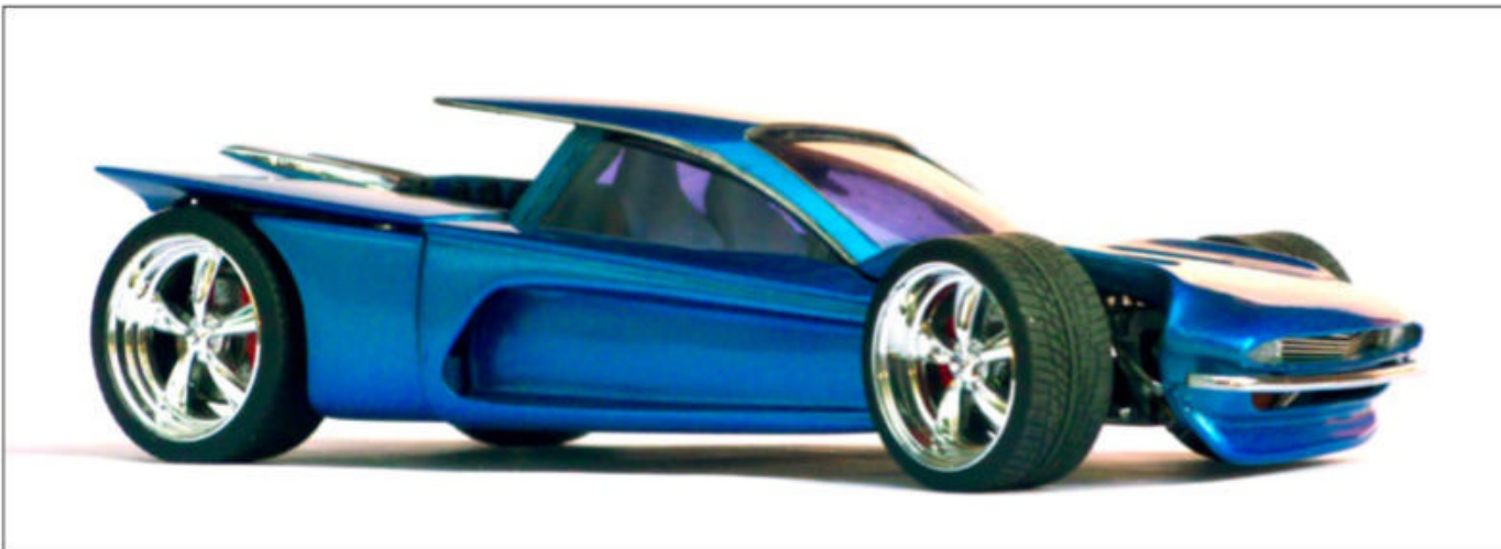
Tim Slesak calls this racy custom El Commotion . To call his mods to an AMT 1959 El Camino radical would be an understatement. Chopped, sectioned, narrowed, and restyled, the body rests on an all-brass chassis with a chrome-plated working suspension.
