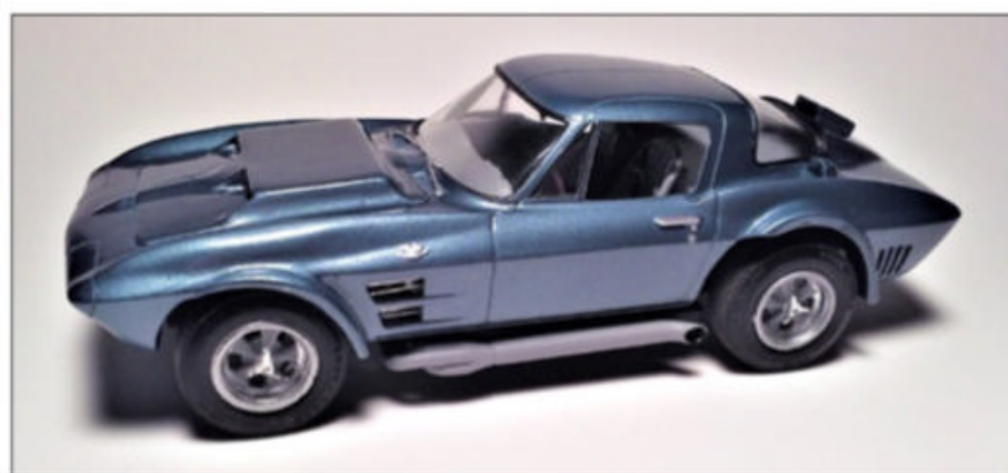
Ken Keltner saw a 1963 Corvette Grand Sport in a book and fell in love. For his model, he used an AMT kit and installed the hood scoop, intake manifold, oil cooler, and fender flares. The side pipes, wheels, and driver's seat came from his spares box.
