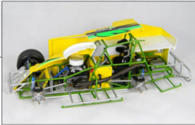
John Rothermel scratchbuilt a 1/24 scale cutaway model of Ron Kline's Dirt Modified race car. He soldered the chassis from 1/16-inch brass rod, and brought in 3D-printed components, like the engine, hubs, brakes and rotors, seat, and coil-over shocks from Custom Dirt Cars. John made the body from .040-inch styrene sheet. The wheels and tires come from ADC Diecast.
