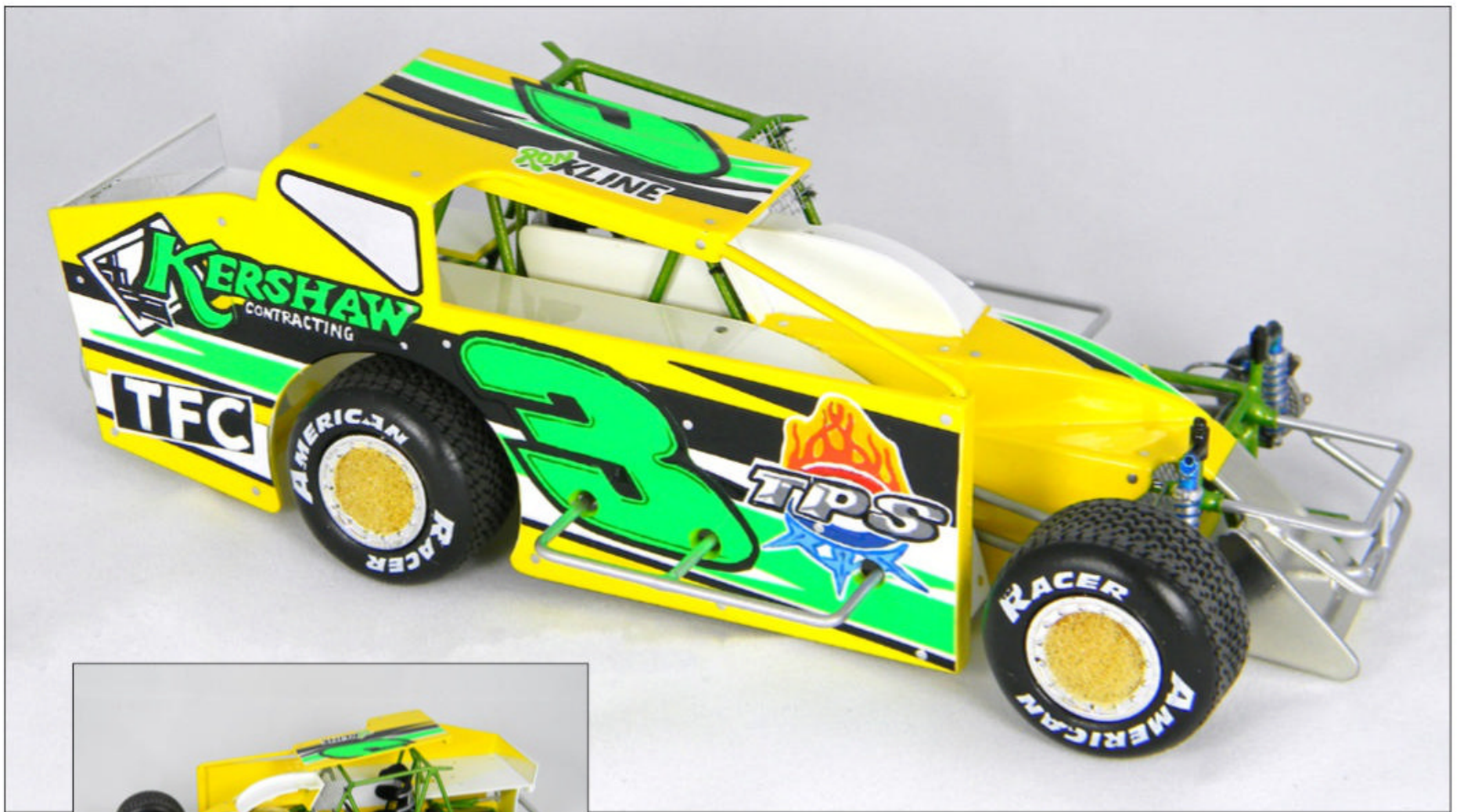
John Rothermel scratchbuilt a 1/24 scale cutaway model of Ron Kline's Dirt Modified race car. He soldered the chassis from 1/16-inch brass rod, and brought in 3D-printed components, like the engine, hubs, brakes and rotors, seat, and coil-over shocks from Custom Dirt Cars. John made the body from .040-inch styrene sheet. The wheels and tires come from ADC Diecast.
