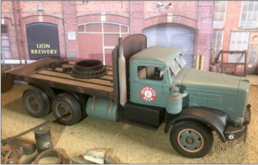
This 1940 Autocar from Bill Borgen uses a American Industrial Truck Models resin body mounted on an AMT Autocar frame. Bill scratchbuilt the bed from balsa wood and styrene. he painted with SEM Green Etch Primer and weathered with pigments.
