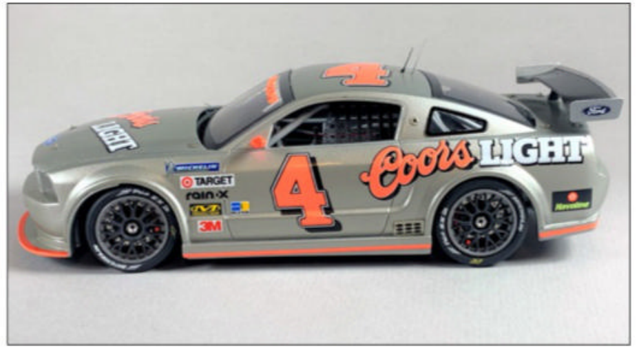
Testors German Silver spray paint covers Robert Davidovich's No. 4 Coors Mustang Road Racer. A fantasy vehicle, Robert designed and photo-etched his own metal brake rotors, front grille, and side exhaust screens.
