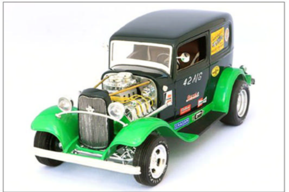
Charles Shinkle built this MPC 1932 Ford panel van box stock, except the engine looked awful bare. He rescued a glue bomb engine, replaced the intakes and carbs with spares, and wedded the mill to a Funny Car transmission of unknown pedigree.
