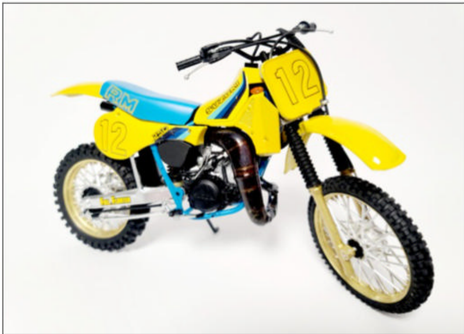
This Tamiya 1/12 scale Suzuki RM250 was built box-stock by Erik Lane. He used Rust-Oleum Sunburst Yellow for the body, Dupli-Color Grabber Blue for the frame, and Tamiya acrylics and clears for the engine and exhaust details.
