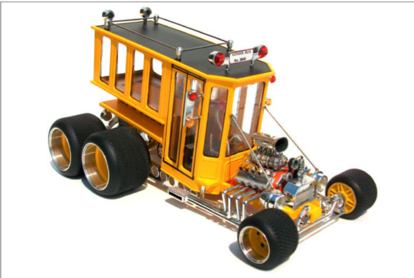
Boban Arsic's Li'l Yeller school bus gave him some trouble at first, with ill-fitting and missing parts. But once he got in the swing, he had fun lowering the front, detailing the cooler with aluminum mesh, wiring the engine, and installing a homemade roof rail.
