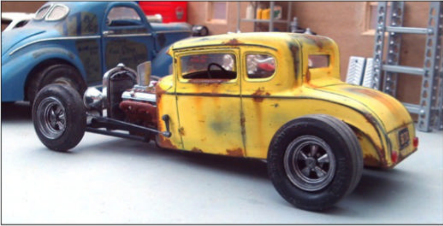
Basically a parts-box build, Mark Hook's 1930 Ford Model A coupe features a scratchbuilt frame, floor, and interior. The rails up front cradle a Mopar 413. Mark painted the body with Rust-Oleum Yellow and weathered with real rust and Tamiya products.
