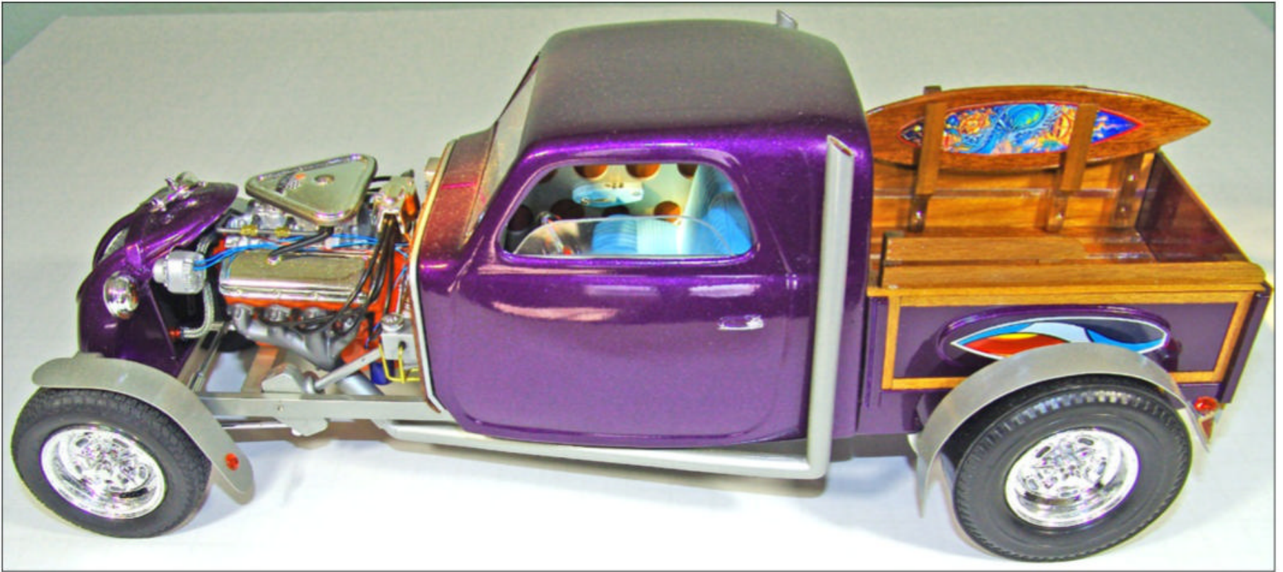
Doug Wallin wanted to build a unique pickup, and the old Lindberg 1/12 scale Fiat Dragster/Cabriolet gave him an idea. He scratchbuilt the pickup bed for his woody from styrene and mahogany, and built a frame from rectangular brass tube.
