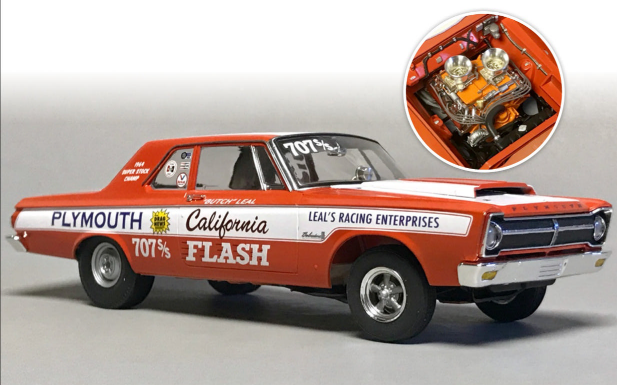
This stunning replica of Butch Leal's California Flash 1965 Plymouth Hemi 426 Super Stock drag car comes from John Barker. Beginning with a Moebius kit, John ratcheted up the detail with Detail Master plug wires, distributor, looms, and velocity stacks; Fireball Resin Holley carbs; fuel lines of .5mm solder; and return springs made from stretched fine wire. Astounding job!
