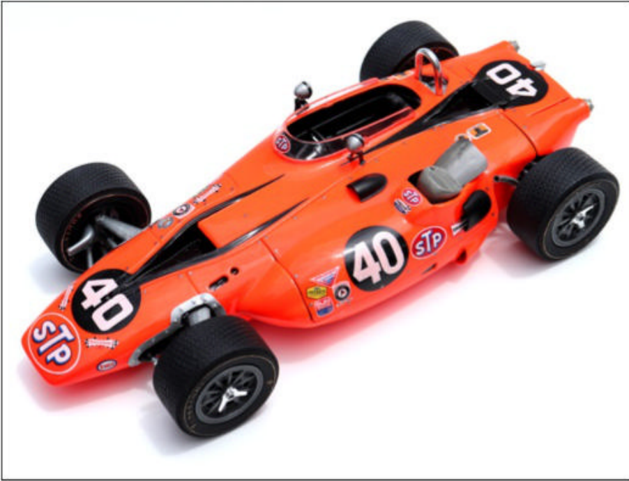
Gene King revisited his childhood by building this MPC 1/20 scale STP No. 40 Indy turbine car. Wanting to do it right this time around, he carefully painted and detailed the car, including an aluminum exhaust shroud and accurate resin-cast tires.
