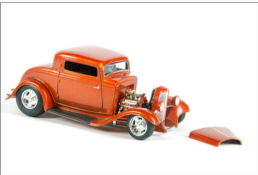
This 1932 Ford coupe hot rod was built by Jim Kampmann. He used his own chopped resin coupe body, lowered the suspension, used a photo-etched metal grille from Model Car Garage, and finished it with Testors lacquer.
