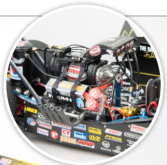
To model a 2007 U.S. Army Top Fuel dragster, John Ruiz updated the chassis from a Revell kit and added fuel lines, a puke tank, 3D-printed magnetos, and carbon-fiber decals. The rail is finished with Tamiya and Revell lacquers.
