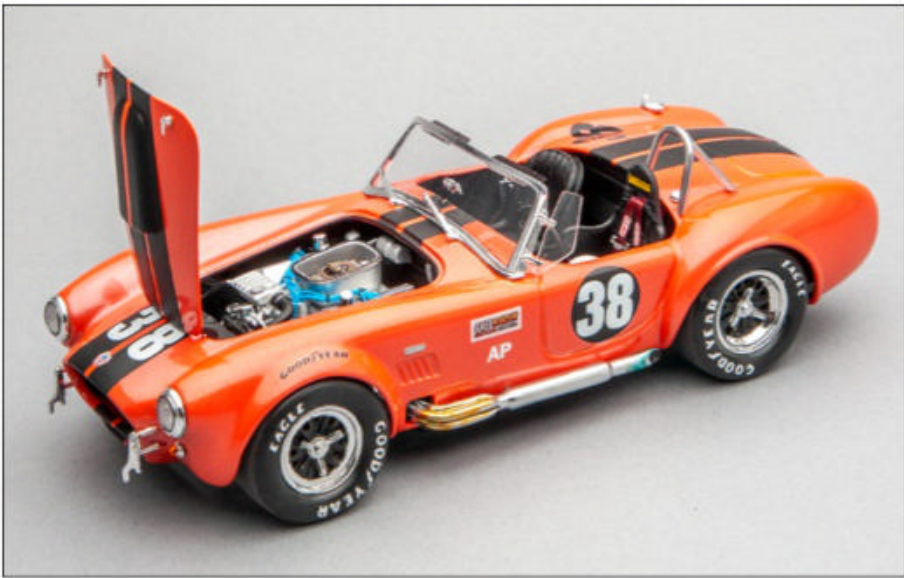
Matt Key imagined his own fantasy race car and set about building it with a Revell 1/24 scale Shelby Cobra 427 SC. He cut the spindles to lower its height, detailed the engine, and slipped NASCAR wheels and slicks underneath.
