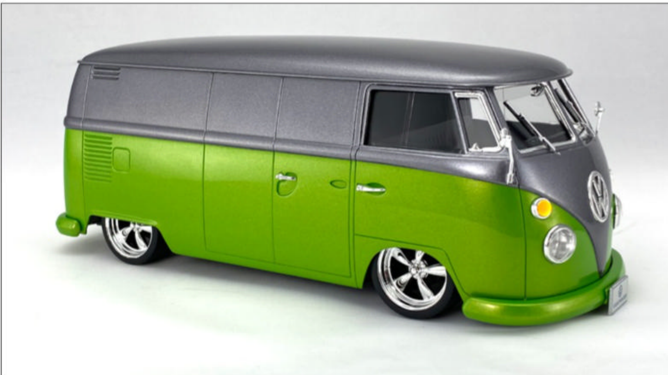
Alex Samardzich aggressively lowered and shaved the trim from a Hasegawa 1967 Volkswagen Type 2 delivery van for this custom. The two-tone paint is Tamiya Light Gunmetal and Candy Lime Green under Gloss Clear. The five-spoke wheels come from Pegasus, and the trim is – what else? – Bare-Metal Foil.
