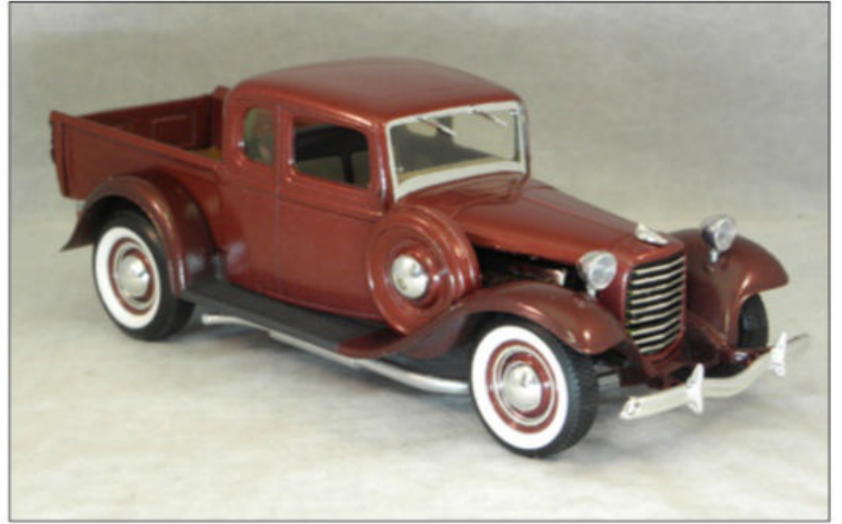
This '34 Ford custom pickup from Dennis Mills utilizes an AMT '32 Ford coupe body for the cab; a shortened bed with basswood and N-scale railroad track; wheels and tires from a Revell '31 Model A sedan; and seats and inner door panels from a '29 Ford.
