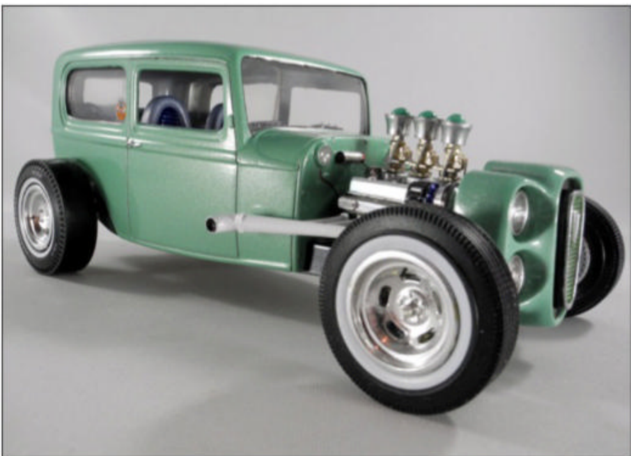
William Just took an AMT '32 Ford sedan and dropped the front axle, changed out the wheels and tires for replacements from a part pack, and removed the running boards. He installed a Halibrand GQ rear end and detailed the Buick nailhead engine.
