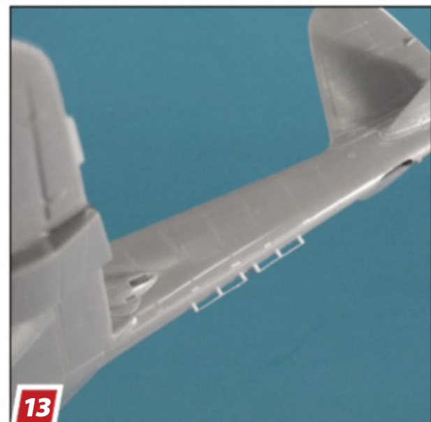
... after using a hobby knife blade to square the rod's edges, I superglued wire over the posts.
