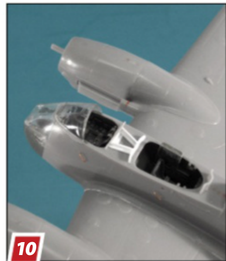
After cutting open the canopy, I added wiring, PE scraps, and sheet styrene for more detail in the cockpit.
