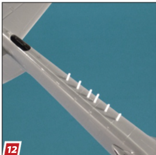
The antennas on the plane's underside removed earlier were replaced with .03-inch Evergreen styrene rod and metal wire. ...
