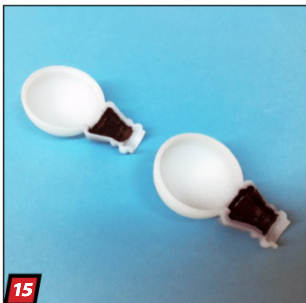
I painted the bottom of the lamp globe black before assembly to block light where I didn't want it to shine.
