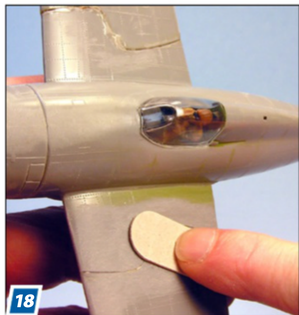
18 I attached the stabilizers, and filled the drop tank holes, wing fold joints, and adjacent sink marks with superglue. I smoothed the seams and restored the mismatched leading-edge shape at the wing fold with emery boards and sandpaper.
