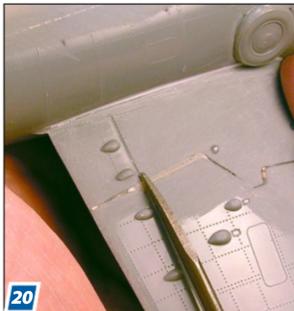
20 Afterward, I restored the recessed flap hinge line with a knife-edge file. With the outer panels attached, I addressed the lack of machinegun blast tubes.
