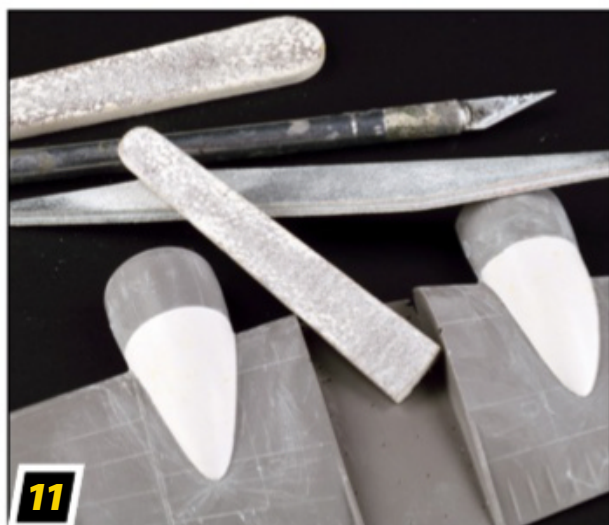
11 A lot of sanding and sculpting was needed to get the nacelles near the right shape. I used several different files of varying coarseness.
