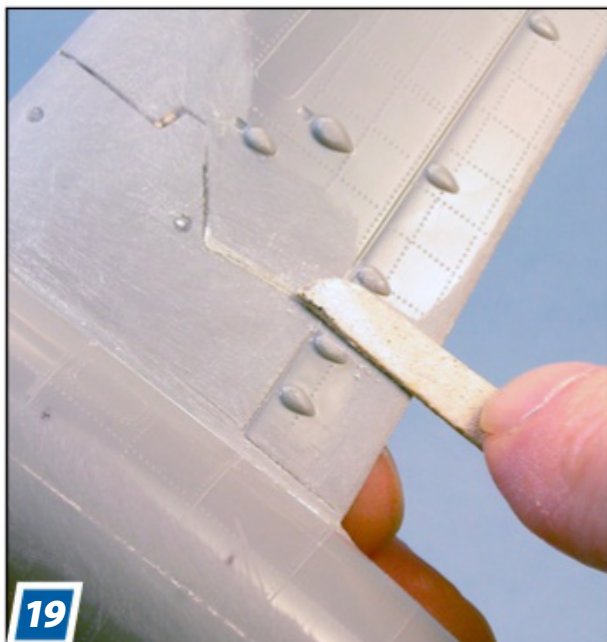
19 Cutting down an emery board with scissors enabled me to smooth the wing joint between the flap hinge blisters.
