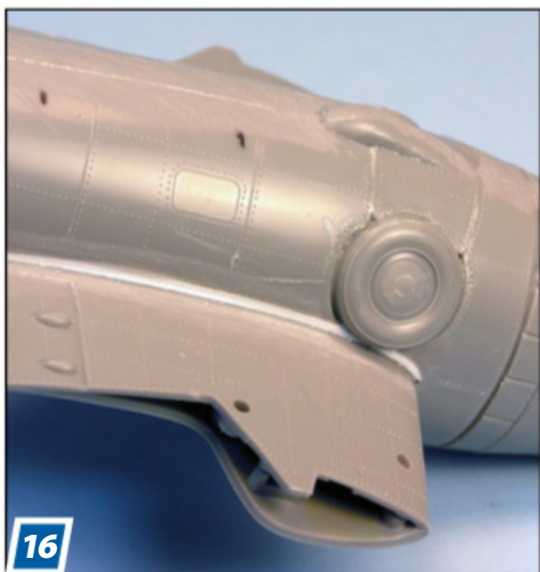
16 After cleaning up the wheels, I added styrene strips to fill gaps under the wing at the wing-root. I smoothed the join, leaving a round notch for the wheels to fit. Now, I could add wheels and doors and fill the gaps with superglue.
