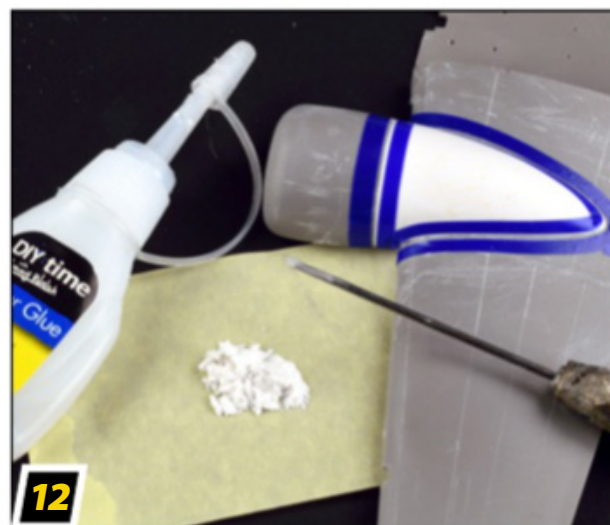
12 A mix of superglue and talcum powder is used as a filler, building up the edges and adding strength to the nacelles' joins.
