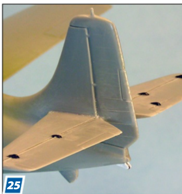
25 Then I added details to the elevator hinge and control tabs with scrap plastic. I also added the rear towing and tail hook bracket under the tail cone. Finished with construction, I now gave it a thorough wet-sanding to start with a clean slate.
