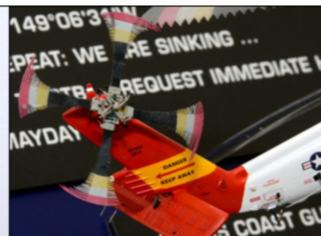
15 Making the tail rotor appear to spin was easy. I used PropBlur PE blades and detailed the hub with PE bits from the Eduard sheet, and some thin wire. Painting some pink and gray on the rotor's outer edges also enhanced the illusion of motion.
