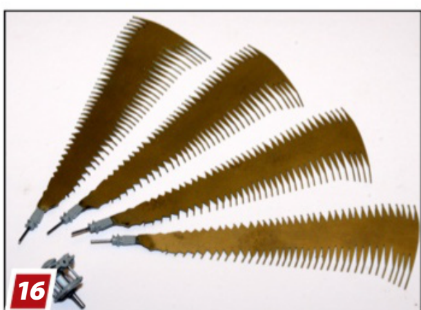
16 I designed my own PE main rotors. A small German company reproduced them for me at minimal cost. I also replaced the rotor shaft and pins with metal rods.
