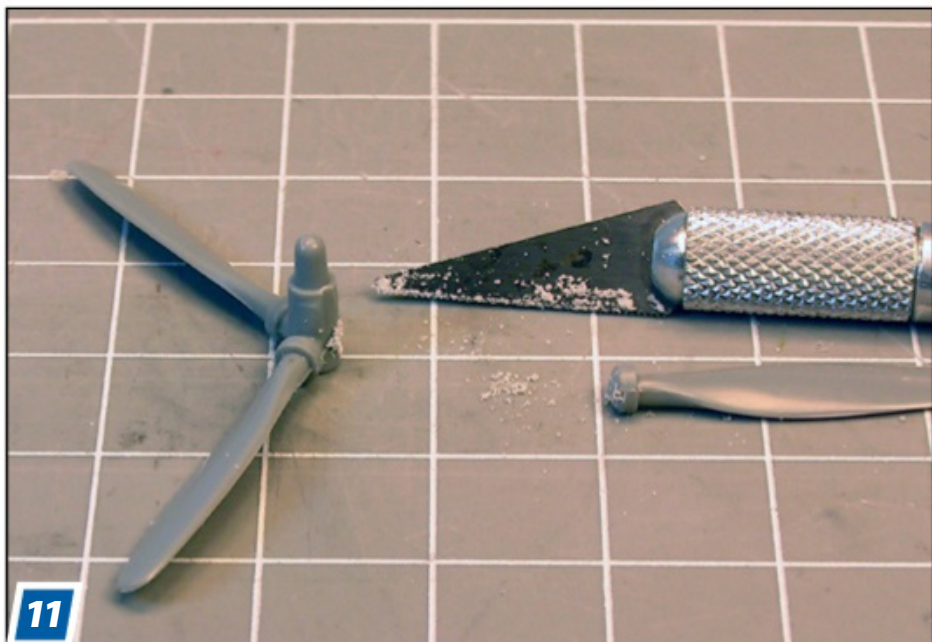
11 Since the kit's uncuffed prop isn't correct for an FM-1, I modified it with blades from Tamiya's 1/48 scale Wildcat. First, I removed the blades with a micro saw, as close to the hub as possible. Then, I secured the hub to a shaft of 1/16-inch diameter brass tube with superglue.
