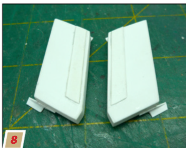
8 Some flails were fitted with these boxes from which powdered chalk ran out of the bottom as flailing was underway, marking a cleared lane behind the tank.
