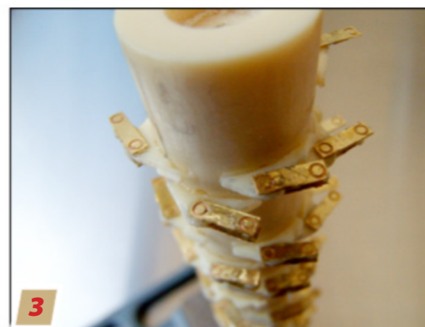
3 Studying photos and inspecting a real example at a museum revealed there were four rows of seven and four rows of six flail attachments spaced around the drum.
