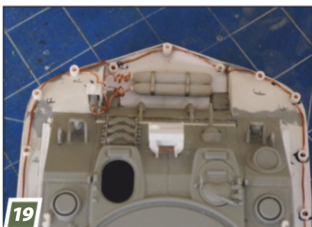
19 The air regulator unit was fabricated from scrap sprue, styrene profiles, and wire. Once finished it was all fixed in place on the hull.
