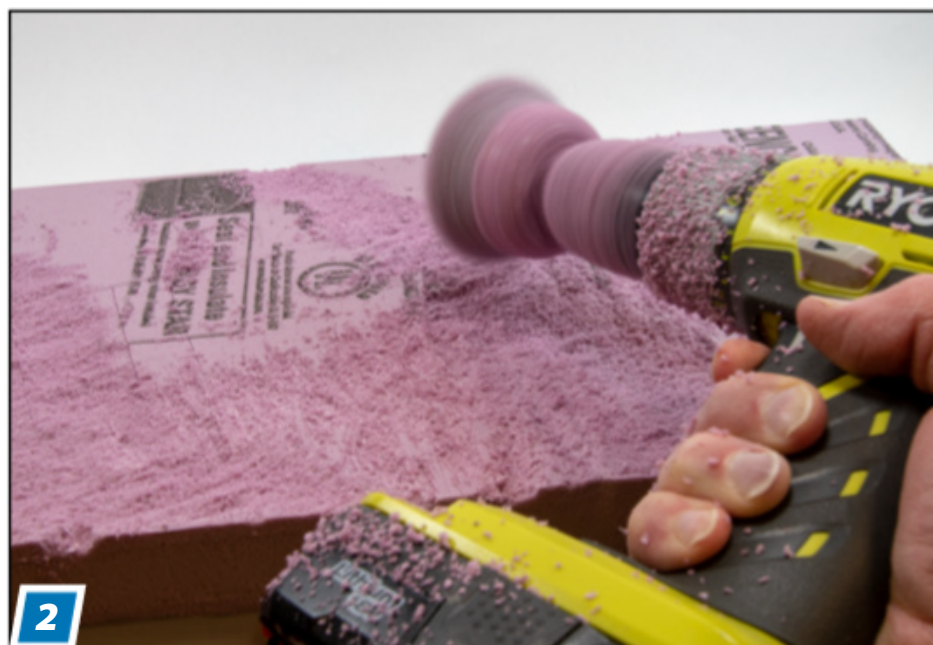
The next couple of steps are messy, so do them somewhere you can clean up easily. Using a coarse drill cup wire brush in a power drill, I first carved the troughs in the sea. I wanted them deep enough to notice but not so deep as to risk swamping the LCVP.
