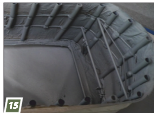
15 The front strut supports were made of styrene rod and scrap wire.
