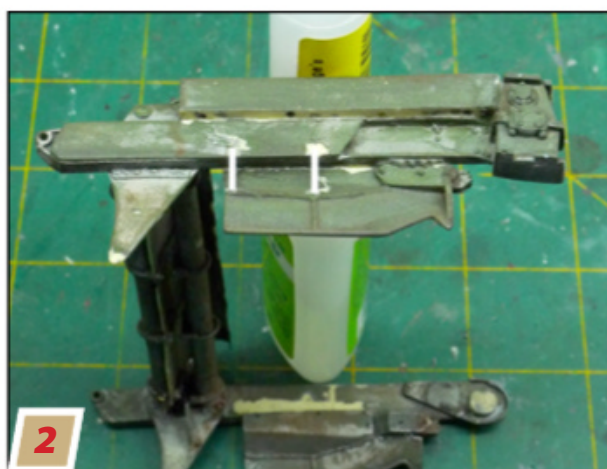
2 Here is the flail arm assembly lightly glued together and ready to be fitted to the hull.
