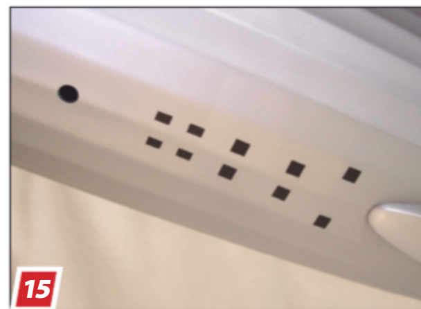
15 Black square decals were used to represent openings along the keel.
