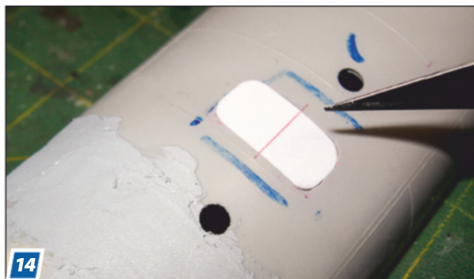
14 Rolling the new door around a small screwdriver handle matched its curve to the fuselage. I removed the tape and placed the door.
