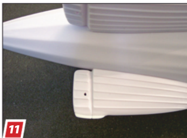
11 A thin strip of styrene modeled a bumper guard on the lower tailfin.
