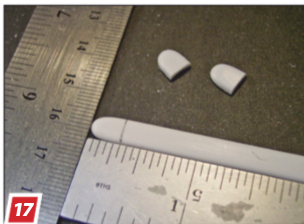
17 I carved and sanded gas shaft vent covers out of styrene.
