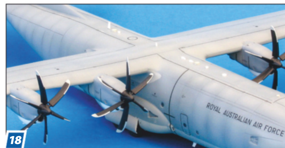
18 The propeller blades did not exhibit the correct twist off the sprue. To feather them, I twisted each of the blades ever so gently. Then, I glued the props and spinners in place.
