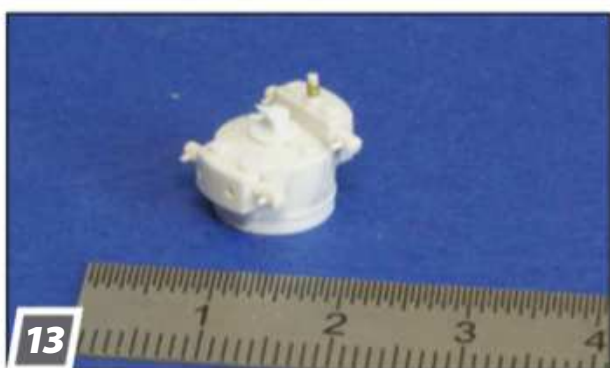
13 With most components in place, the piece can be cut loose and the last fragile details added. The rangefinder is now finished.
