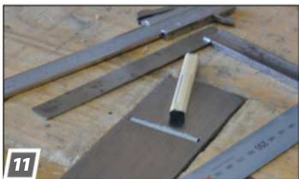
11 Shaving a small piece by pulling it over an upturned plane. Watch your fingers!
