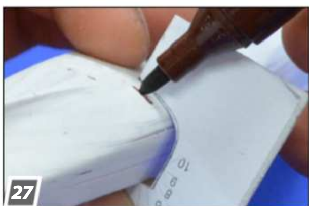
Refining the hull shape: I mark where the frame template touches the hull.
