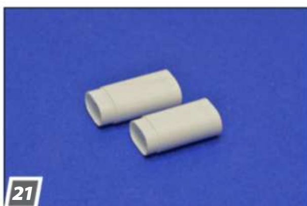
21 Making a funnel: I wrapped three layers of .3mm styrene sheet around a stick, taped it, and dipped it into boiling water. After cooling, the sheet can be cut off, removed from the stick and glued together again.
