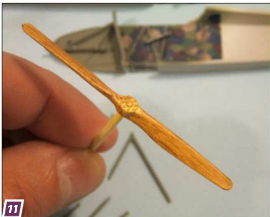
11 Dragging artist's oils across a tan acrylic base coat replicates grain on the propeller and other wood parts.
