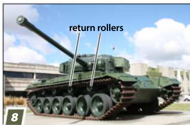
Suspended track supported by return rollers on an A41 Centurion. This tank has a bogie suspension.
