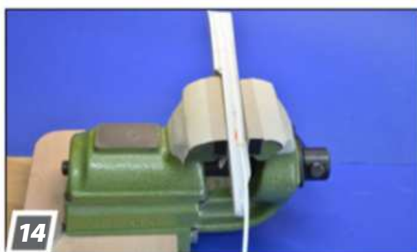
14 A high-quality vise holds the hull while .1mm strips are being glued. Cardboard over the jaws prevents damage.
