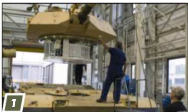
1 Anniston Army Depot (ANAD) employees guide a repaired turret, complete with turret basket, to an M1A2 hull.
