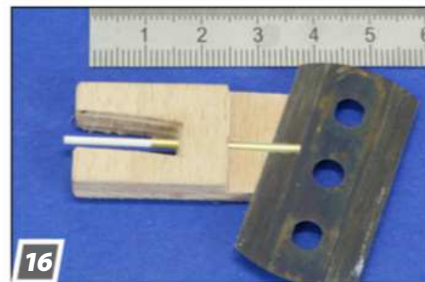
16 A small plywood jig holds a torpedo tube while I saw it to shape. I inserted styrene rod to keep the tube from being deformed.
