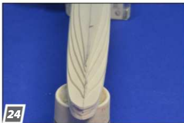
I glued the hull together in layers: The centerlines of the layers have been carefully aligned.
