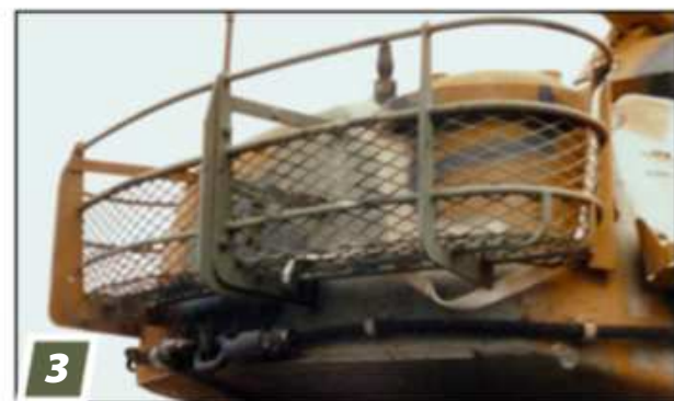
3 The large squirrel cage on an M60A3. The expanded steel screen kept crew gear intact (although there were never any guarantees).
