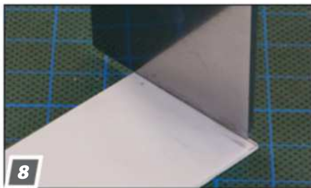
8 On thicker styrene sheet, make the first cut slightly outside of your scribed line. Plant the chisel in the scribed line and press from above.
