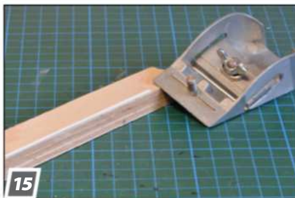
15 Double-sided tape can hold a strip of styrene to be planed or sanded to shape. This cheap plane uses a razor blade, but it's worth it to buy a higher quality block plane.
