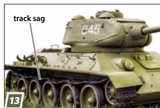
The Soviet T-34/85 with dead track that is unsuspended and sags along the upper run.
