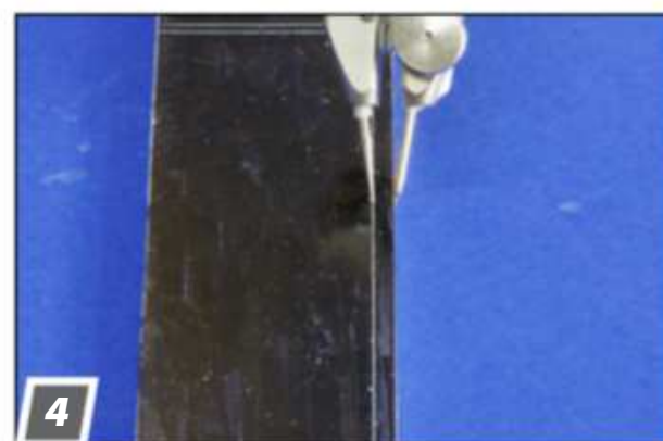
Put one point of the dividers at the edge of your material and press the other point gently into the material. Then pull the dividers along the edge for a straight, true mark.
