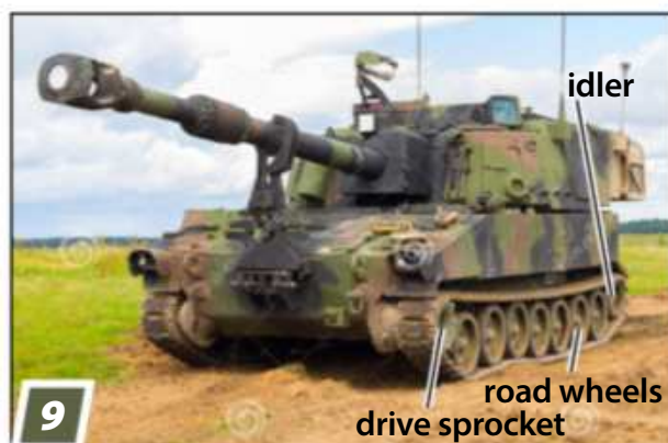
A U.S. M109 howitzer with flat track supported by the drive sprocket and idler. This vehicle has torsion bar suspension.
