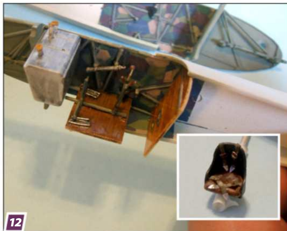
12 Cockpit appointments were spartan — styrene rod and fine painting detail the space. Belts, buckles, and a cushion make the seat more plush.
