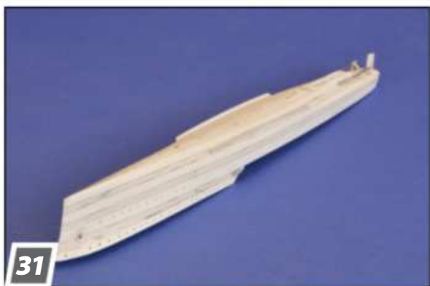
31 The finished hull with propeller shafts, rudder, plating, bilge keels and portholes.
