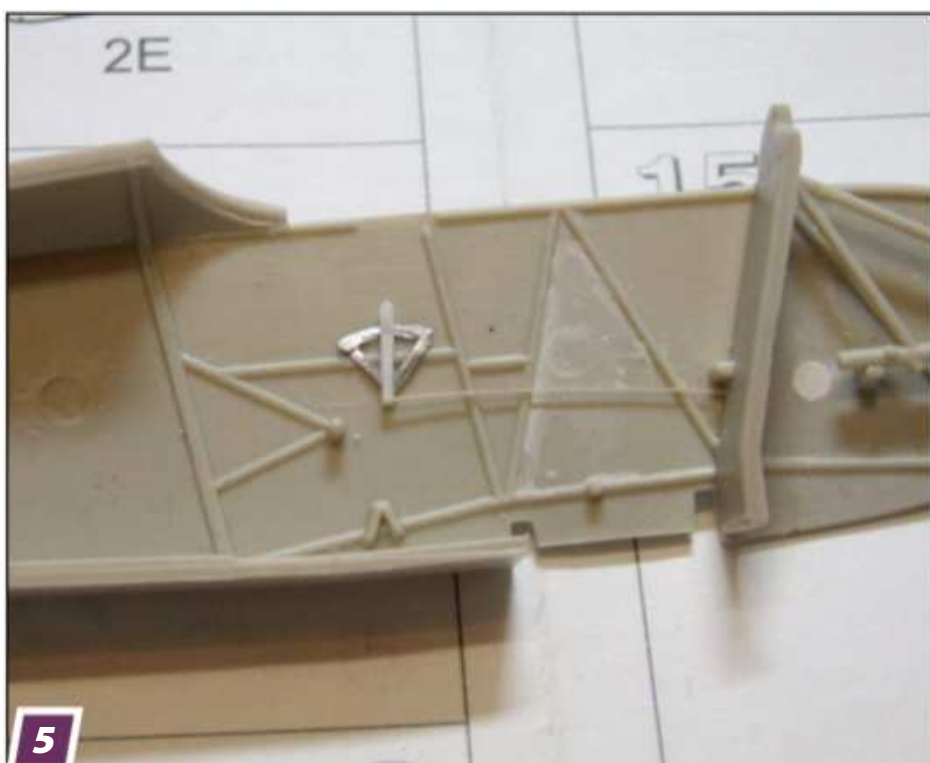
5 Added detail on the cockpit wall was removed to apply lozenge decals.
