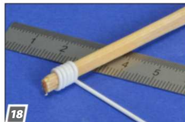
18 Making life rafts: Secure styrene rod by sticking it through a hole in a dowel, dip it into boiling water, and wind the rod around the stick by turning the stick and gently stretching the rod.
