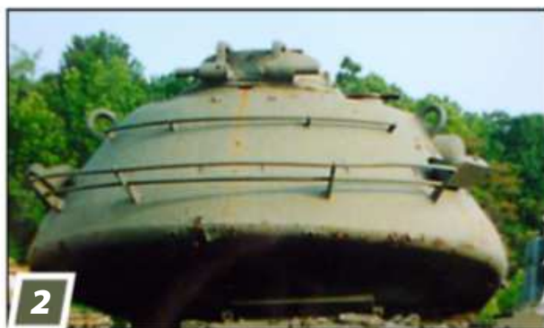
2 The bustle on a T-43 120mm gun tank at Fort Knox. Without caged sides it's easy to see how this was known as a bustle rack, as it resembles the wire frame once worn under clothing, also called a bustle. It supports gear with straps.
