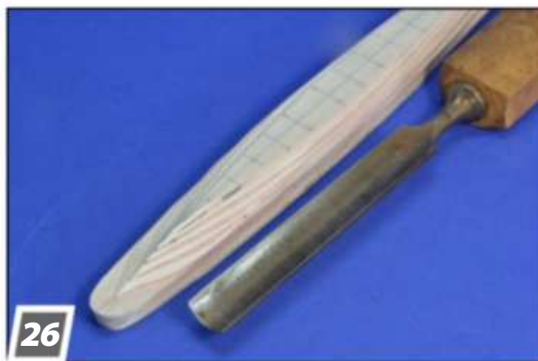
Initial rough cuts to shape the hull were made with a gouge. Old chisels, well sharpened, are often better than new ones.
