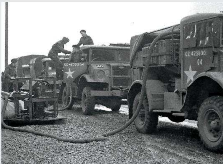
15-cwt 200-gallon water tankers making a pickup. The second vehicle in line is from an infantry division headquarters. These trucks usually had a frame and canvas top over the bodywork to appear more ordinary to enemy observers.
