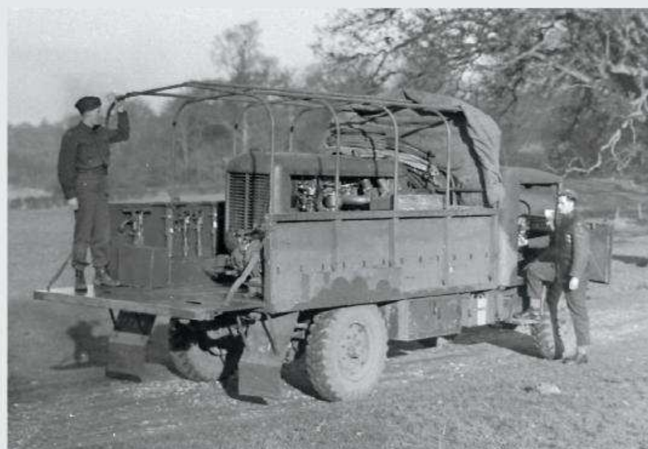
Canadian ingenuity: A Royal Canadian Engineers CMP 3-ton GS has been converted to a compressor truck to power road-breaking equipment (like jackhammers). Typically, these compressors were towed; mounting one inside the body makes it quicker to use.
