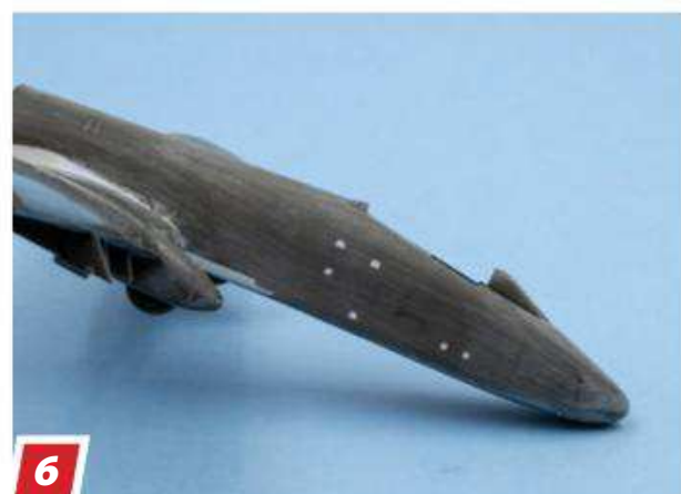
6 I also used the putty to fill in locating holes for the Pave Penny mount, vents, and strakes, none of which were on the prototype.
