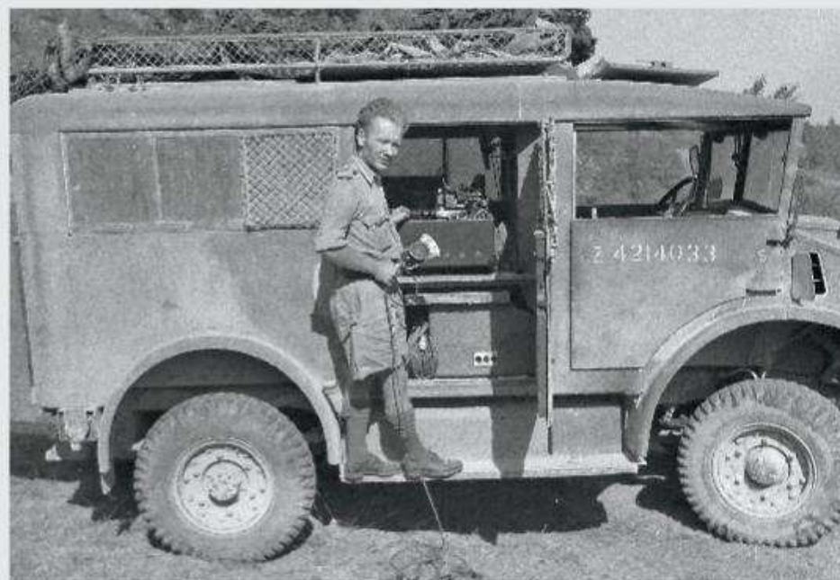
Chevrolet C8A heavy utility fitted out as a mobile recording studio for Canadian Broadcasting Corp. war correspondents in Italy. Interviews and battle noise were recorded on discs that were sent out for radio newscasts.
