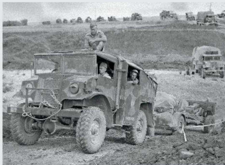
Cab 13 Chevrolet FAT of an unknown field regiment towing a 25-pounder gun/howitzer and limber through a streambed in Italy. Almost all the vehicles following are CMP trucks.
