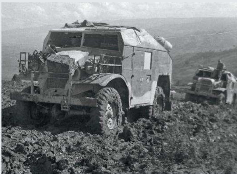
Cab 12 Chevrolet Field Artillery Tractors (FATs) from the Field Regiment RCA trying to cope with a muddy battlefield. This is the Chevrolet version of the Ford FAT, as modeled by Tamiya. Racks on the front fenders are for 2-gallon petrol/oil/water containers.
