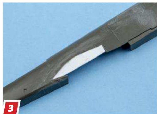
3 ... and filled the void with sheet styrene, cut to shape.
