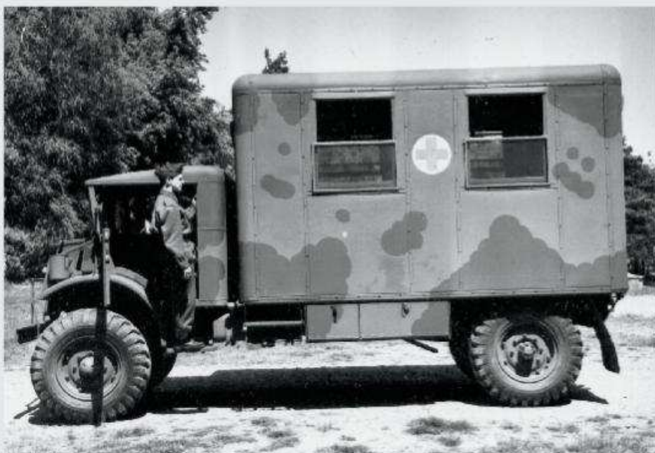
Chevrolet C60L with Lindsay mobile dental surgery bodywork. Developed by the Lindsay Co. of New York, the bodies had interchangeable panels for multipurpose use as ambulances, mobile workshops, and wireless vans.
