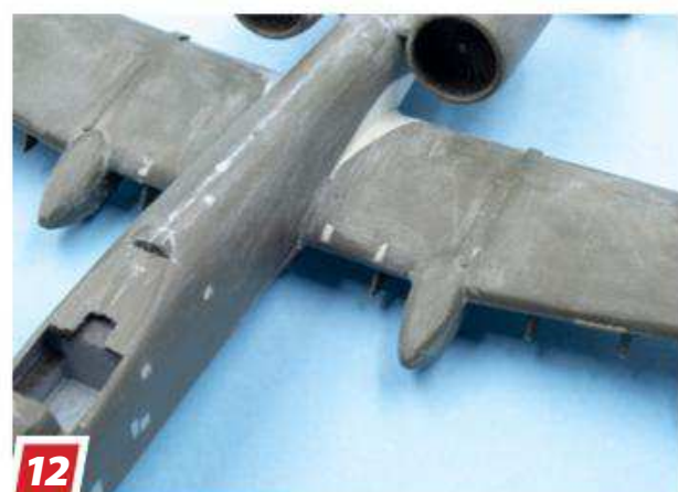
12 I filled in locating holes for the leading-edge slats with more two-part epoxy and sanded them smooth.
