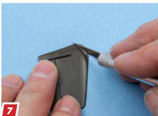
7 The vertical tails were different, too: The original's leading edges reversed direction near their base. I cut the kit parts with a hobby knife ...
