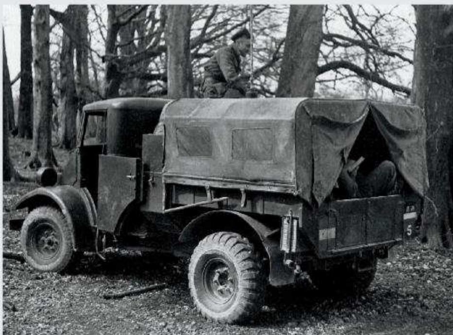
An 8-cwt wireless truck in service with 3rd Field Regiment, Royal Canadian Artillery, England, 1941. The canvas top could be removed and used as a shelter supported by folding legs.
