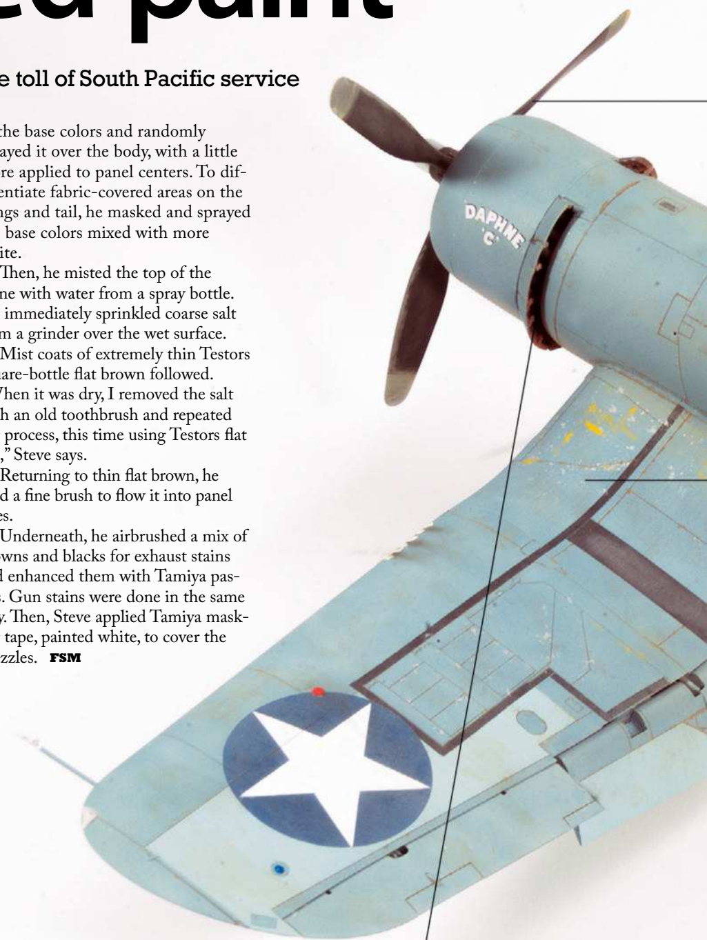
Engine: The engine cylinders were painted with Alclad II aluminum, and the crankcase with Testors square-bottle gloss gray. Steve applied a black enamel wash to emphasize details.
