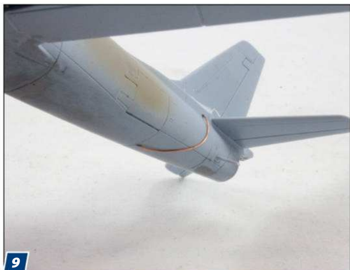
9 A telemetry cable curved from the ventral centerline up the port side to the stabilizer fairing. I added it using copper electrical wire.
