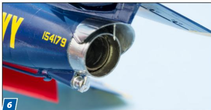
6 The angled pipe injects paraffin directly into the exhaust, which is then dispensed in the form of colorful smoke under the "sugar scoop," seen here on the finished model.
