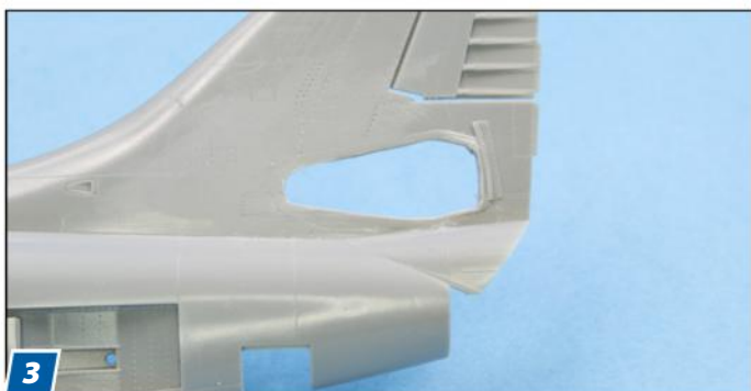
3 To re-pose the horizontal stabilizers, I cut away the molded sliding plates to make way for resin replacements.
