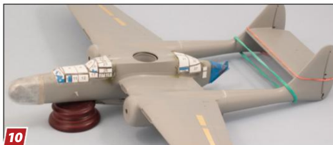
10 After gluing the wings, I let them set up before using rubber bands to pull the tail booms together slightly to connect with the rear stabilizer.
