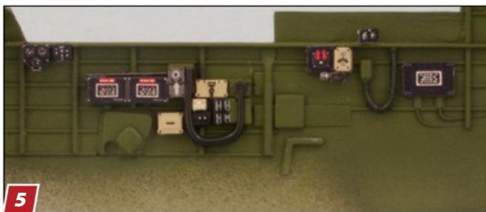
5 Here is the right side of the front cockpit with PE upgrades installed.
