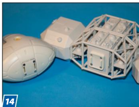
14 I super glued the magnets into holes on the command module and front passageway. After drilling pilot holes with a bit in a pin vise, I reamed them out to the proper diameter with a hobby knife.
