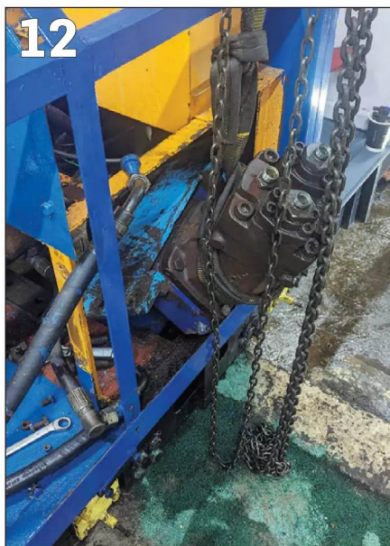
PHOTO 11: Reconfiguring the sprockets to try and get the chain into a space to clear everything.
