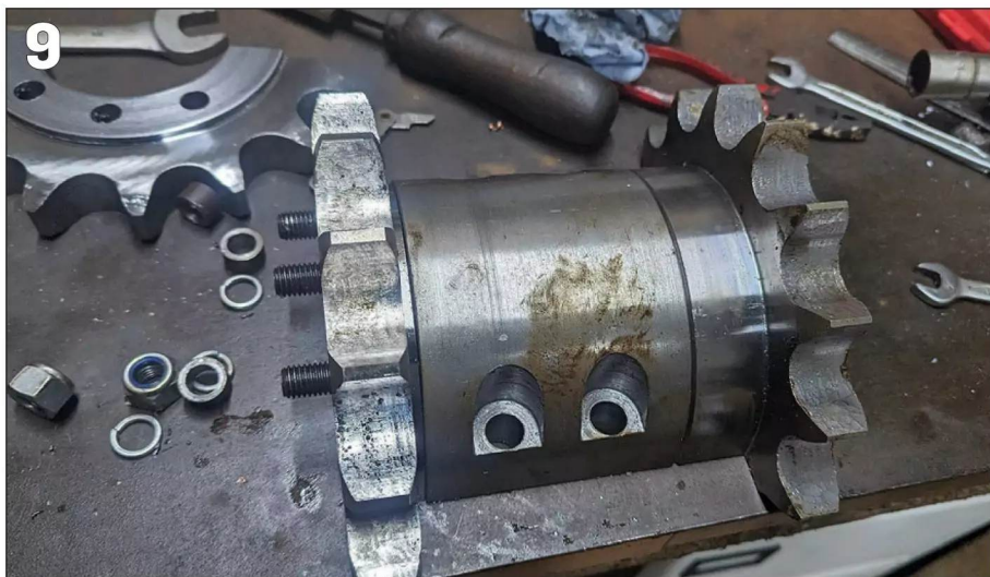
PHOTO 10: With the clamps in place Harry could line up the sprockets and discover the chain would pass through the motor...
