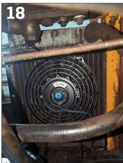
PHOTO 17: With the frame stretcher out of the way Harry took the opportunity to occupy the space to remove the old hydraulic cooler fan. This shows the tight confines that our correspondent occasionally has to work in...
