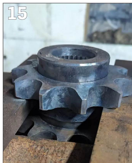
PHOTO 15: Heat and the press was enough to move the sprocket enough to clear the chain rivets.
