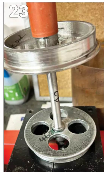
PHOTO 15: Turning the back down to correct thickness.
