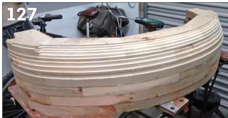
PHOTO 127: Cab former built up and rough-routed to shape.
