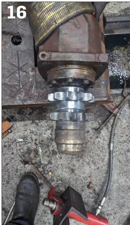
PHOTO 16: You can see the extra space between the sprockets now the carrier is back on the hydraulic motor.
