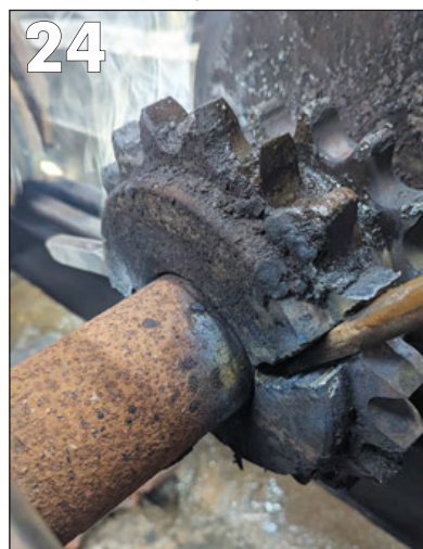
PHOTO 26: The axle appears to be in pretty good condition.
