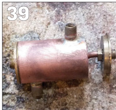
PHOTO 39: Shell of heat exchanger can see full boiler pressure as axle pump feeds water supply. Test before fitting.
