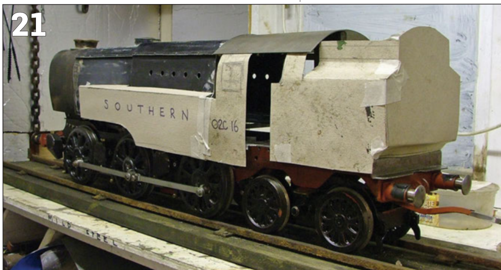
PHOTO 21: First mock up of the platework; the bunker was fine but cab sides and tanks were refined later.
