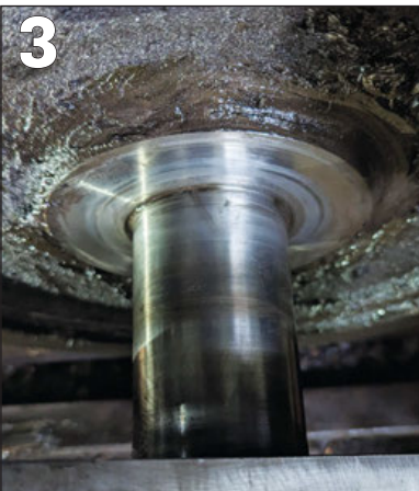
PHOTO 5: The matching score in the bearing material.
