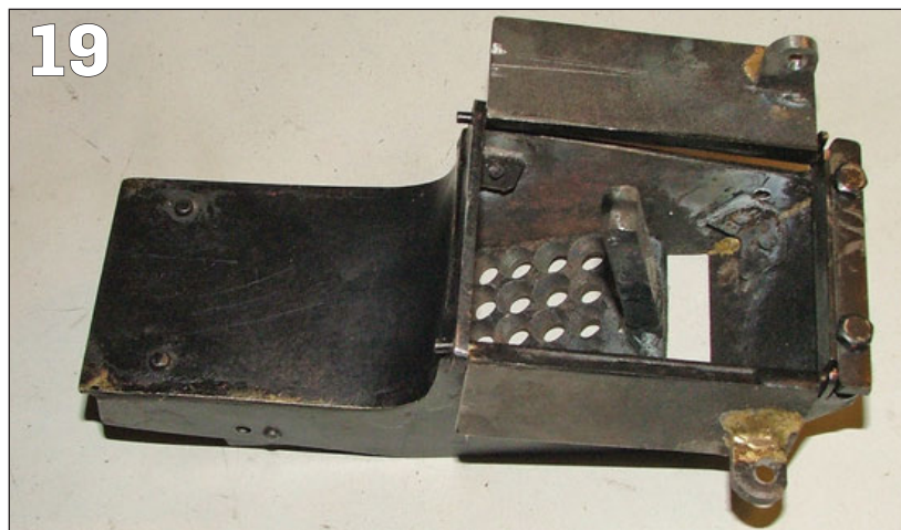
PHOTO 19: Ashpan and grate remain fixed to the boiler, disposal of the fire is achieved by removing the pin that drops the grate and hopper doors together.
