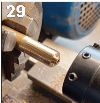
PHOTO 29: Threading the adjuster with die in tailstock.
