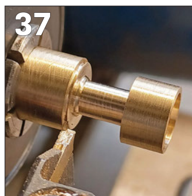
PHOTO 35: The guide turned, faced and then centre-drilled.
