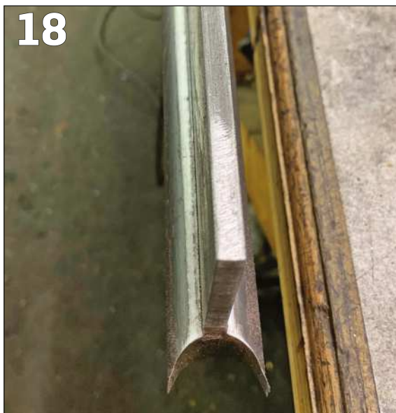
PHOTO 18: The bracing bar fits beautifully in the slot. The machining of the semi-circular arc was detailed in an earlier article (EIM April 2022).
