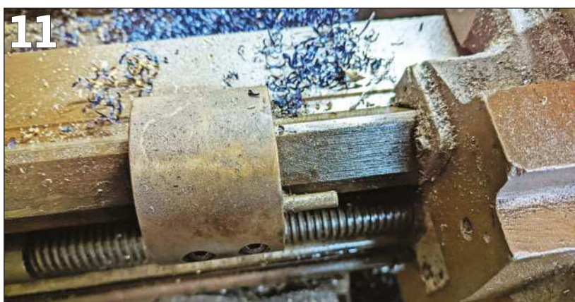
PHOTO 12: Part-machined axle end – small amount of material still needs removal for correct final length.
