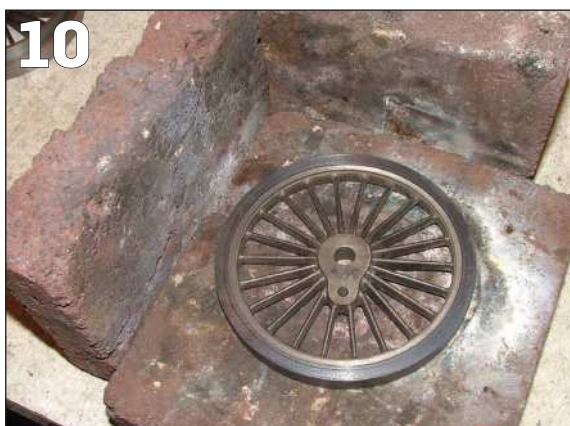
PHOTO 12: The 6ft 7-inch coupled wheel of 'Cheltenham'. The balance weight is opposite the coupling rod pin.
