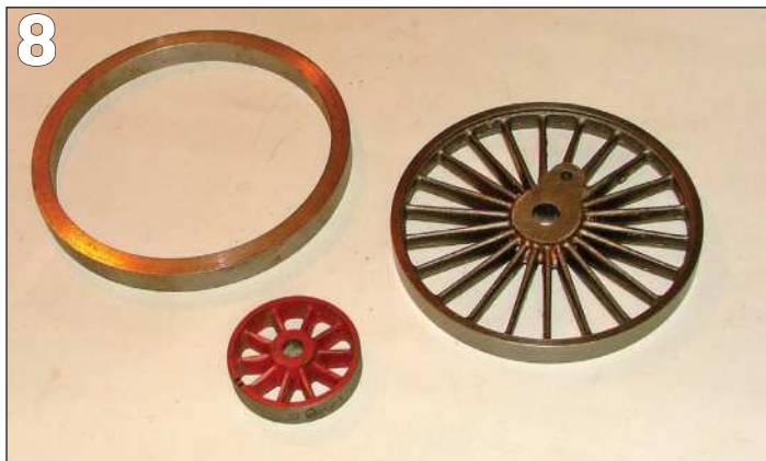
PHOTO 8: All the loco's cast iron wheels were turned down or ground off to accept mild steel tyres. The tyres were machined from thick-wall steel tubing.
