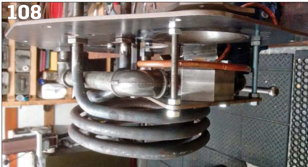
PHOTO 108: Side view of superheater and blast nozzle assembly.
