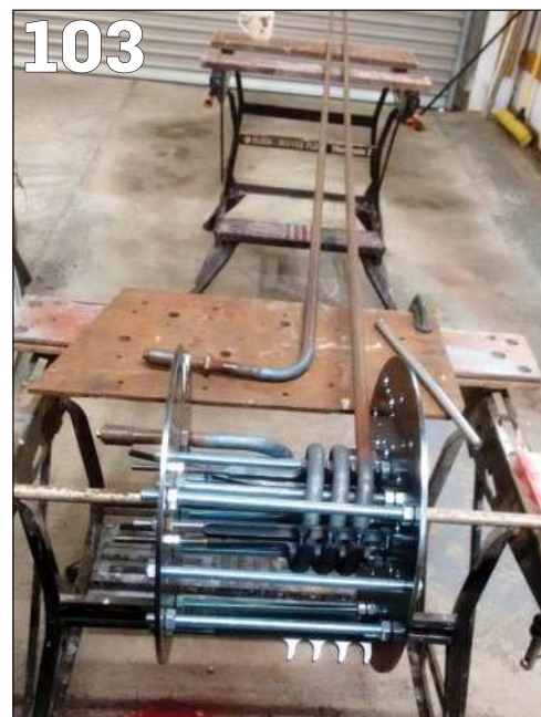
PHOTO 103: Coil winding from the operator's position. Note support axle for the jig and length of pipe to be coiled.
