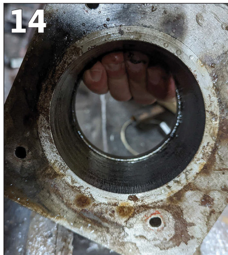
PHOTO 13: Pressing the second axlebox apart only the vesconite came out, not the steel carrier.
