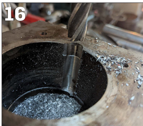
PHOTO 20: Some of the axleboxes had grub screws holding the vesconite and carriers in. Inset shows four grub screws for two holes – across the three axleboxes this way there were two different thread sizes.
