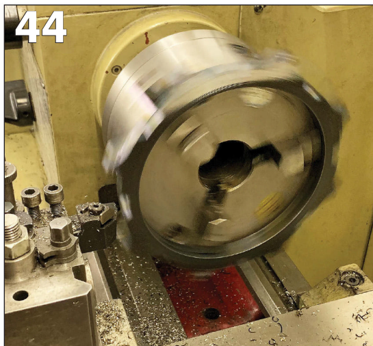
PHOTO 45: Parting tool being used to cut 'slots' to (ultimately) accommodate the brake hangers.
