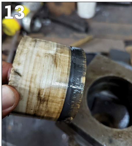
PHOTO 13: Pressing the second axlebox apart only the vesconite came out, not the steel carrier.
