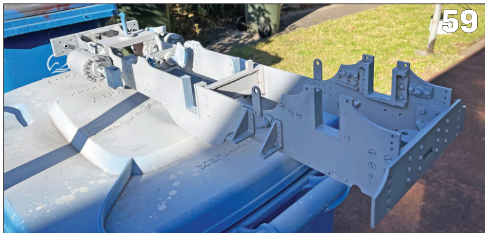
PHOTO 59: Frames, cylinders and valve chests kept together for painting.
