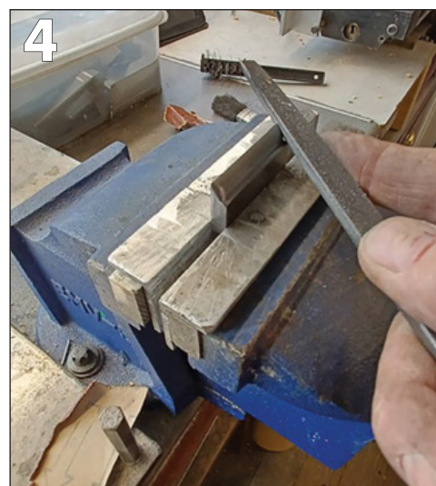
PHOTO 4: Punch finished by having its corners rounded over to match.
