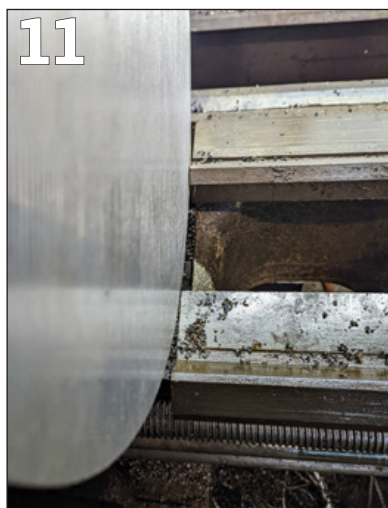
PHOTO 9: Small relief put in where clamping section meets extension, so any flashing or swarf on a lip does not hold workpiece off the jaws.
