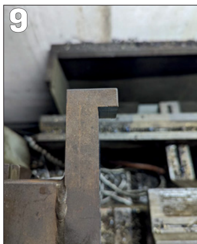
PHOTO 7: Machining chuck jaws to suit blank size, here thinning down to allow blank to drop into the gap bed on the lathe.
