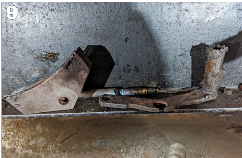
PHOTO 9: The offending hanger with its spacer – Harry had to cut the pin with a gas axe to get it and the brake block off.
