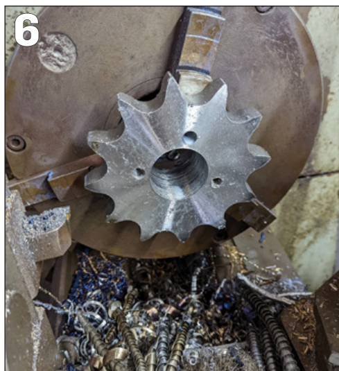
PHOTO 7: With top slide angle set approximately, machining carried out until close to finish size before testing fit. Here it is only contacting at the bottom of the hole.
