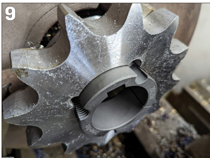
PHOTO 10: The witness mark towards the left of the bush shows the angle has been over-adjusted.
