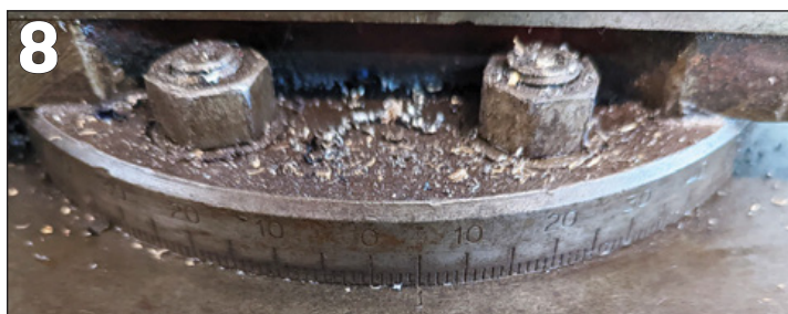
PHOTO 7: With top slide angle set approximately, machining carried out until close to finish size before testing fit. Here it is only contacting at the bottom of the hole.
