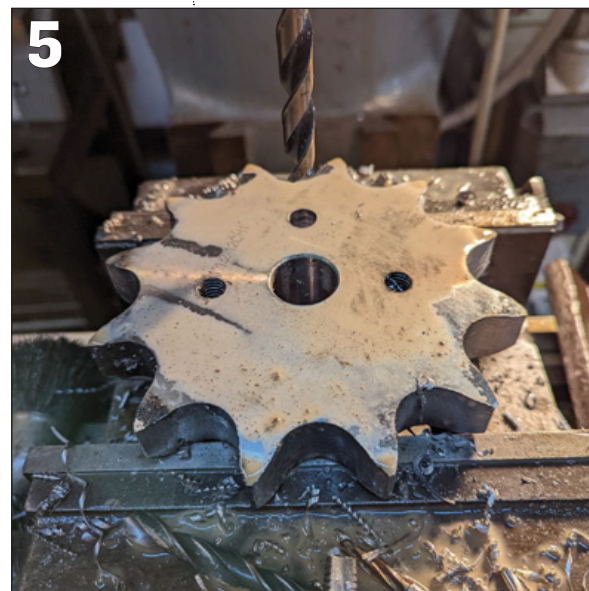
PHOTO 6: Set up in the lathe, the first thing to do was to drill out the central hole as big as possible.
