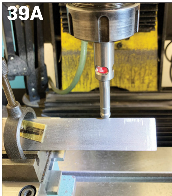
FIGURE 39A/B: Re-checking that bar is level by a different means; (a) reference position and (b) measurement position.
