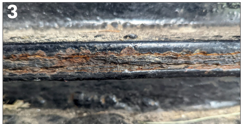
PHOTO 2: One of the welds split on a carriage.
