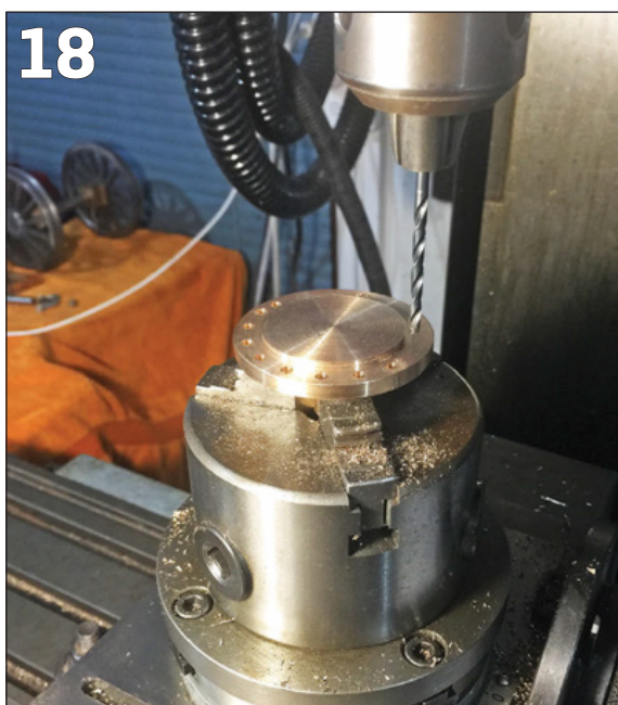
PHOTO 19: Careful measuring and machining needed for slide bar mounting tabs on cylinder rear covers.
