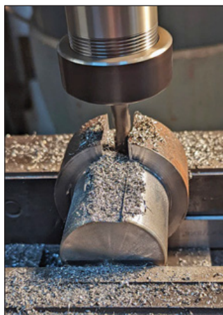
3) Machining the broach guide, a simple turning job before using an end mill to cut a slot – a tight sliding fit for the broach. Depth of slot is important for the first pass.
