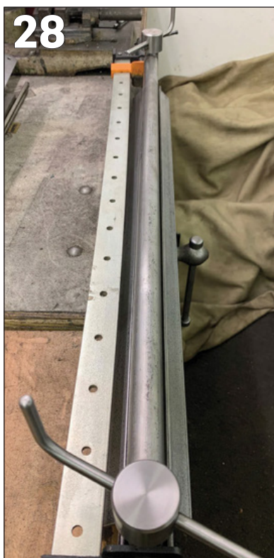
PHOTO 26: Alternative (captive) method of configuring base-section. Now single piece of angle can be welded into place along its length.
