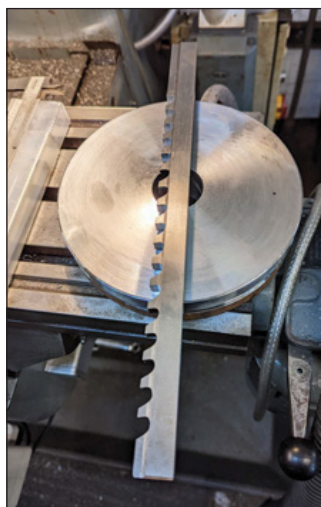
1) The broach sitting on the crank blank. Note the taper as the teeth go up the broach.
