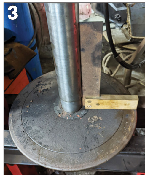
PHOTO 02: Machining the keyway into the axle end – Harry intentionally put the key towards the journal so that when he fitted the cranks, he had a place to rest it on before lining the keyways up.
