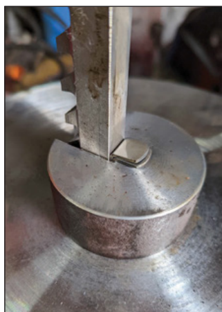
5) The broach part way through a pass, with 2 x 1.5mm shims added – this is the amount of material removed in each pass.
