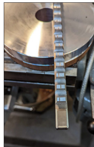
2) Different view of the broach, the small lines in the teeth are to help the chip break off.
