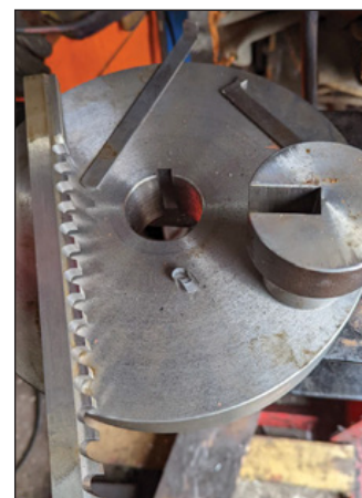
6) Broach, broach guide, shims and crank blank with a perfect keyway cut into it. Also shown are the chips that the broach cuts.
