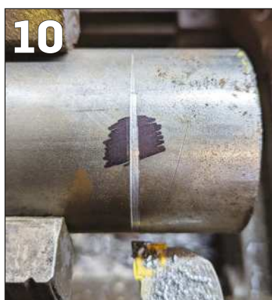
PHOTO 9: Tool tip carefully aligned with the scribed mark.
