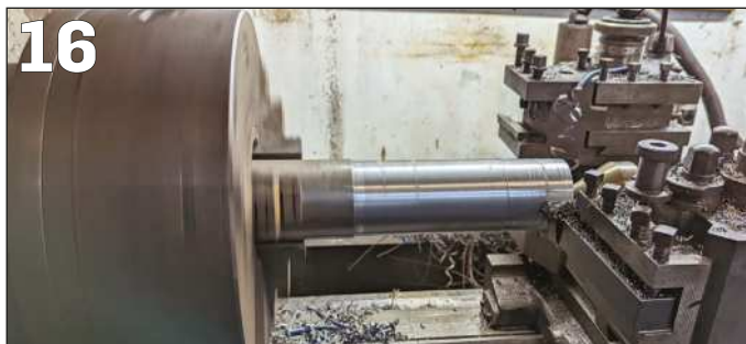
PHOTO 18: Final polish of bearing journal surface to make it as smooth as possible and exactly to size.
