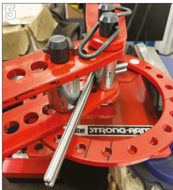
PHOTO 2: Bending/flaring tool configured for (a) flaring, (b) bending and (c) sharp-bending.
