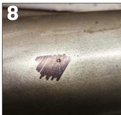
PHOTO 6: Axle stub shows just how thin material was needed to make press work.
