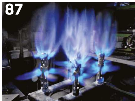
PHOTO 87: Four burners on a manifold made of flattened copper tubing, with threaded brass nipples silver-soldered on.
