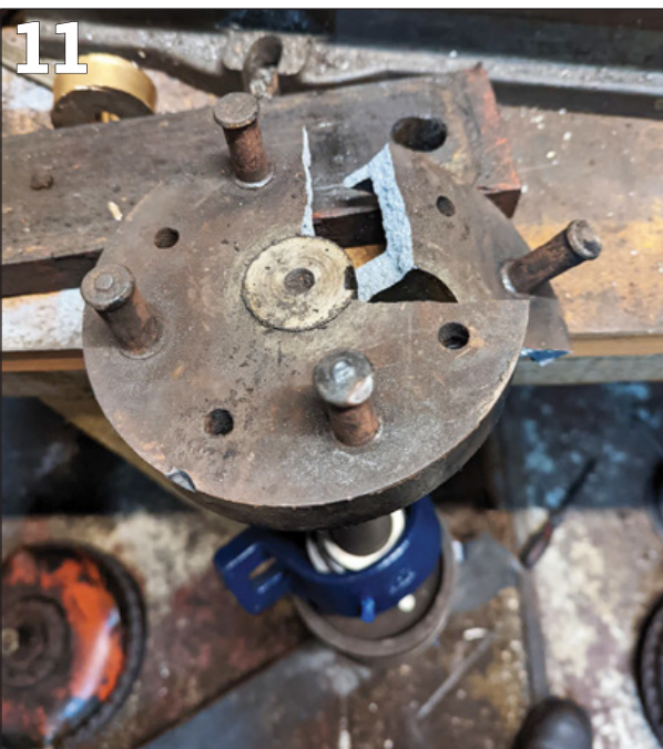
PHOTO 9: Using a slotting head attachment on the milling machine to cut the keyways in the new carriers.
