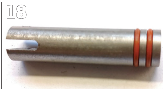
PHOTO 17: Mk1 piston with two O-rings.
