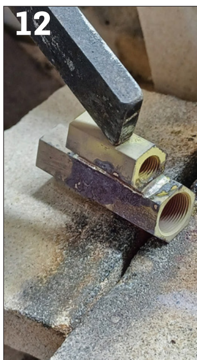
PHOTO 11: Pricking the pump body.
