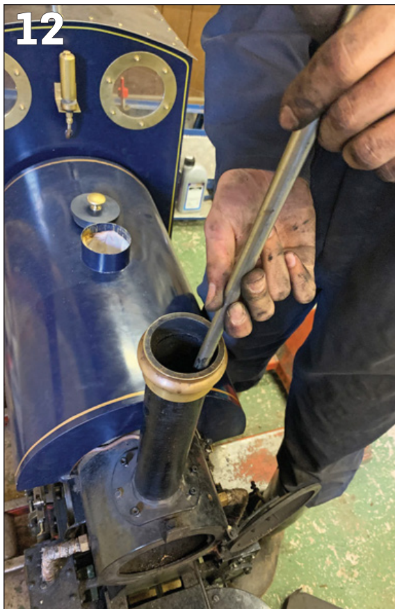
FIGURE 6: Blastpipe shroud style of spark arrester, for 7¼-inch gauge Sweet William or Romulus-sized locomotive.
