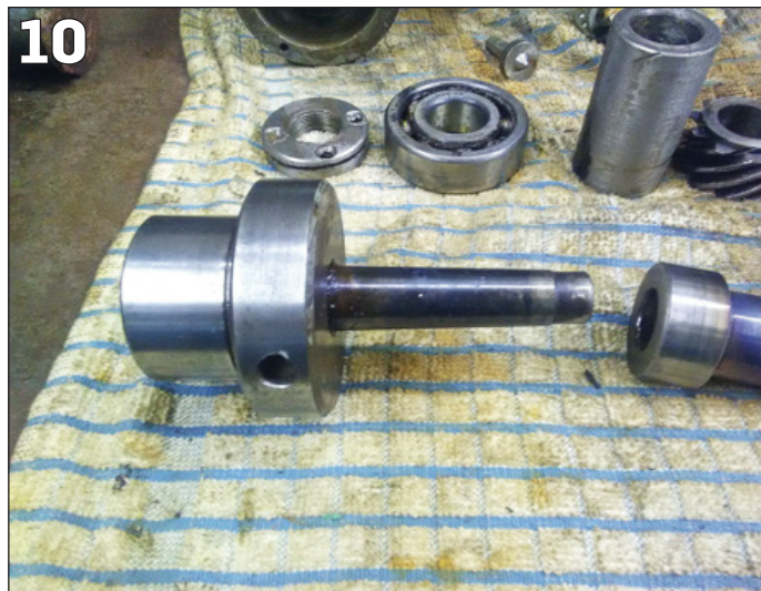
PHOTO 9: The component parts of the vertical head after dismantling.
