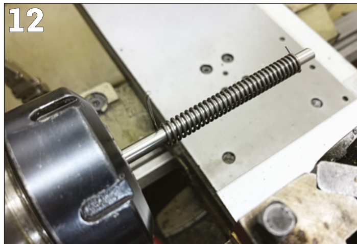
PHOTO 10: Spring-making underway, using automatic lathe feed (screw-cutting) settings.
