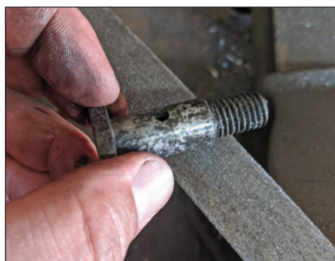
23: Pin checked with file to ensure it is hard enough – file skates over the surface, proving pin is harder than file.
