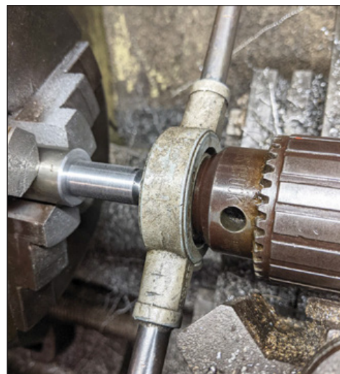
4: Face of chuck rests against die to ensure thread is cut parallel.
