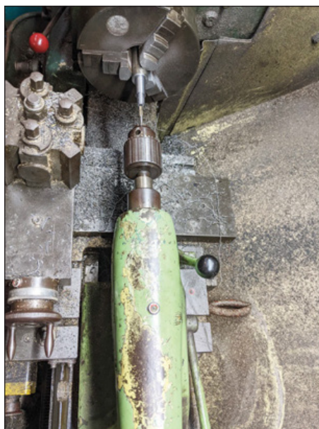
6: Power tapping at very slow speed, tap held in tailstock chuck which is not clamped to bed and can be drawn towards chuck as thread is cut.
