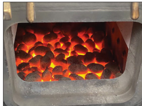
ABOVE: Bio-coal producing what was described as an even fire bed in the Bure Valley Railway's locomotive 'Blickling Hall', on which the trials were conducted. Photo: BVR
