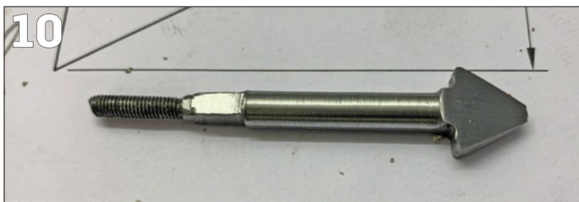
PHOTO 9: Experimenting with part which had not been pre-rounded by filing.
