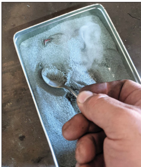
19: Hot pin covered over and left for couple of minutes.
