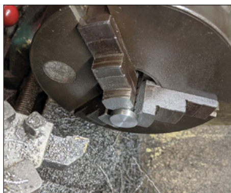
12: Final lathe operation – pin head faced down to final thickness.
