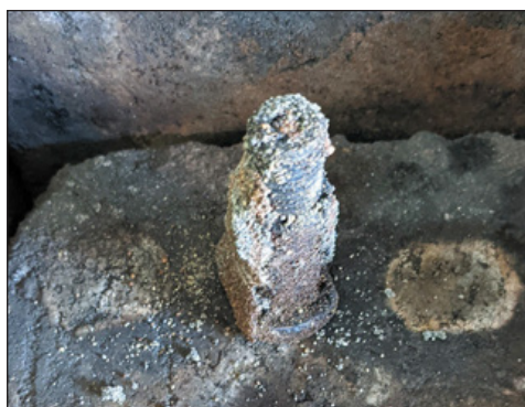
21: Pin then re-heated until powder turns molten and black – this is also annealing temperature.
