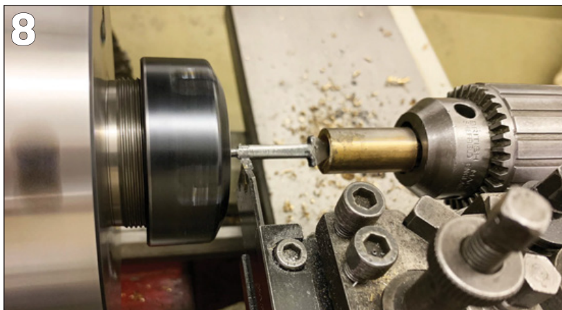
PHOTO 6: Side view of dead-centre – turned-down section allowed it to be gripped in standard (13mm) Jacobs chuck.
