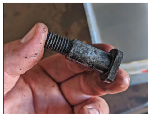
22: After quenching pins look like this – process can be repeated to increase hardening thickness.
