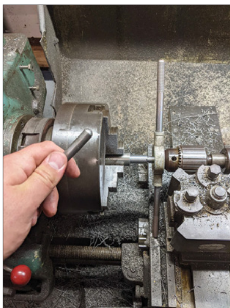
5: With lathe out of gear, chuck key used to turn workpiece while gentle pressure applied using tailstock.
