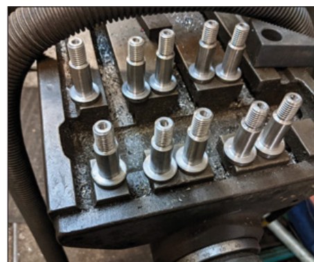
13: The 10 finished motion pins ready for milling of their heads.
