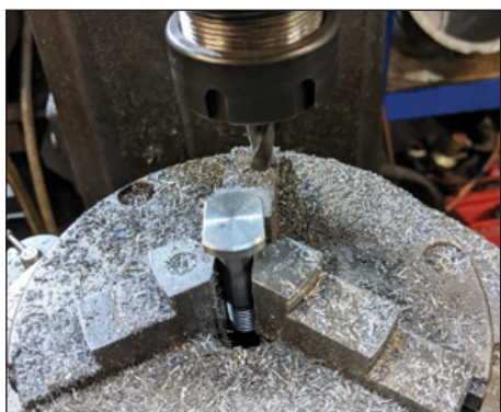
14: Milling flats on heads using rotary table to spin pins 180 degrees at a time.
