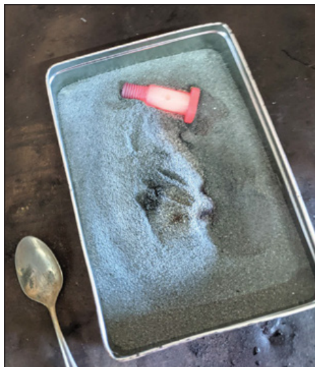
18: Once at correct temperature pins put into hardening powder.
