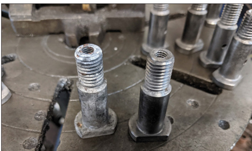
24: Quench tubular items with cross holes in carefully – this staged photo shows water can flash-boil in hole and shoot out at great speed.
