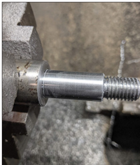
9: Final finish following use of emery – pin turned 2 thou under-size to allow for thickness of surface hardening.
