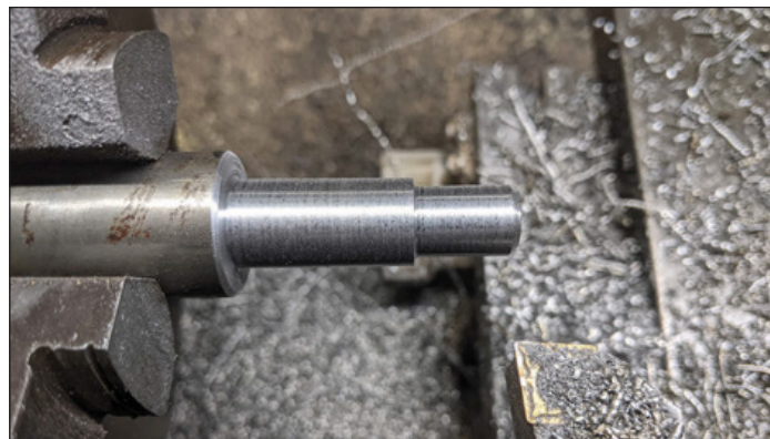
2: Turning the thread outer diameter – a little manual CNC to put a chamfer on the end.
