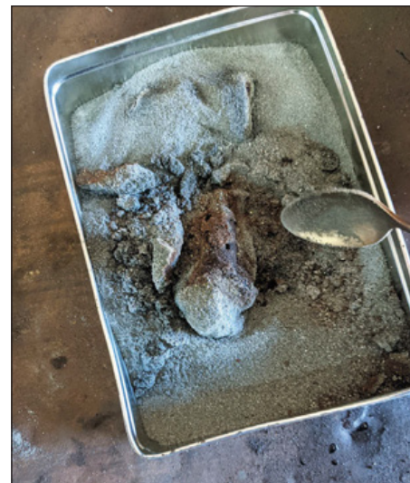
20: Pin will come out with layer of powder semi-melted onto it.
