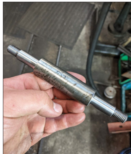
10: Pin blanks machined on each end of piece of bar before cutting off, this allows for less wastage and better part holding in lathe.
