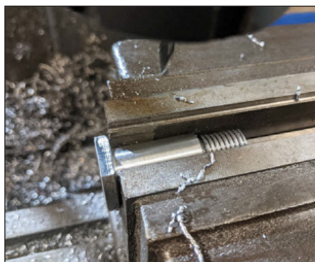
15: Using 4mm two-flute end mill to put grease-way into side of pin.
