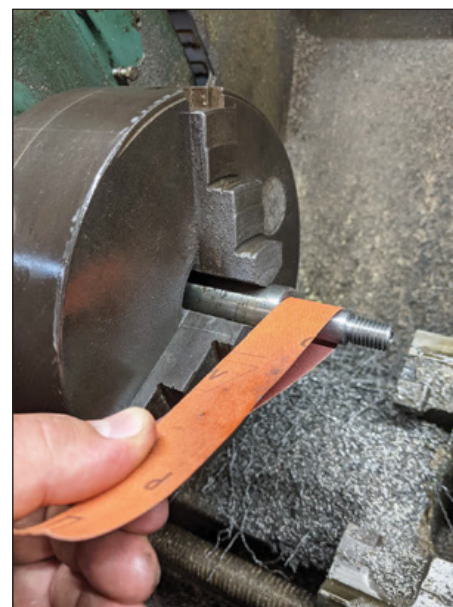
4: Face of chuck rests against die to ensure thread is cut parallel.
