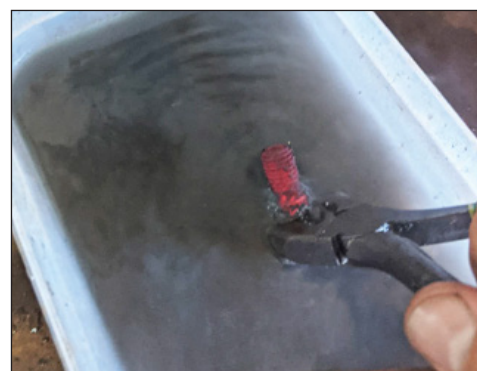
24: Quench tubular items with cross holes in carefully – this staged photo shows water can flash-boil in hole and shoot out at great speed.
