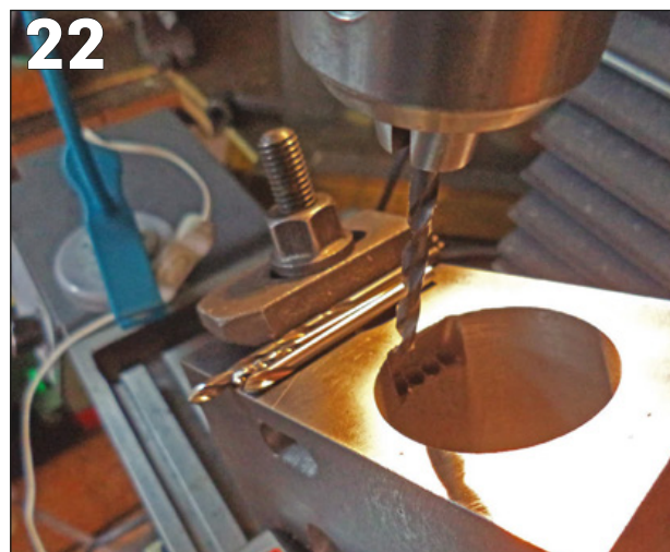
PHOTO 23: PCD feature on DRO used for drilling and tapping holes for covers.
