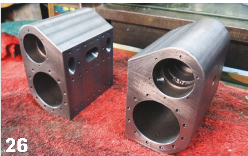
PHOTO 24: Cylinder fixing holes drilled and tapped.
