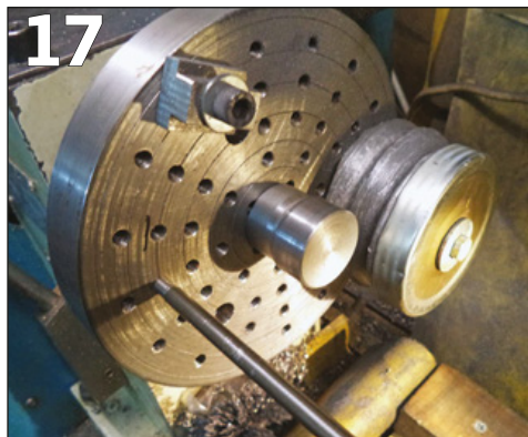
PHOTO 17: Face plate with mandrel clamp stud and counterbalance weight attached.
