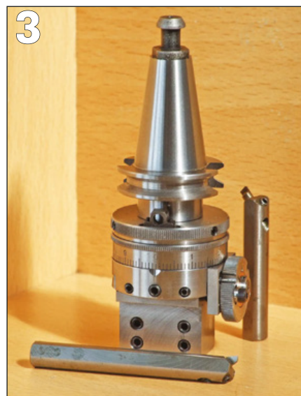
PHOTO 2: The 50mm boring and facing head with a torque arm.
