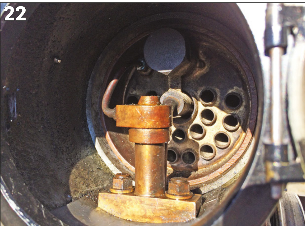
PHOTO 22: Blastpipe arrangement assembled in smokebox.
