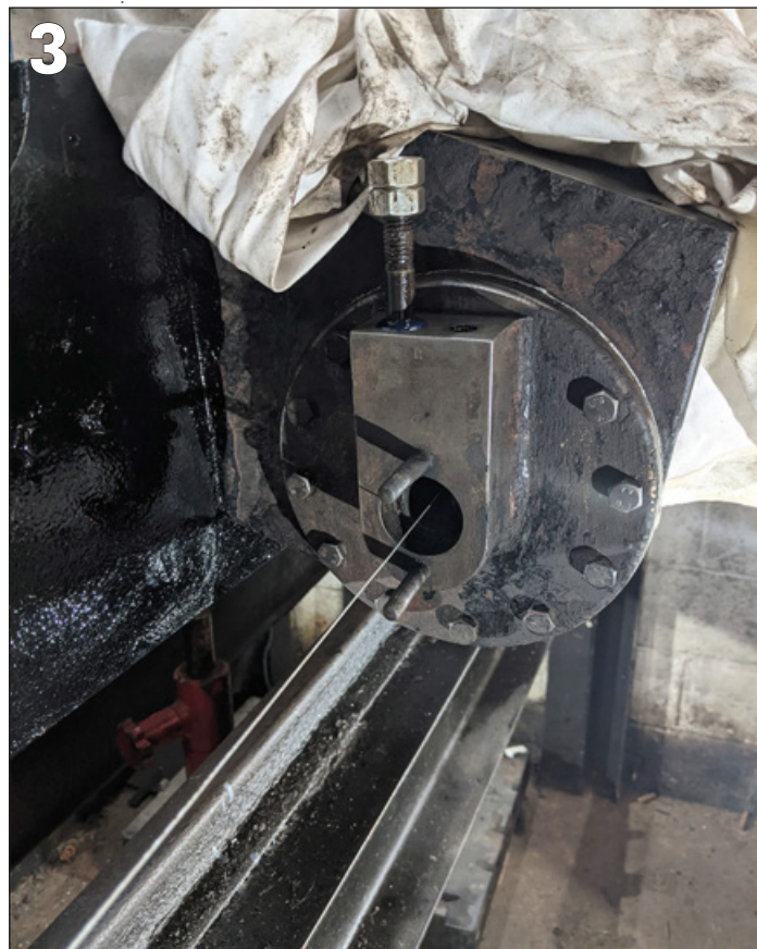
PHOTO 3: Cylinder lining showing taut wire passing through rear cylinder cover, extreme care needed to ensure this is absolutely true to bore.
