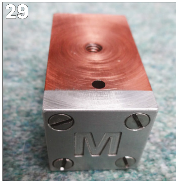
PHOTO 28: Milling machine CNC engraving the M on top of cylinder cover.
