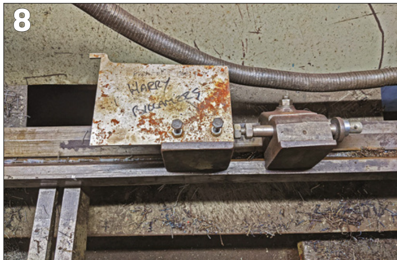
PHOTO 7: Copier head dropped onto the dovetails on the back of the cross-slide.
