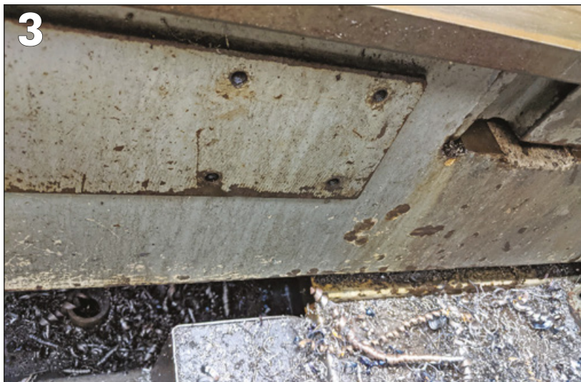
PHOTO 3: Bolting pads for the copier on the back of the lathe bed.
