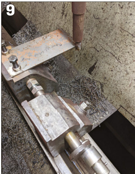
PHOTO 9: Further view of pattern-holding block and adjuster block, note dial adjuster to move pattern longitudinally.
