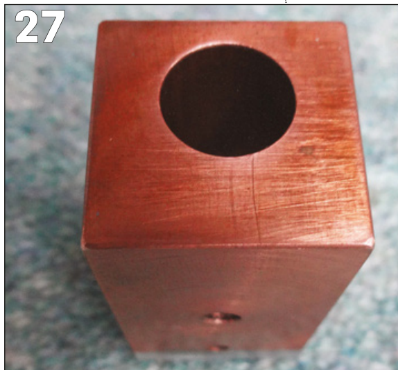
PHOTO 27: Cylinder base, showing the cylinder bore – this reamed beautifully, ending up silky-smooth.
