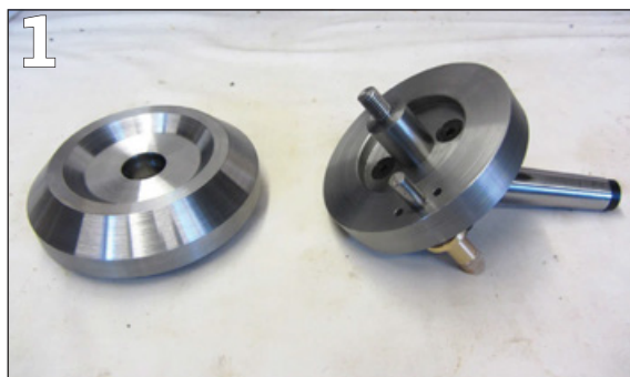
PHOTO 1: Tailstock turret and its backplate.
