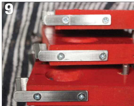
PHOTO 11: Tubular spacers turned to suit crank pins.
