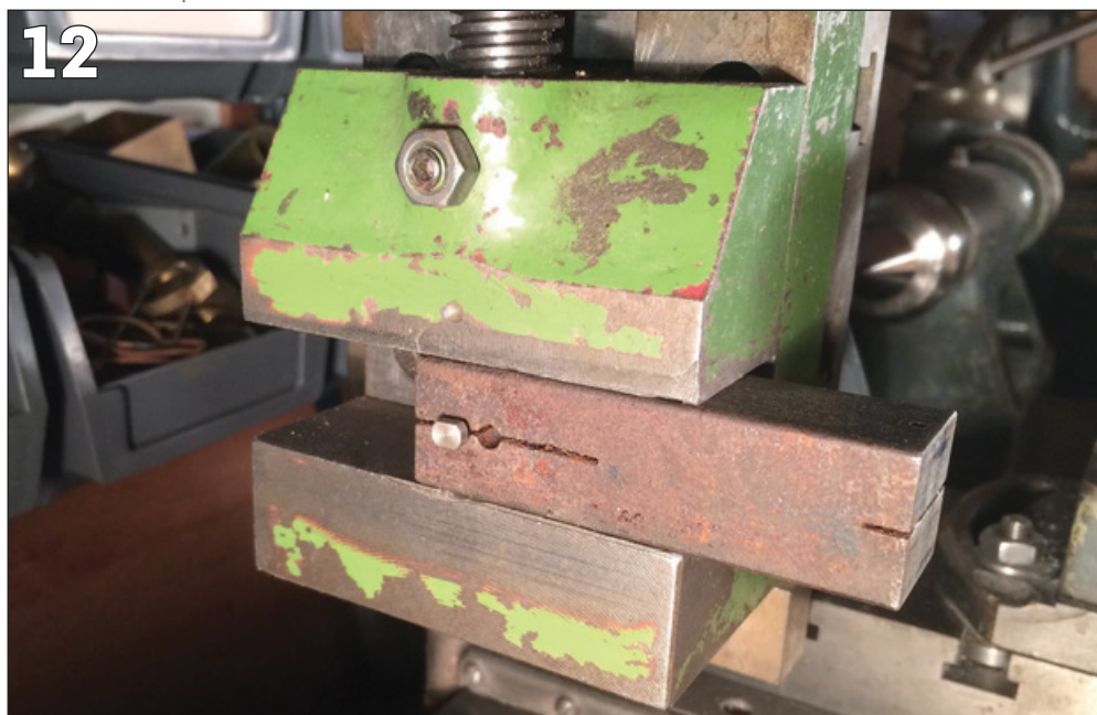
PHOTO 12: Final step on pins, machining flats on heads to accept a spanner.
