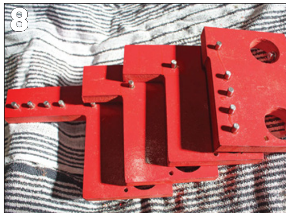
PHOTO 8: Axle and crank holding points fitted.
