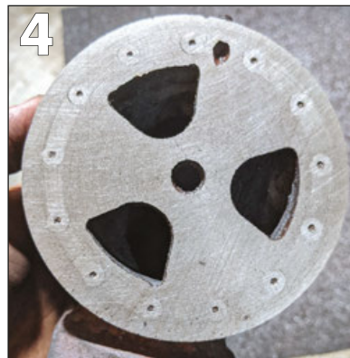
PHOTO 1: Start – bronze moving section of regulator as taken off boiler.
