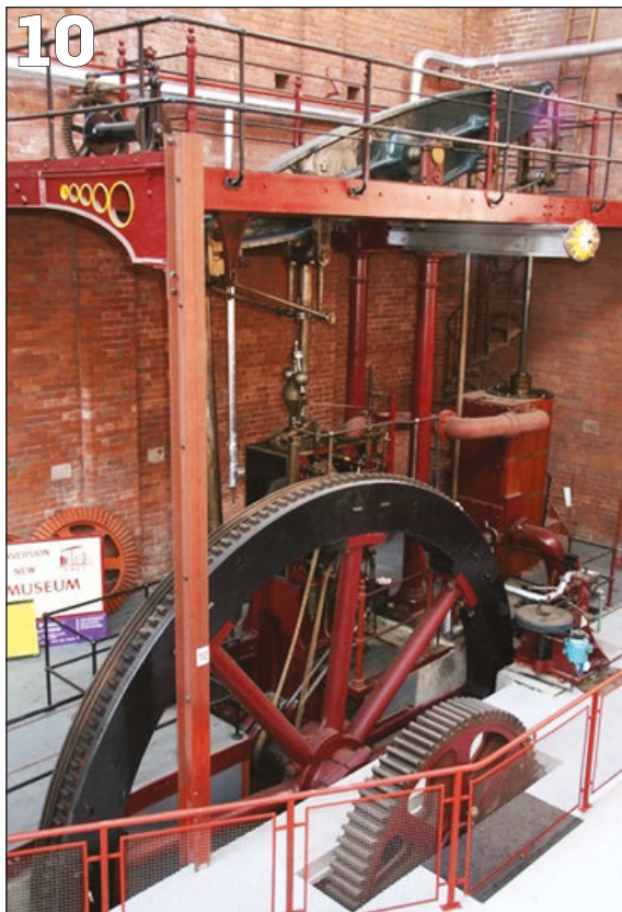
PHOTO 10: To increase the power output of an early beam engine, William McNaught introduced a second high pressure cylinder fitted at the crankshaft end. This modification was made to the Cellarsclough Mill engine, and the forerunner of true compounding. This McNaught beam engine is preserved in the extensive collection at the Bolton Steam Museum.
