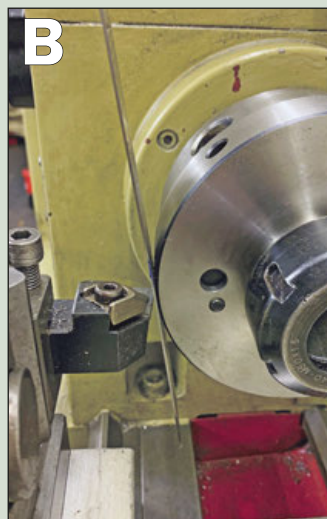
B: Setting tool height on Harrison M300 – here tool is too low.
