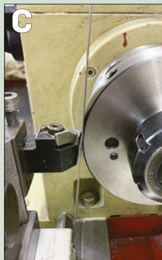
C: Here tool is sloping towards chuck at top, showing it's too high.
