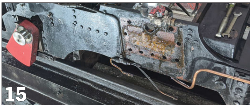
PHOTO 13: Sherpa's left-hand cylinder after removal.
