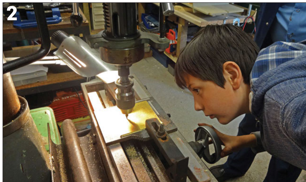
PHOTO 2: Setting up the manual mill ready for drilling with a Slocomb centre-drill bit.
