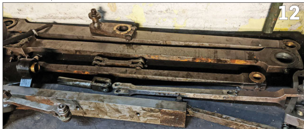
PHOTO 12: Motion of loco 'Sherpa' has been carefully stacked on shelving for later refitting.
