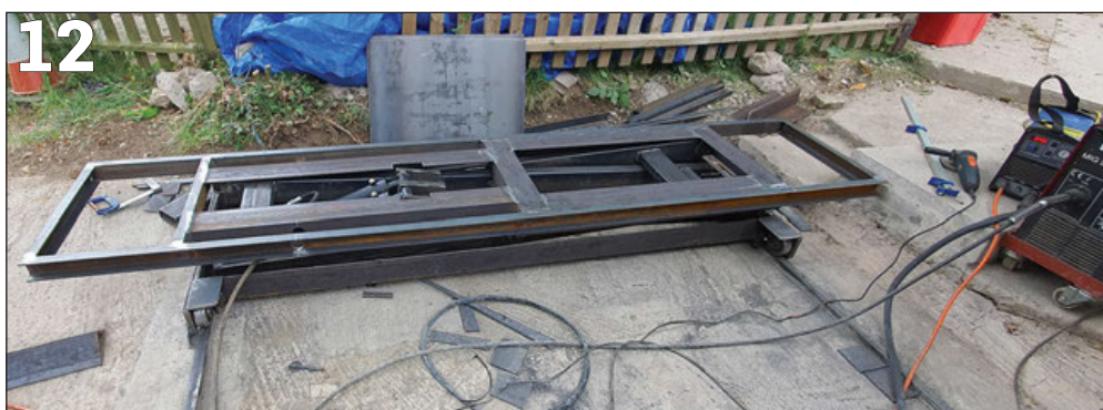
PHOTO 8: Pivot bushes for the outer scissor legs being welded into place.
