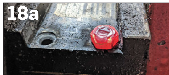
PHOTO 18A-C: Nuts had to be welded onto axlebox keep bolts to remove them. Top view shows second attempt after first weld failed.
