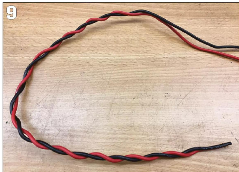
PHOTO 9: The resulting twisted-pair cable, this one relatively loosely twisted.
