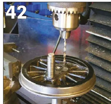
PHOTO 39: Left-hand wheel pinned to axle.
