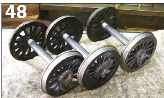
PHOTO 46: Centre-punch holes show where axles were boded to fit.
