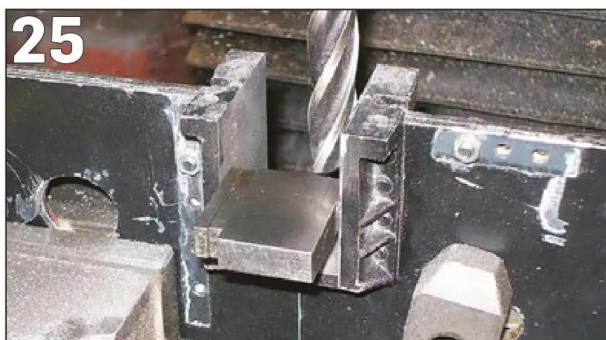
PHOTO 30: Jig for milling hornblocks to width.
