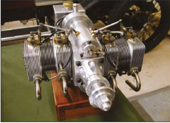
ABOVE AND BELOW: Front and rear views of the twin-cylinder Demont double-acting engine.
