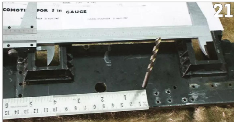
PHOTO 21: Frame marked out for centre of axlebox.
